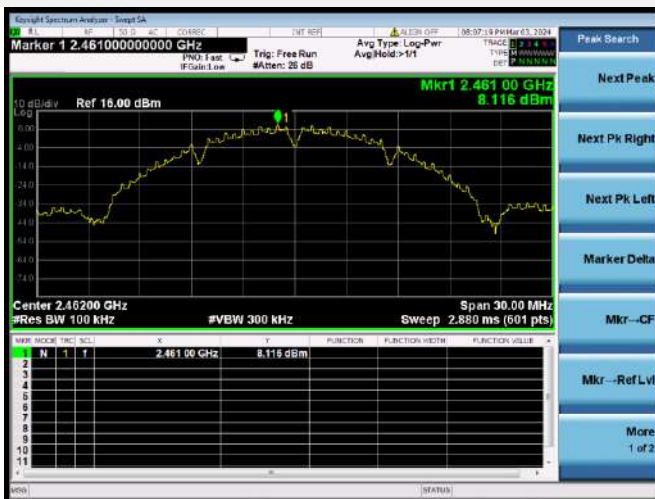
802.11b CHANNEL 11, CARRIER LEVEL
