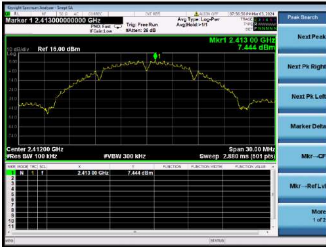
802.11b CHANNEL 1, CARRIER LEVEL
