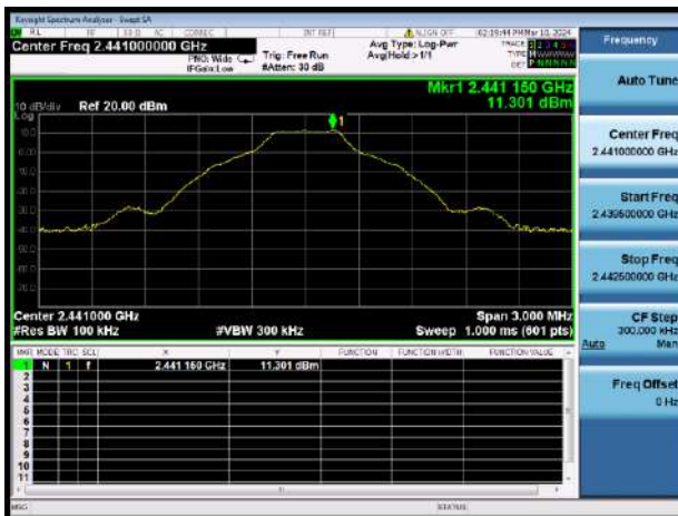
GFSK MIDDLE CHANNEL, CARRIER LEVEL
