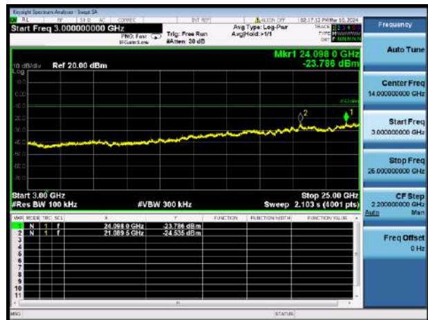
GFSK LOW CHANNEL, SPURIOUS 3 GHz ~ 25 GHz
