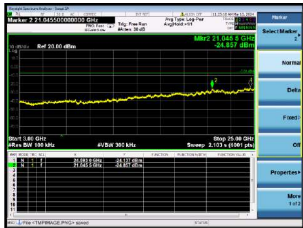
GFSK MIDDLE CHANNEL, SPURIOUS 3 GHz ~ 25 GHz
