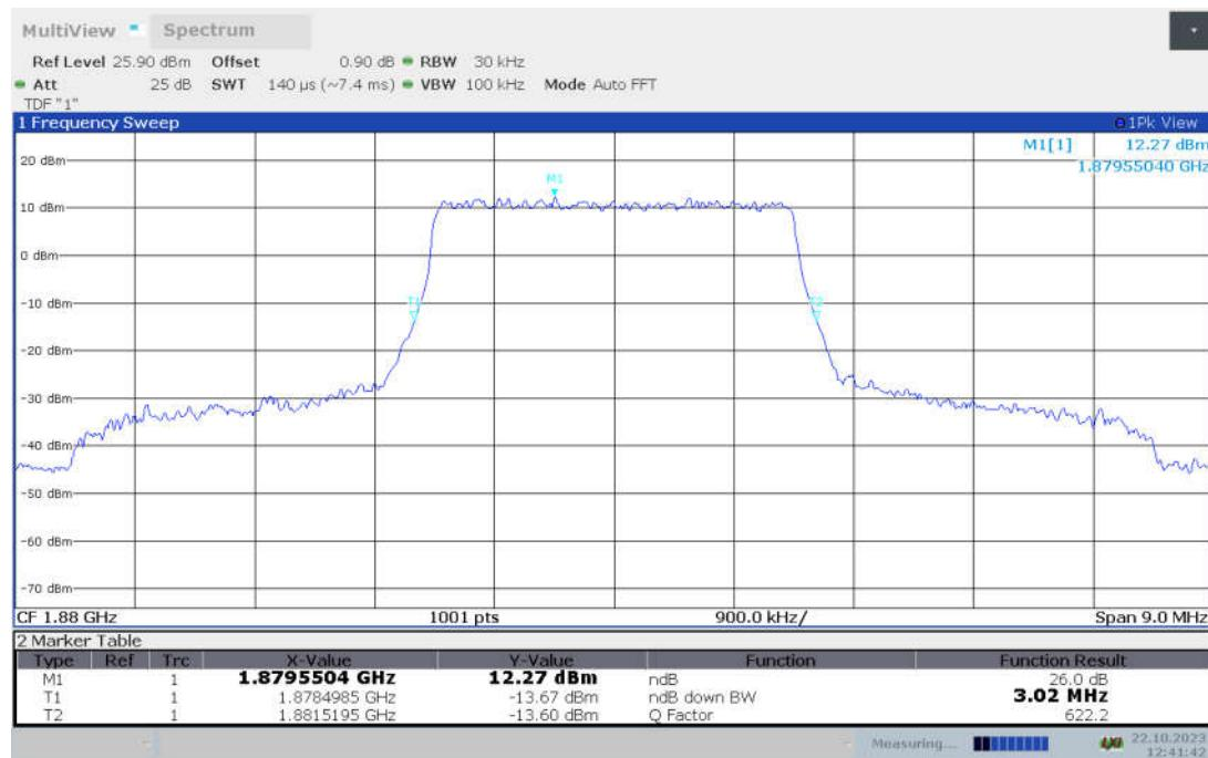
**LTE band 2 , 3MHz Bandwidth, MID, 16QAM (-26dBc BW)**
