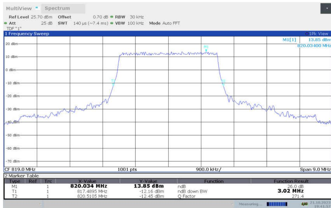
**LTE band 26 , 3MHz Bandwidth, MID, 16QAM (-26dBc BW)**
