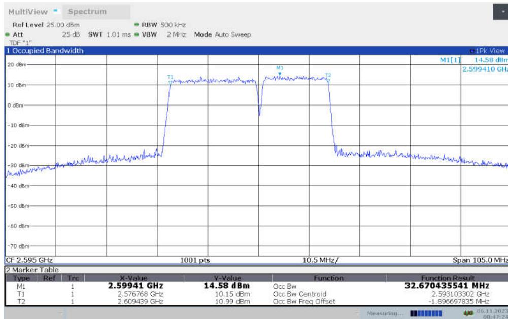
**LTE CA\_41C , 20MHz+15MHz Bandwidth, 16QAM (99% BW)**
