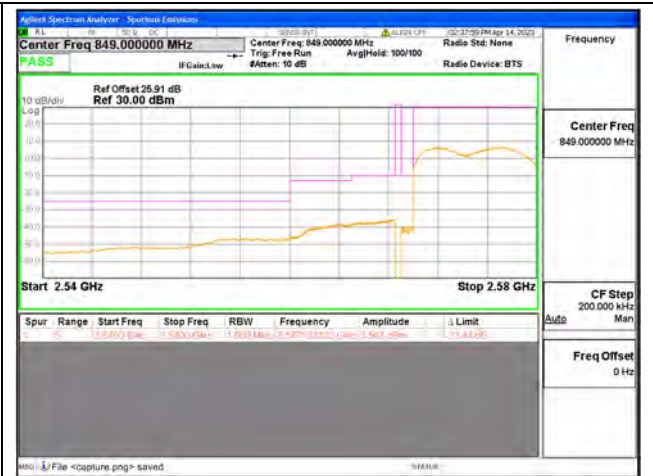
Band38 / 10MHz / Low CH / QPSK / FULL RB
