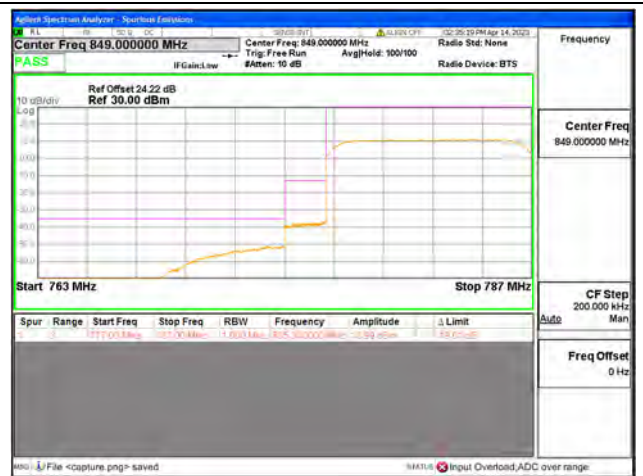
Band13 / 10MHz / Low CH / QPSK / FULL RB
