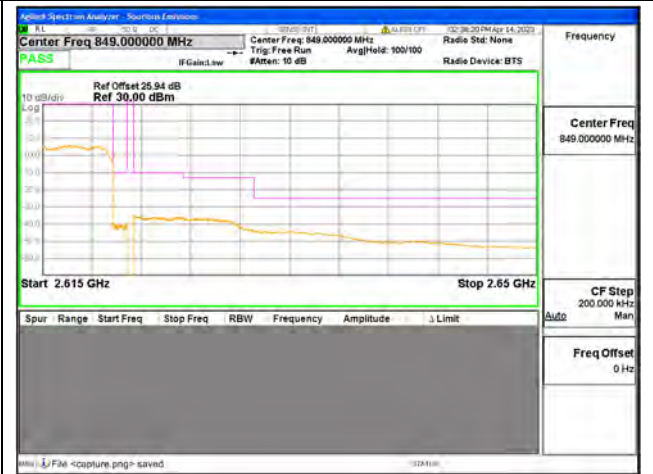
Band38 / 10MHz / High CH / QPSK / FULL RB
