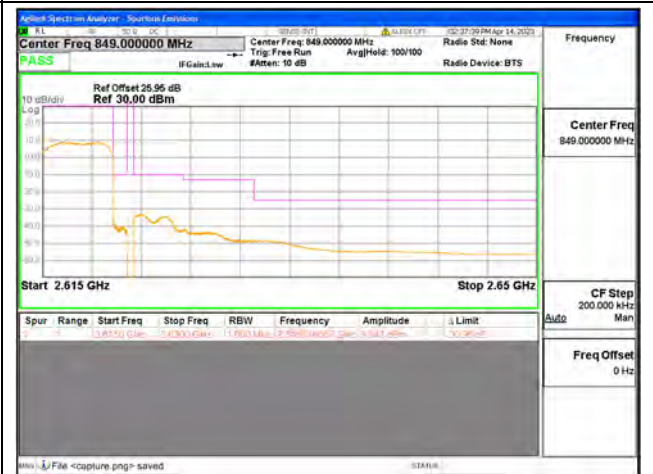
Band38 / 5MHz / High CH / QPSK / FULL RB
