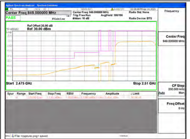
Band7 / 10MHz / Low CH / QPSK / FULL RB
