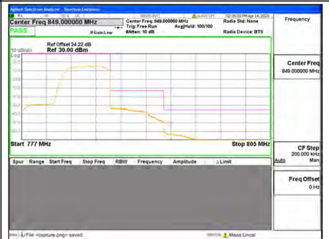
Band13 / 5MHz / High CH / QPSK / FULL RB
