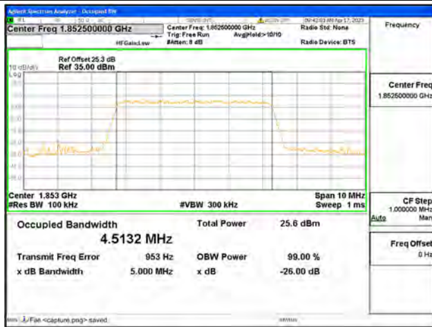
Band2 / 5MHz / 64QAM/ Low CH
