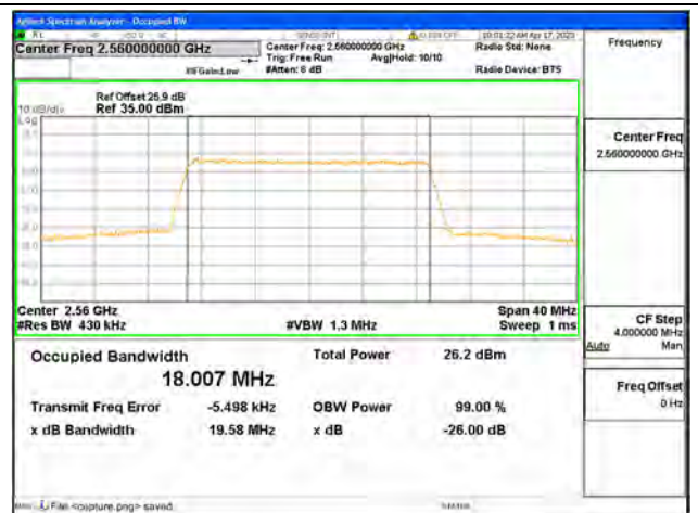
Band7 / 20MHz / 64QAM/ High CH
