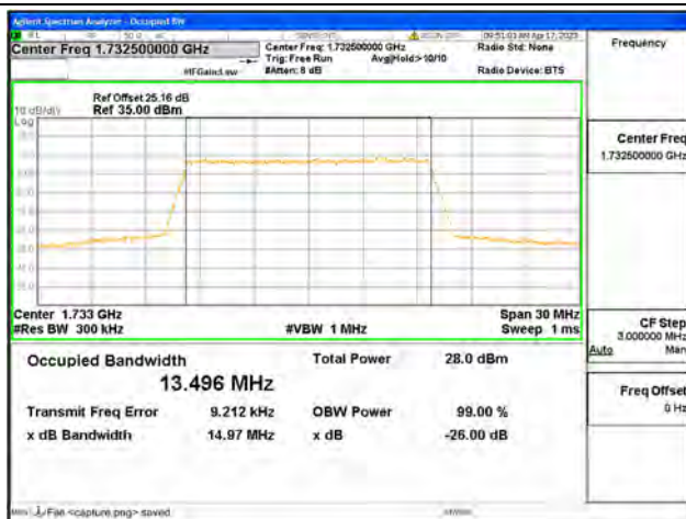
Band4 / 15MHz / 16QAM/ Mid CH
