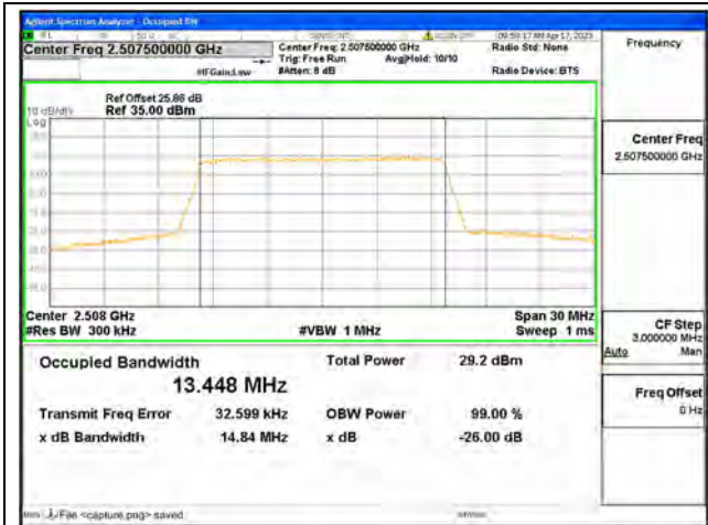
Band7 / 15MHz / QPSK/ Low CH
