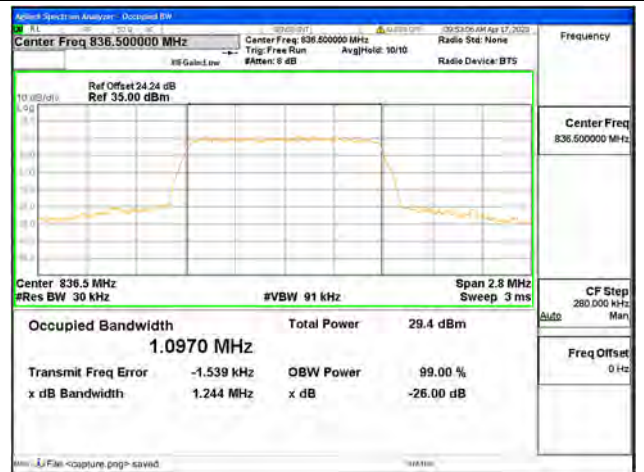
Band5 / 1.4MHz / QPSK/ Mid CH
