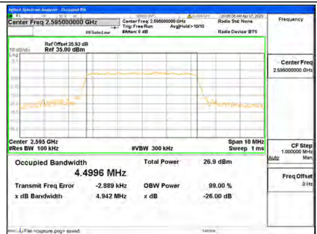
Band38 / 5MHz / 64QAM/ Mid CH
