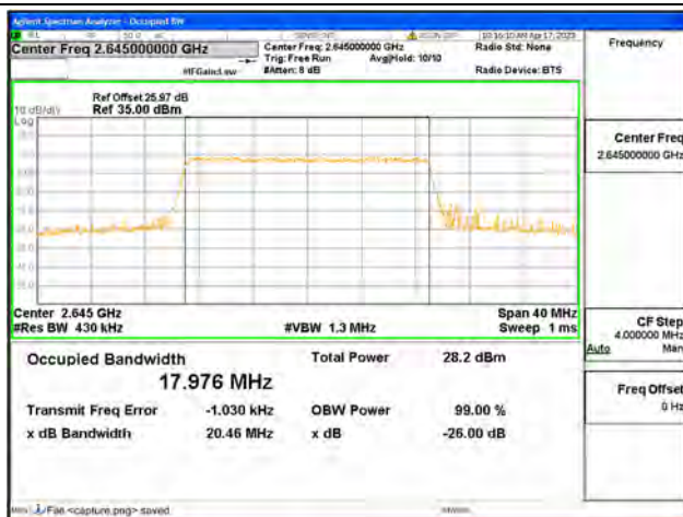
Band41(2535-2655) / 20MHz / 16QAM/ High CH
