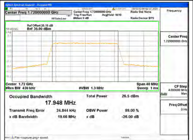
Band4 / 20MHz / 64QAM/ Low CH
