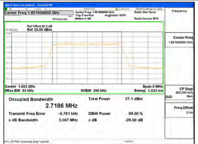
Band2 / 3MHz / QPSK/ Low CH
