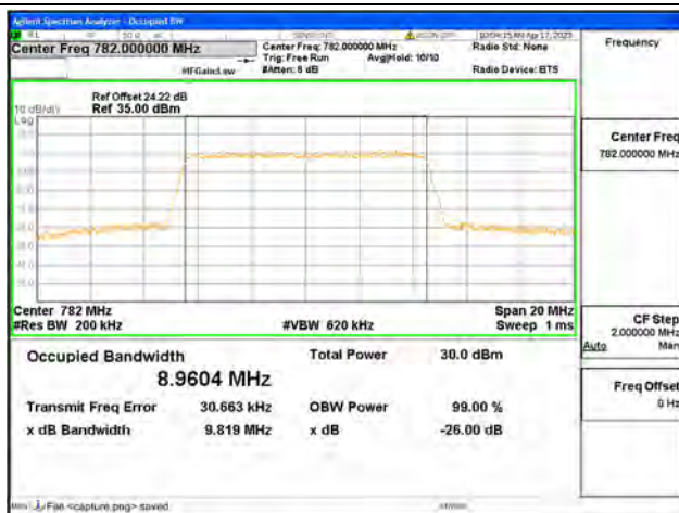
Band13 / 10MHz / 16QAM/ Mid CH
