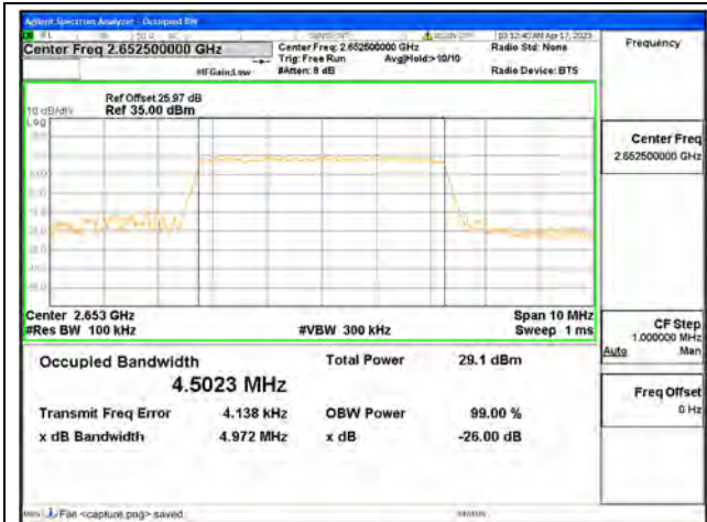
Band41(2535-2655) / 5MHz / QPSK/ High CH
