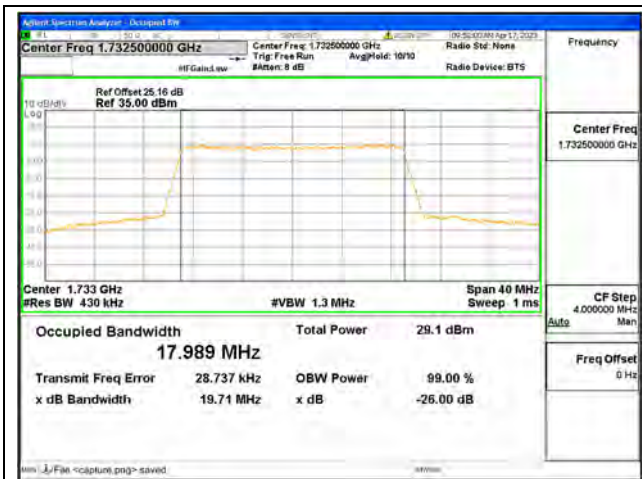
Band4 / 20MHz / QPSK/ Mid CH
