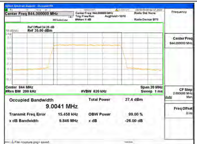
Band5 / 10MHz / 64QAM/ High CH
