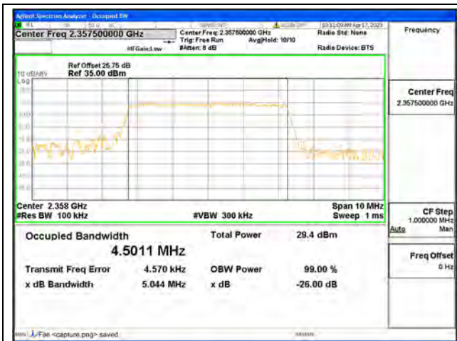
Band40-2 / 5MHz / QPSK/ High CH
