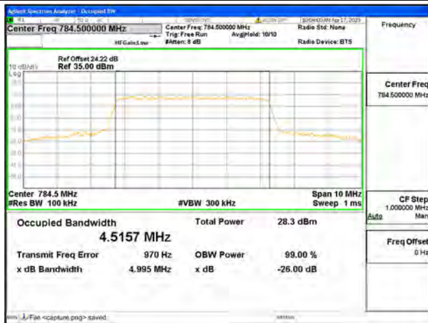
Band13 / 5MHz / 64QAM/ High CH
