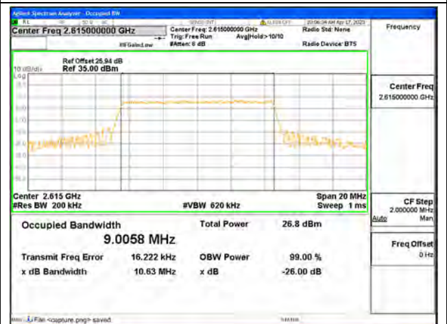
Band38 / 10MHz / 64QAM/ High CH
