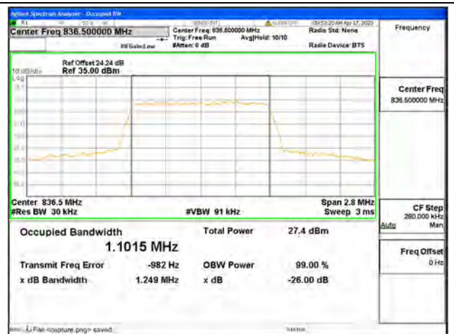
Band5 / 1.4MHz / 64QAM/ Mid CH
