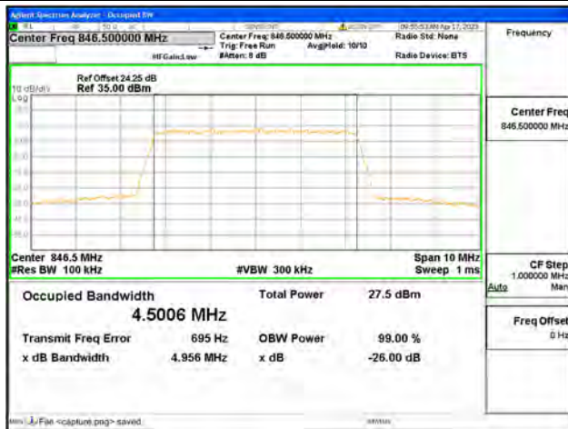
Band5 / 5MHz / 64QAM/ High CH
