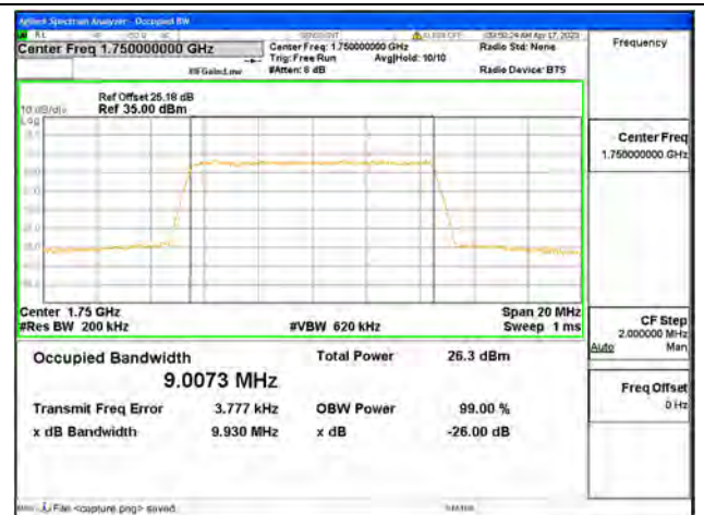
Band4 / 10MHz / 64QAM/ High CH
