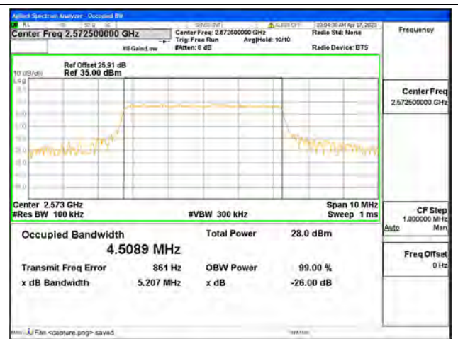
Band38 / 5MHz / 16QAM/ Low CH
