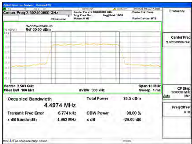
Band7 / 5MHz / 64QAM/ Low CH
