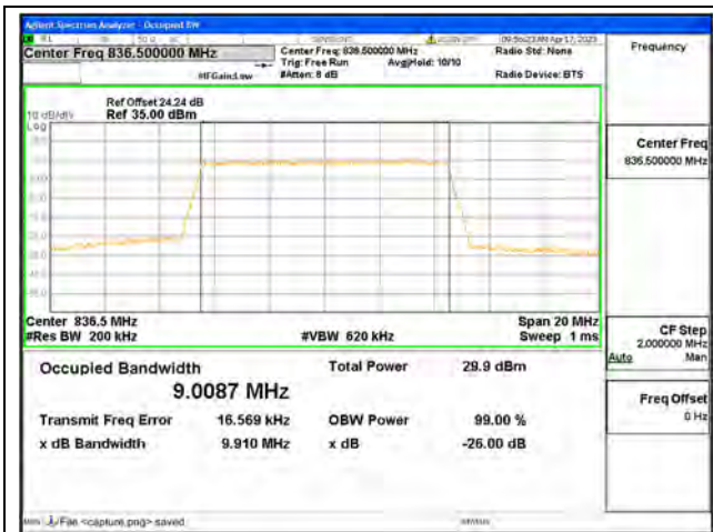
Band5 / 10MHz / QPSK/ Mid CH
