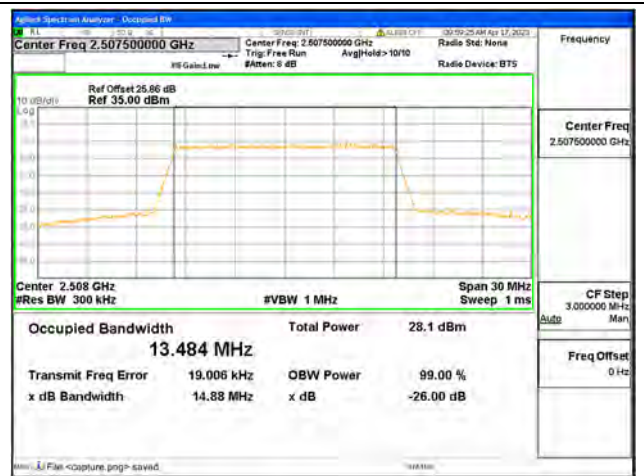
Band7 / 15MHz / 16QAM/ Low CH
