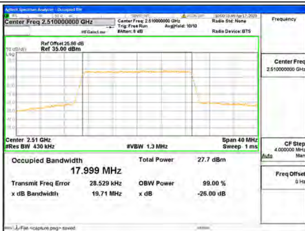
Band7 / 20MHz / 16QAM/ Low CH
