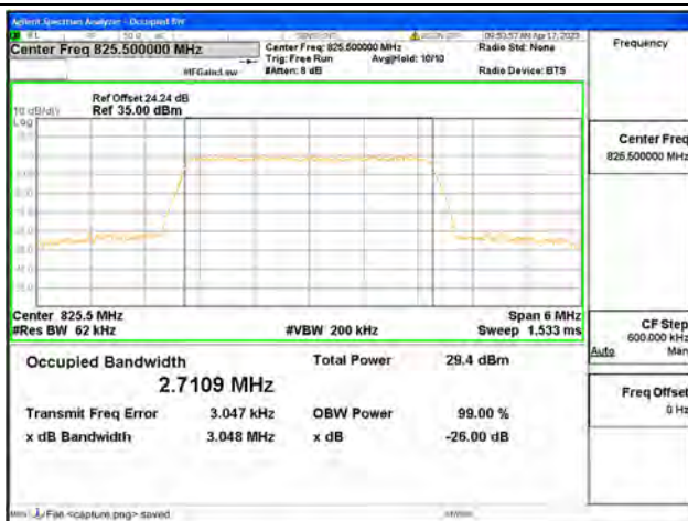
Band5 / 3MHz / 16QAM/ Low CH
