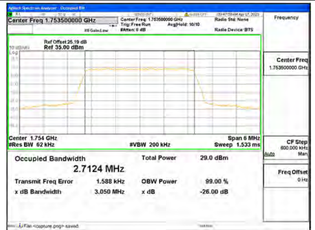
Band4 / 3MHz / QPSK/ High CH
