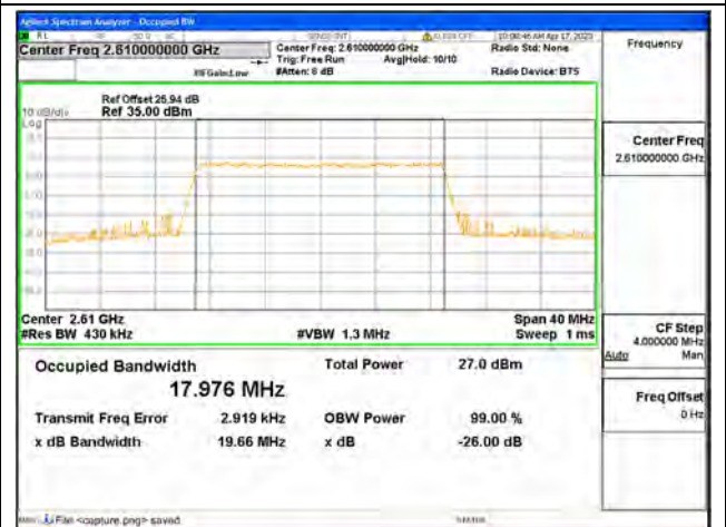
Band38 / 20MHz / 64QAM/ High CH
