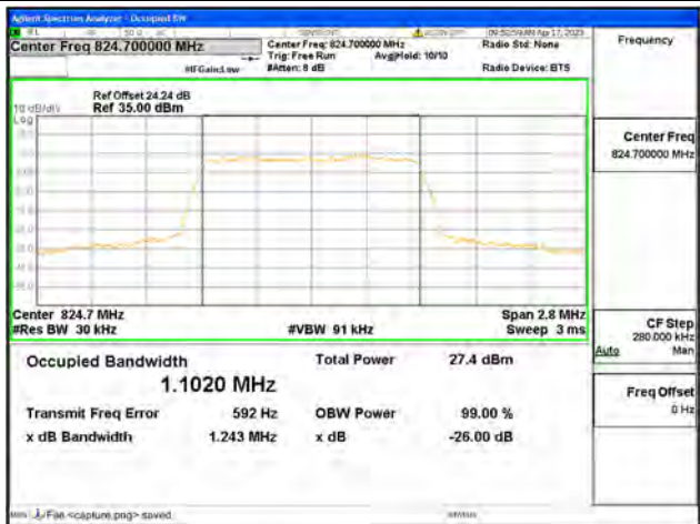
Band5 / 1.4MHz / 64QAM/ Low CH
