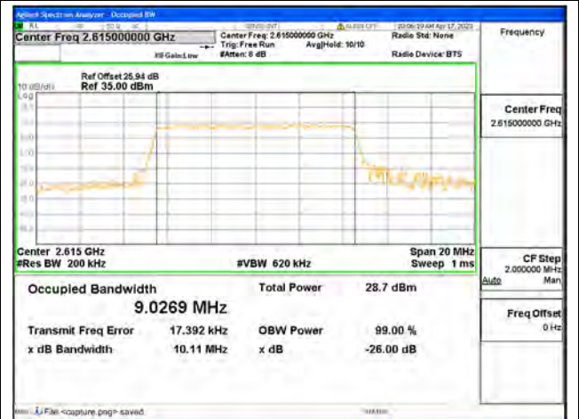
Band38 / 10MHz / QPSK/ High CH
