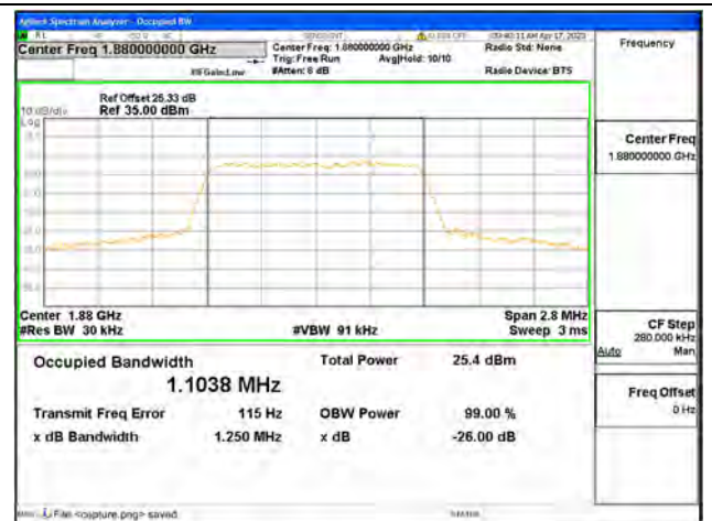
Band2 / 1.4MHz / 64QAM/ Mid CH
