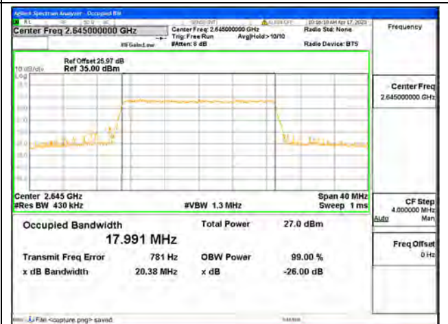
Band41(2535-2655) / 20MHz / 64QAM/ High CH
