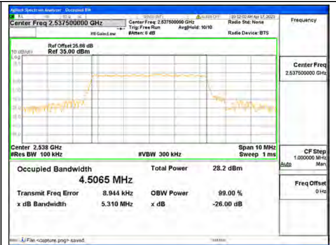
Band41(2535-2655) / 5MHz / 16QAM/ Low CH
