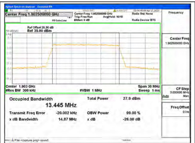
Band2 / 15MHz / 16QAM/ High CH
