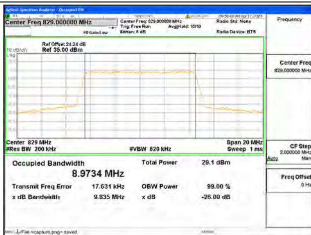
Band5 / 10MHz / 16QAM/ Low CH
