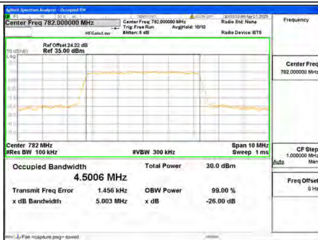
Band13 / 5MHz / 16QAM/ Mid CH
