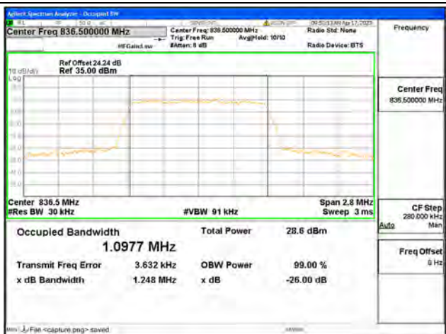
Band5 / 1.4MHz / 16QAM/ Mid CH
