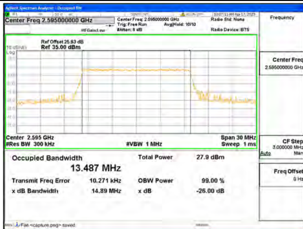
Band38 / 15MHz / 16QAM/ Mid CH
