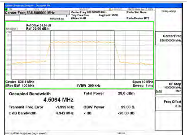
Band5 / 5MHz / 64QAM/ Mid CH
