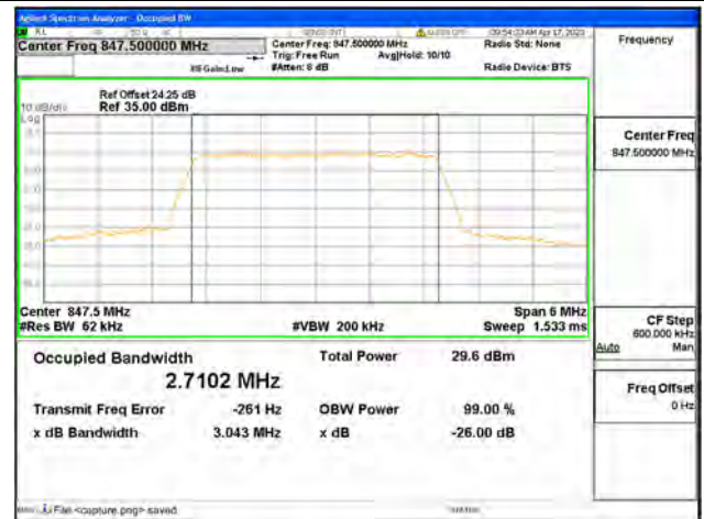
Band5 / 3MHz / QPSK/ High CH
