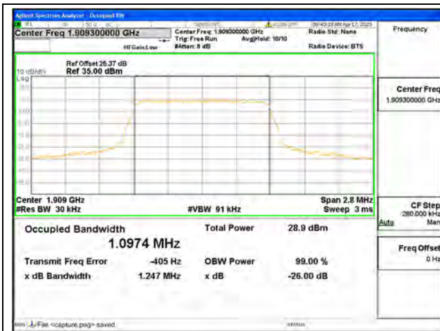
Band2 / 1.4MHz / QPSK/ High CH
