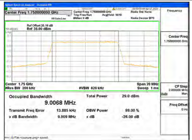
Band4 / 10MHz / QPSK/ High CH
