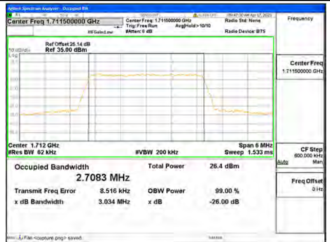
Band4 / 3MHz / 64QAM/ Low CH
