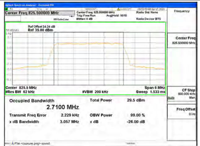
Band5 / 3MHz / QPSK/ Low CH
