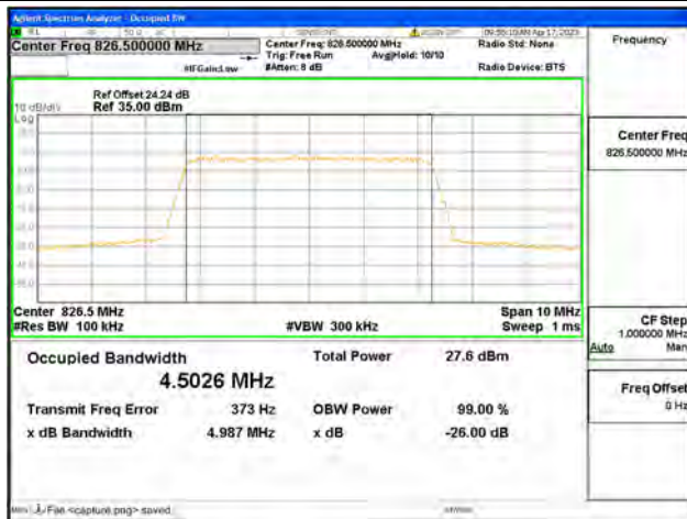
Band5 / 5MHz / 64QAM/ Low CH
