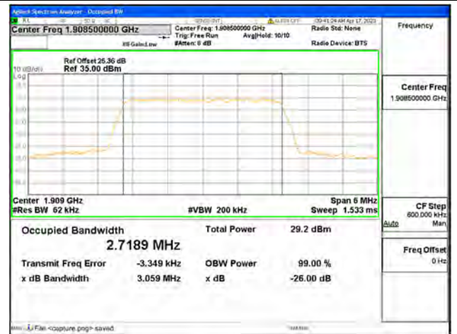
Band2 / 3MHz / QPSK/ High CH
