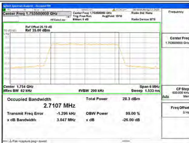
Band4 / 3MHz / 16QAM/ High CH
