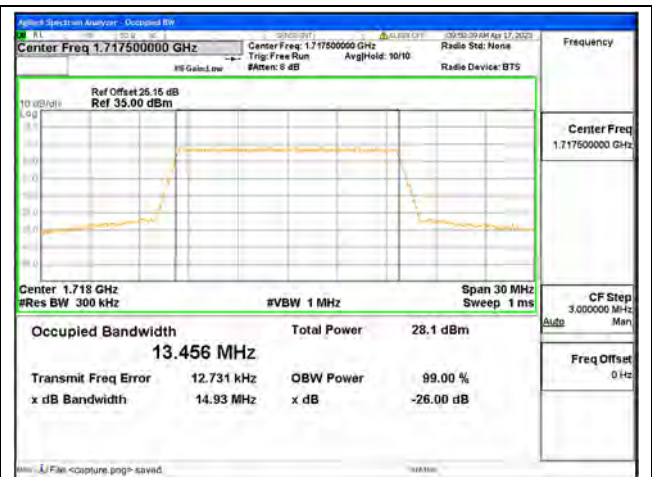
Band4 / 15MHz / 16QAM/ Low CH
