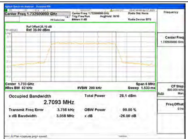
Band4 / 3MHz / 16QAM/ Mid CH
