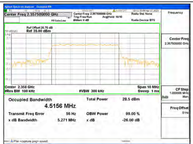
Band40-2 / 5MHz / 16QAM/ High CH
