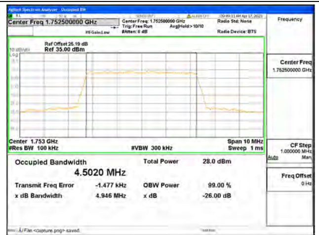
Band4 / 5MHz / 16QAM / High CH
