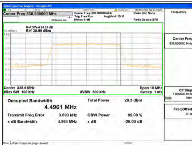
Band5 / 5MHz / 16QAM/ Mid CH
