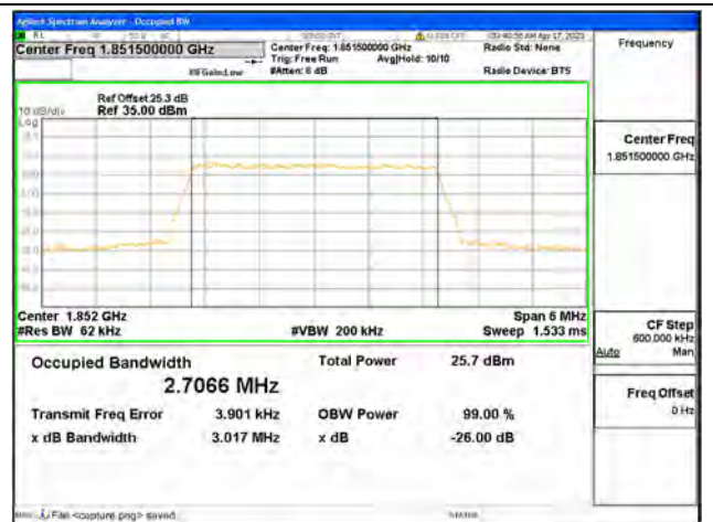
Band2 / 3MHz / 64QAM/ Low CH
