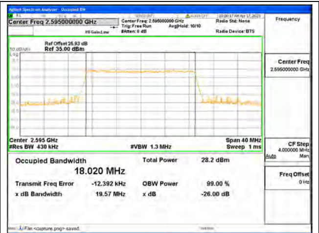
Band38 / 20MHz / 16QAM/ Mid CH
