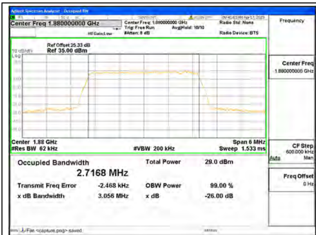
Band2 / 3MHz / QPSK/ Mid CH
