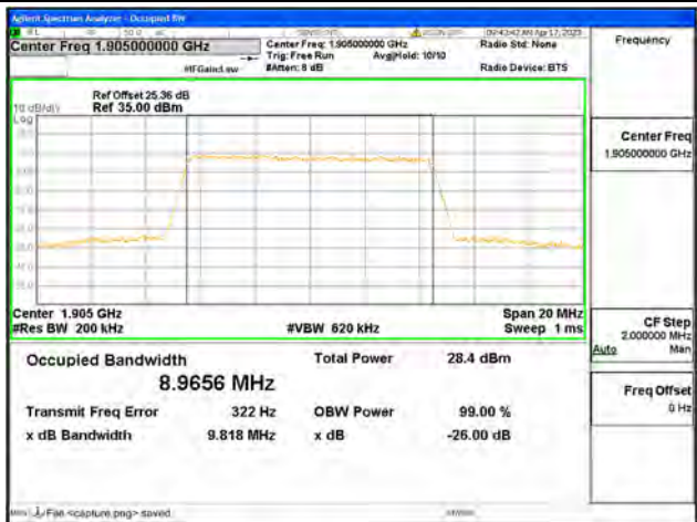
Band2 / 10MHz / 16QAM/ High CH
