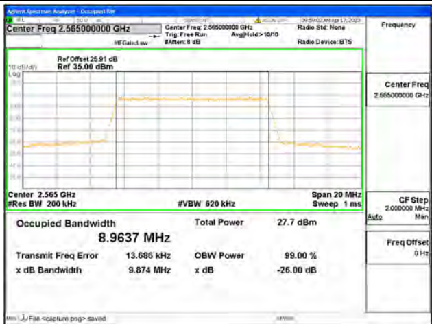
Band7 / 10MHz / 16QAM/ High CH
