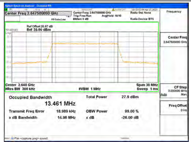
Band41(2535-2655) / 15MHz / 16QAM / High CH
