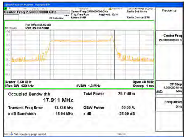
Band38 / 20MHz / QPSK/ Low CH
