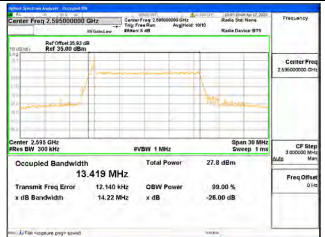
Band38 / 15MHz / 64QAM/ Mid CH
