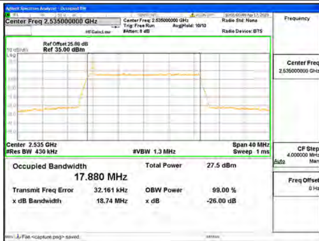
Band7 / 20MHz / 64QAM/ Mid CH
