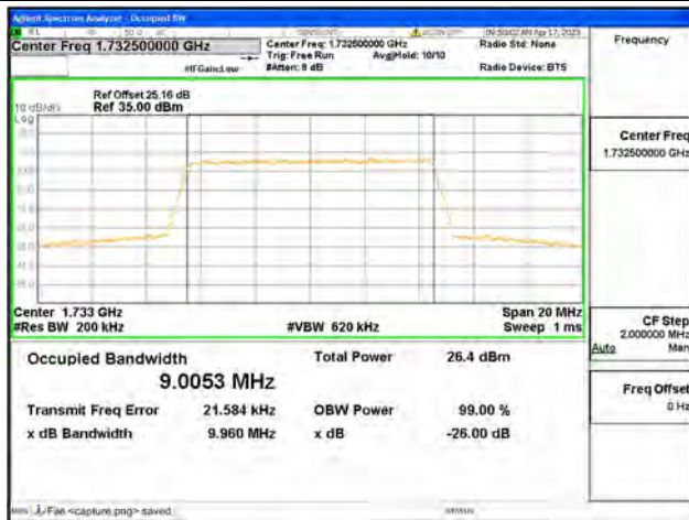
Band4 / 10MHz / 64QAM/ Mid CH
