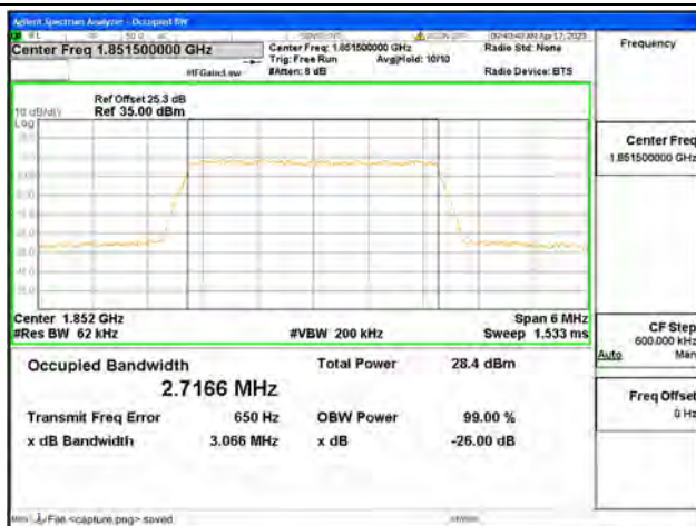
Band2 / 3MHz / 16QAM/ Low CH
