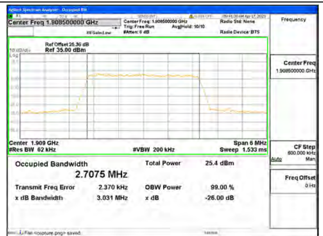
Band2 / 3MHz / 64QAM/ High CH
