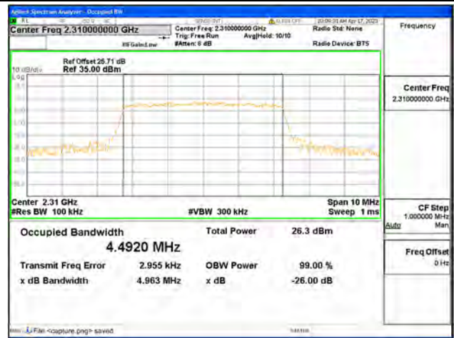
Band40-1 / 5MHz / 64QAM/ Mid CH
