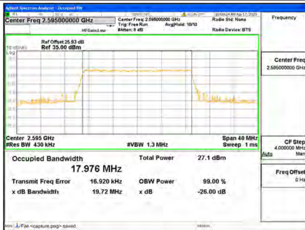
Band38 / 20MHz / 64QAM/ Mid CH
