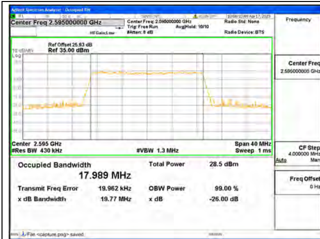
Band38 / 20MHz / QPSK/ Mid CH
