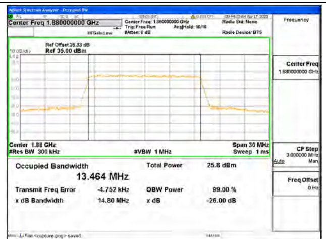
Band2 / 15MHz / 64QAM/ Mid CH
