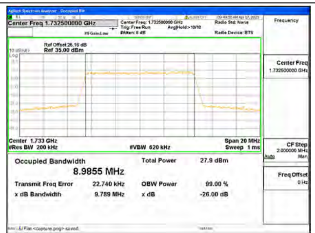
Band4 / 10MHz / 16QAM/ Mid CH
