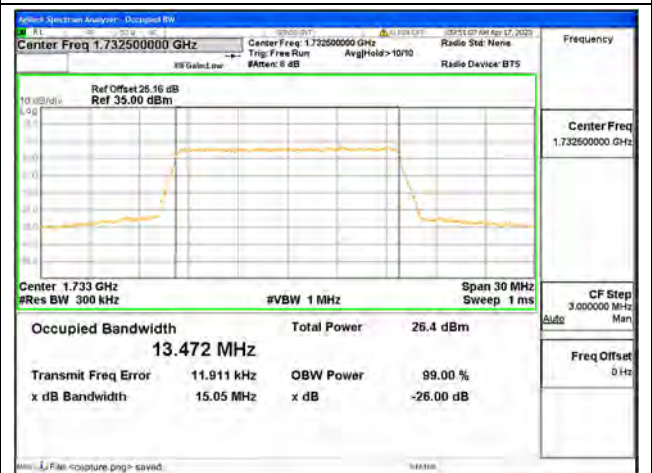
Band4 / 15MHz / 64QAM/ Mid CH
