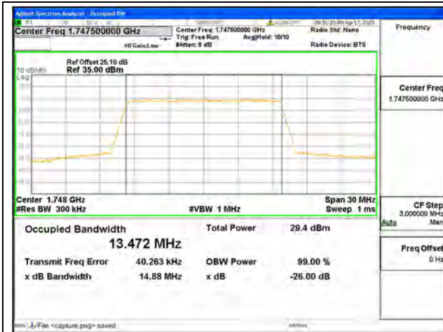
Band4 / 15MHz / QPSK/ High CH
