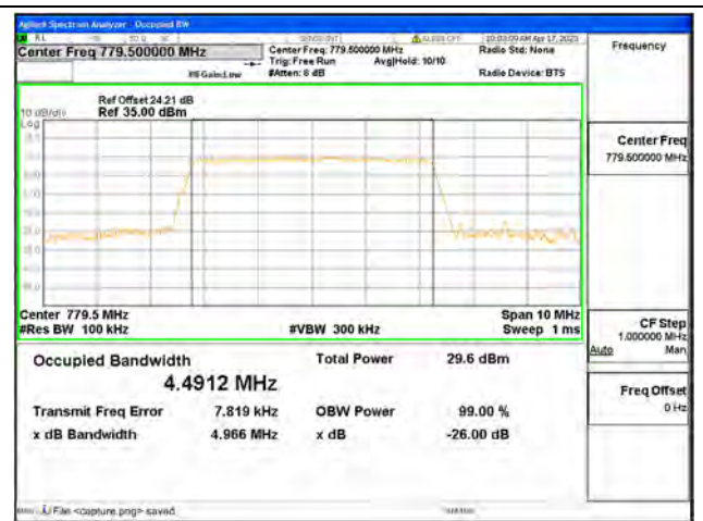
Band13 / 5MHz / 16QAM/ Low CH
