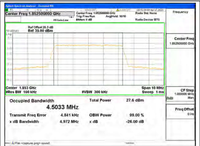
Band2 / 5MHz / 16QAM/ Low CH
