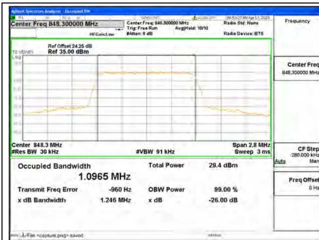
Band5 / 1.4MHz / QPSK/ High CH
