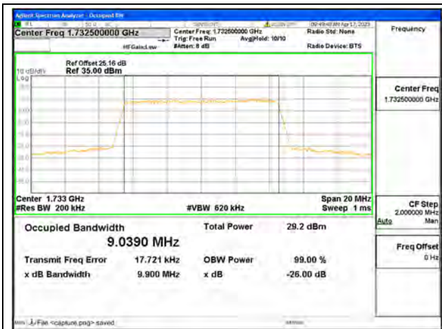
Band4 / 10MHz / QPSK/ Mid CH
