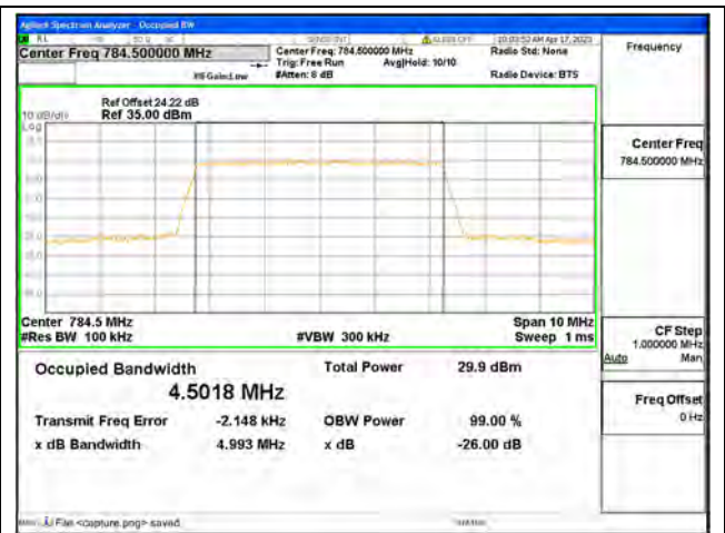
Band13 / 5MHz / 16QAM/ High CH
