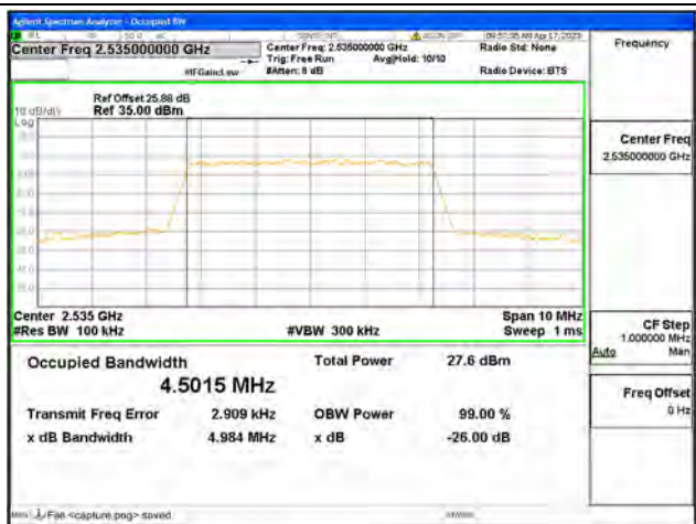
Band7 / 5MHz / 16QAM/ Mid CH
