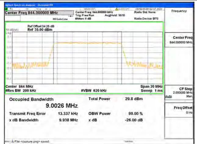
Band5 / 10MHz / QPSK/ High CH
