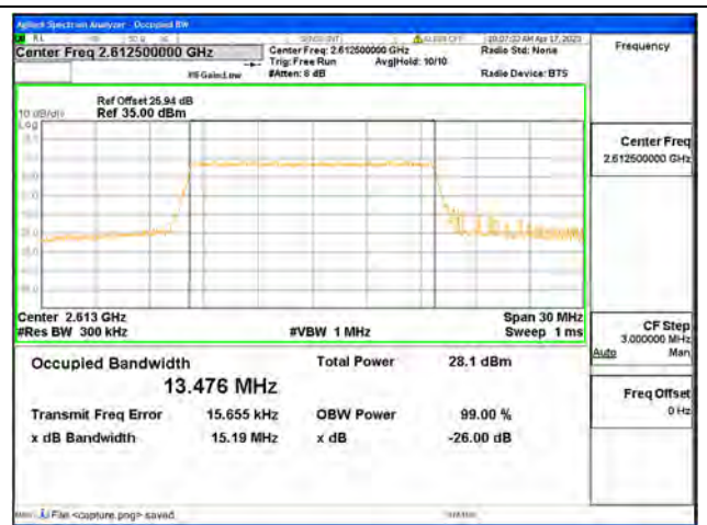
Band38 / 15MHz / 16QAM/ High CH
