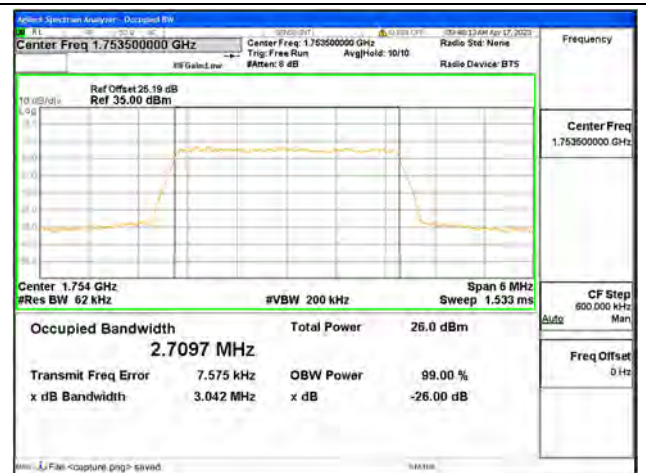
Band4 / 3MHz / 64QAM/ High CH
