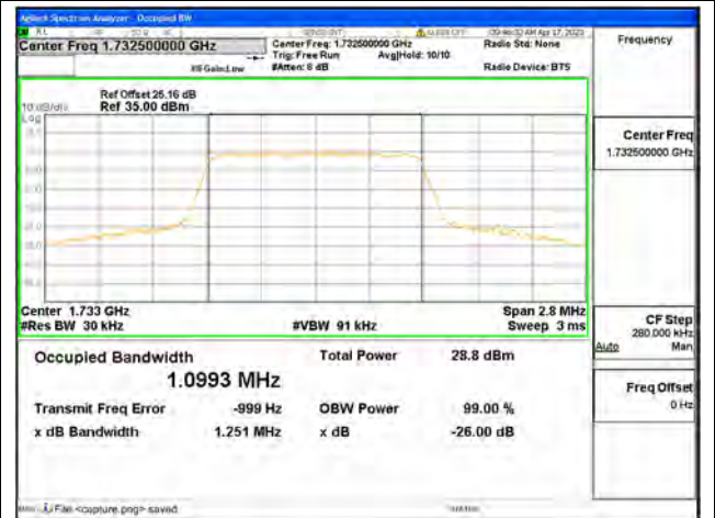
Band4 / 1.4MHz / QPSK/ Mid CH
