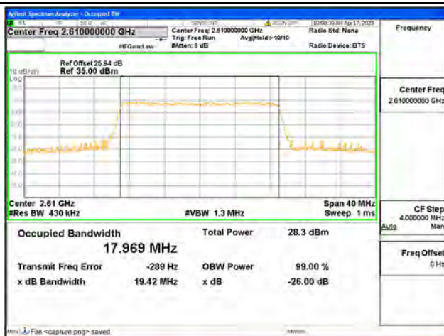
Band38 / 20MHz / 16QAM/ High CH
