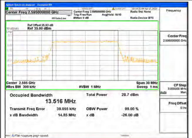
Band41(2535-2655) / 15MHz / QPSK/ Mid CH
