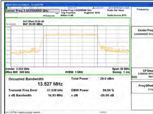
Band41(2535-2655) / 15MHz / QPSK/ Low CH
