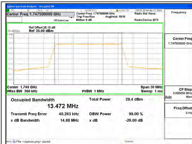
Band4 / 15MHz / QPSK/ High CH
