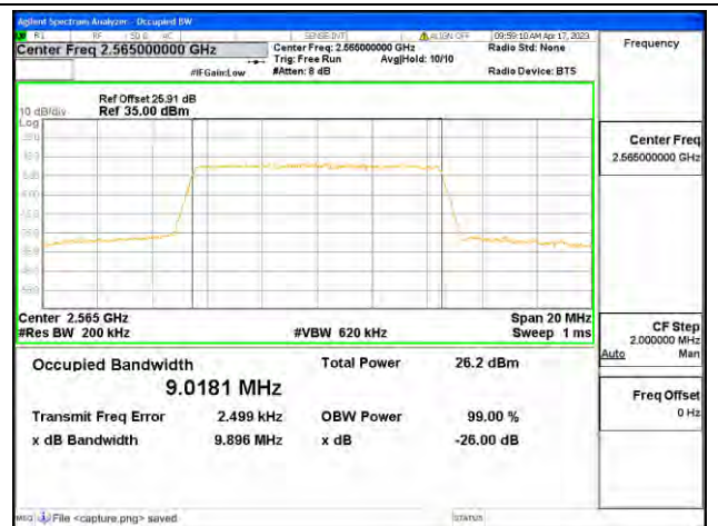
Band7 / 10MHz / 64QAM/ High CH
