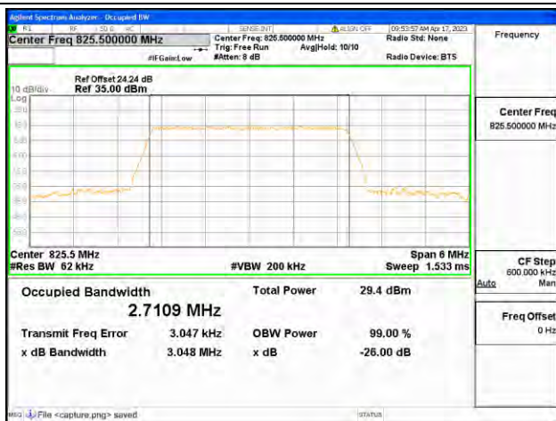
Band5 / 3MHz / 16QAM/ Low CH
