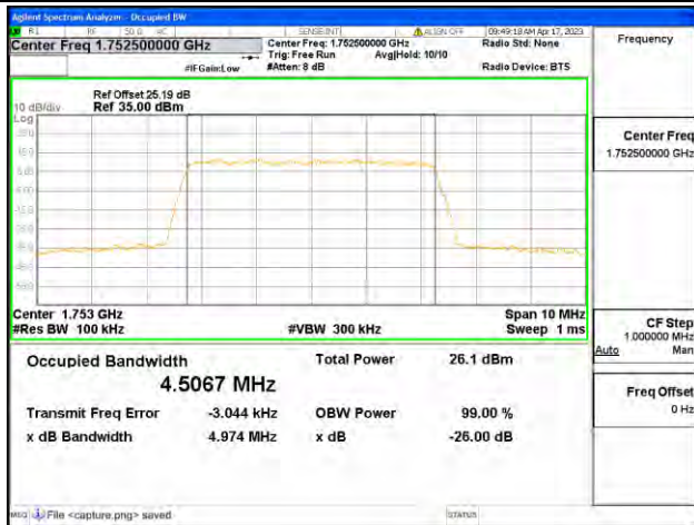
Band4 / 5MHz / 64QAM / High CH
