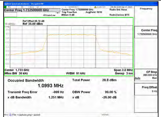
Band4 / 1.4MHz / QPSK/ Mid CH
