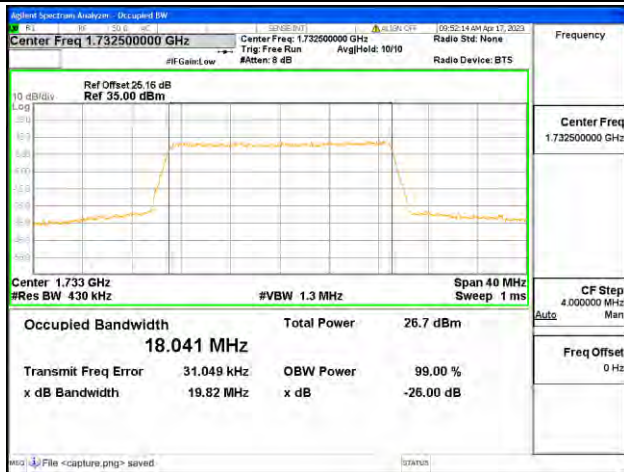
Band4 / 20MHz / 64QAM/ Mid CH
