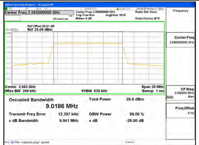
Band7 / 10MHz / QPSK/ High CH
