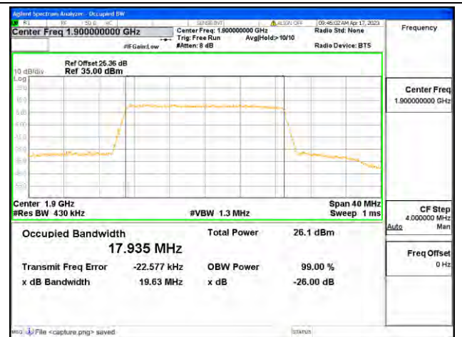
Band2 / 20MHz / 64QAM/ High CH
