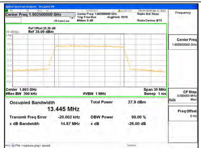
Band2 / 15MHz / 16QAM/ High CH
