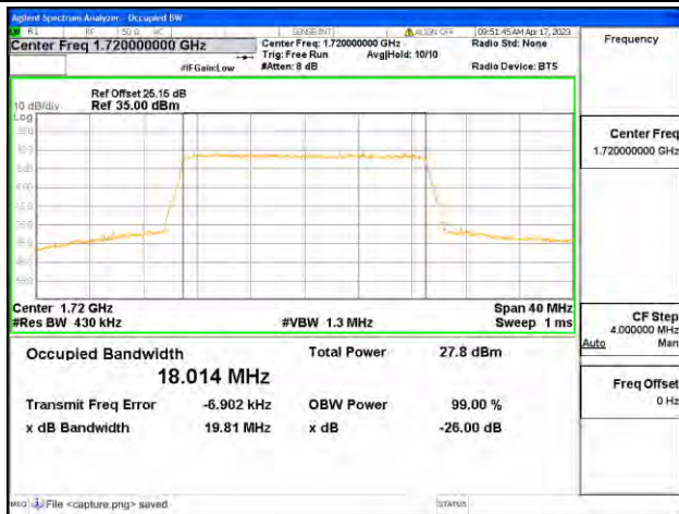
Band4 / 20MHz / 16QAM/ Low CH
