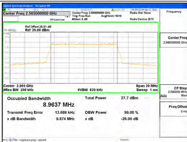
Band7 / 10MHz / 16QAM/ High CH
