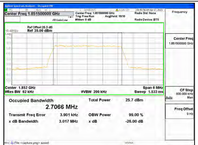
Band2 / 3MHz / 64QAM/ Low CH
