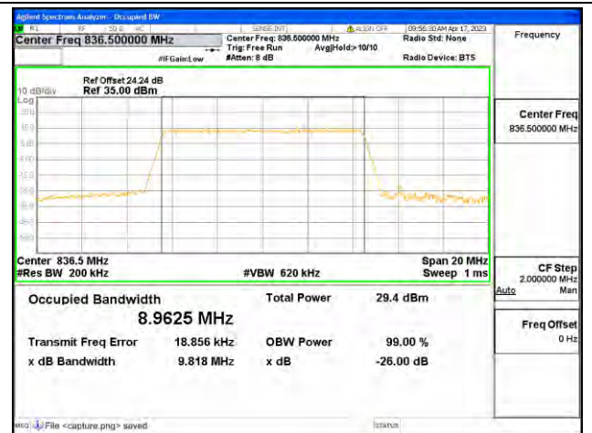
Band5 / 10MHz / 16QAM/ Mid CH
