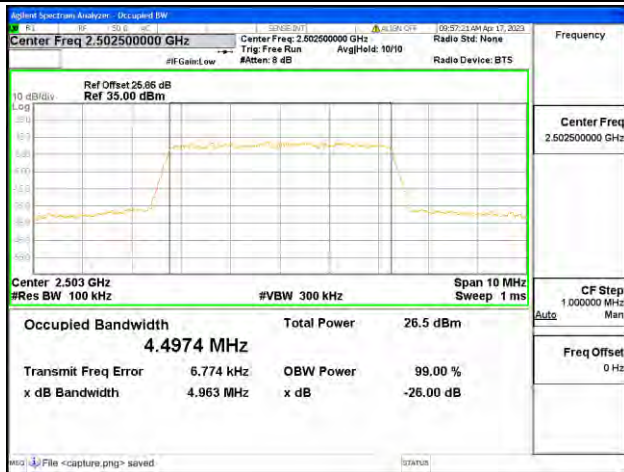
Band7 / 5MHz / 64QAM/ Low CH
