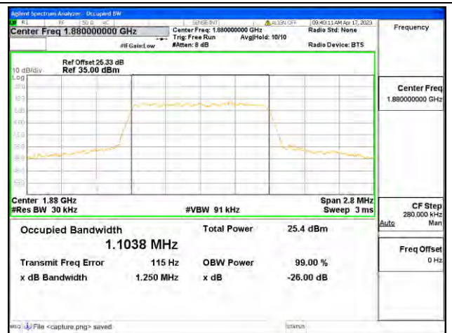
Band2 / 1.4MHz / 64QAM/ Mid CH
