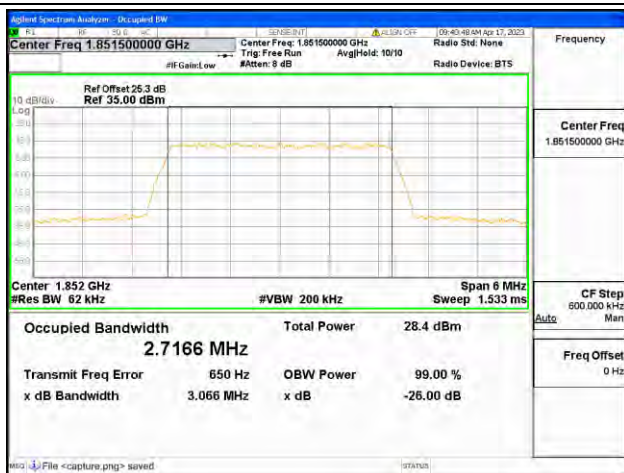
Band2 / 3MHz / 16QAM/ Low CH
