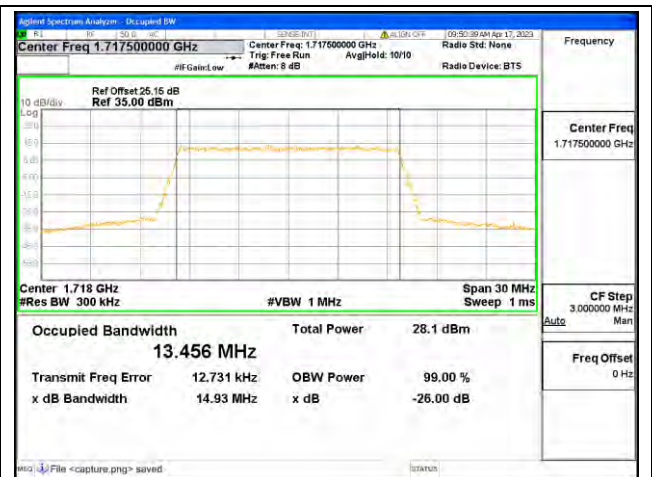
Band4 / 15MHz / 16QAM/ Low CH
