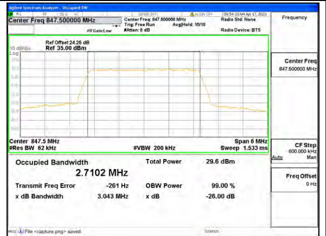
Band5 / 3MHz / QPSK/ High CH
