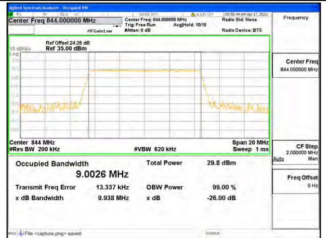
Band5 / 10MHz / QPSK/ High CH
