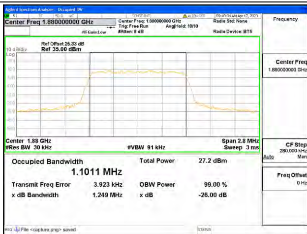
Band2 / 1.4MHz / 16QAM/ Mid CH
