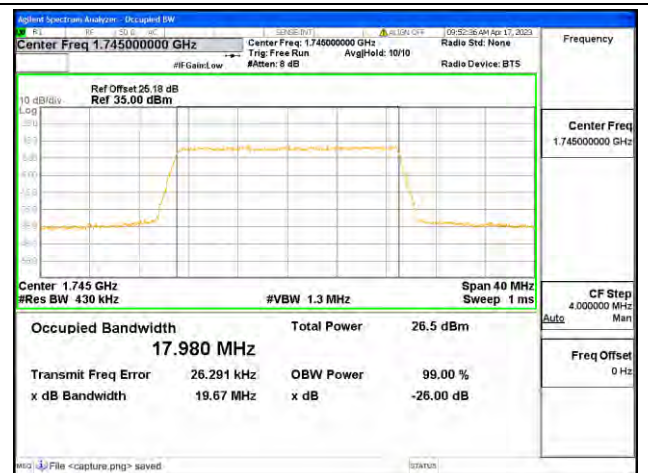
Band4 / 20MHz / 64QAM/ High CH
