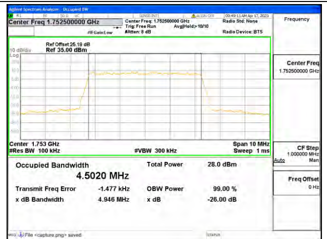
Band4 / 5MHz / 16QAM / High CH
