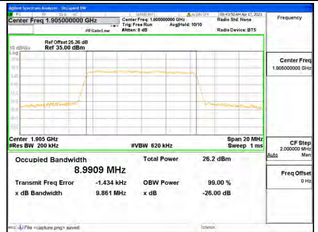
Band2 / 10MHz / 64QAM/ High CH
