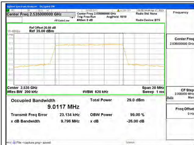
Band7 / 10MHz / QPSK/ Mid CH
