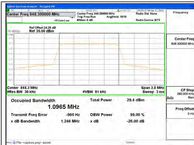
Band5 / 1.4MHz / QPSK/ High CH
