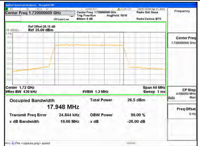
Band4 / 20MHz / 64QAM/ Low CH
