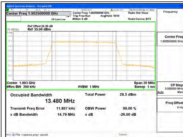
Band2 / 15MHz / QPSK/ High CH
