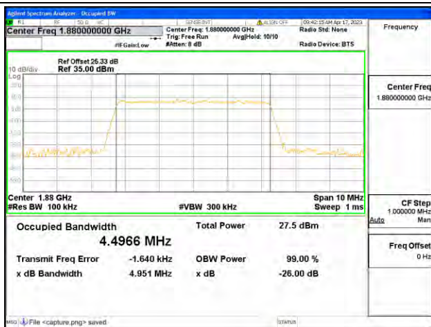
Band2 / 5MHz / 16QAM/ Mid CH
