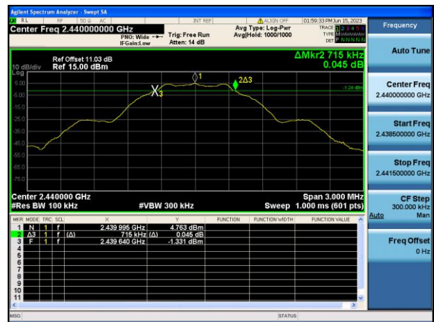
GFSK (BLE 1Mbps) MIDDLE CHANNEL
