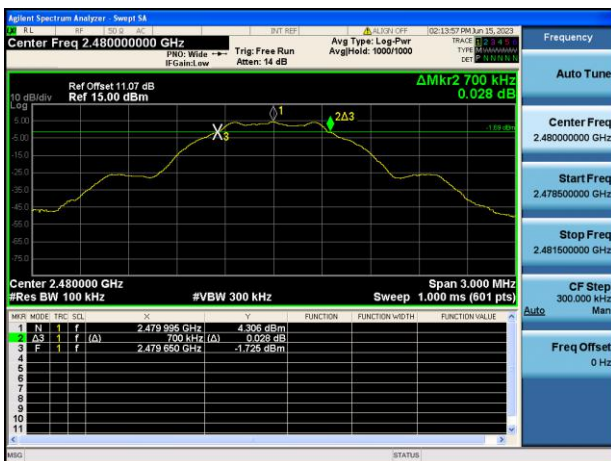
GFSK (BLE 1Mbps) HIGH CHANNEL
