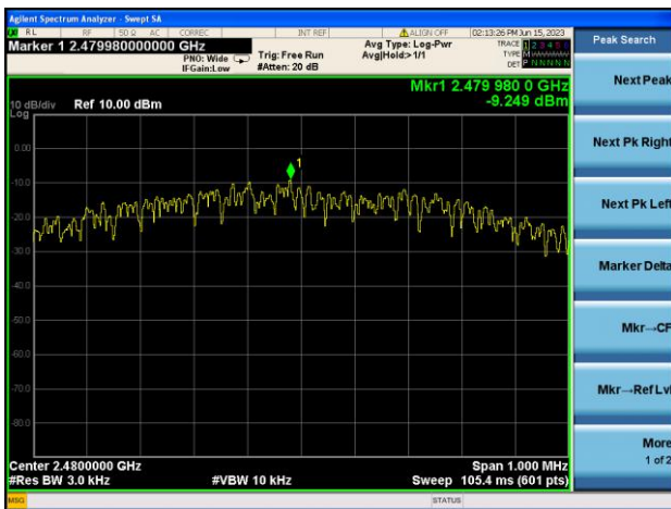
GFSK (BLE 1Mbps) HIGH CHANNEL
