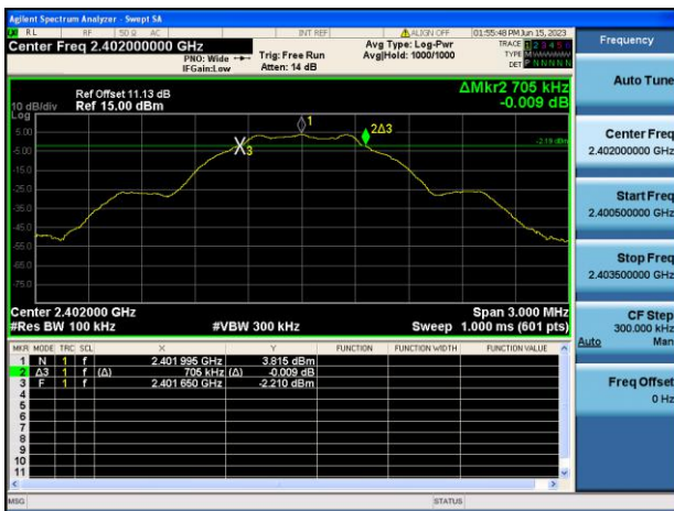
GFSK (BLE 1Mbps) LOW CHANNEL
