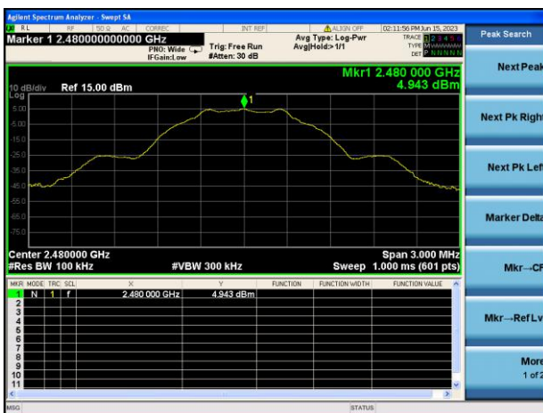
GFSK (BLE 1Mbps) HIGH CHANNEL, CARRIER LEVEL
