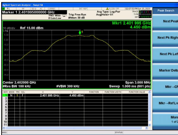
GFSK (BLE 1Mbps) LOW CHANNEL, CARRIER LEVEL
