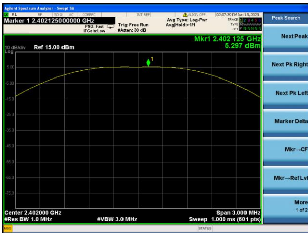
GFSK (BLE 1Mbps) LOW CHANNEL
