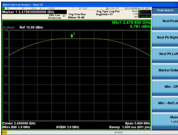
GFSK (BLE 1Mbps) HIGH CHANNEL
