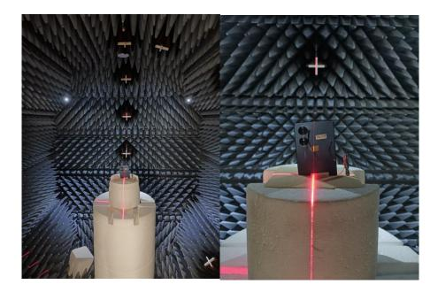
Fig.1. The DUT in the fully anechoic chamber
