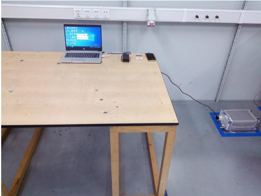
AC Conducted Emission Test Setup -Front
