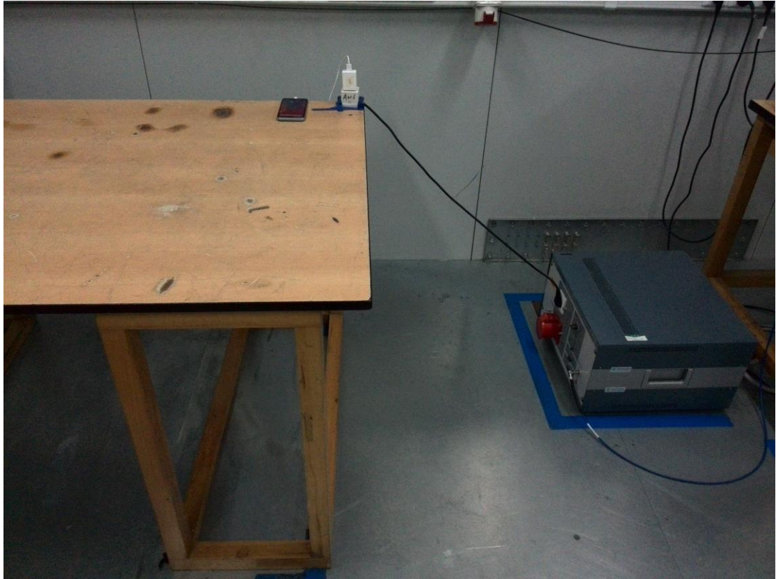
AC Conducted Emission Test Setup -Front
