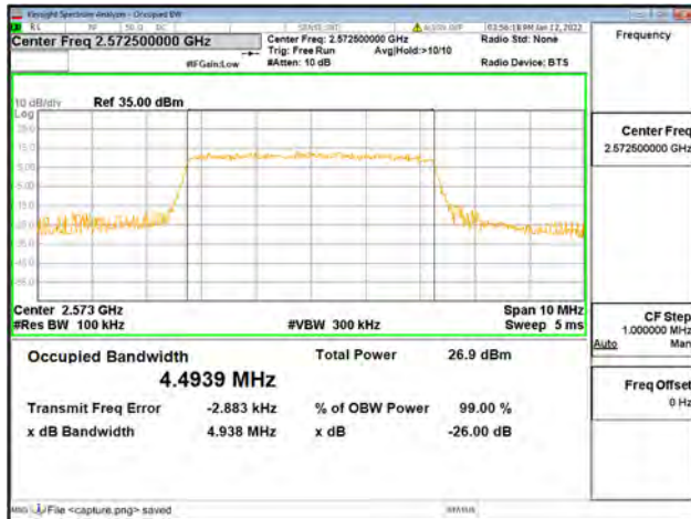
Band38 / 5MHz / Mid CH / 16QAM
