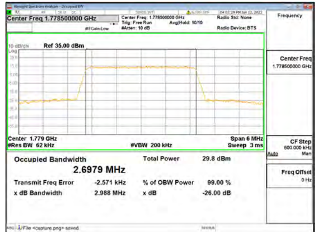
Band66 / 3MHz / High CH / 64QAM
