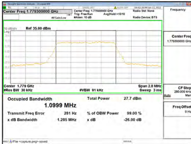
Band66 / 3MHz / Low CH / 16QAM
