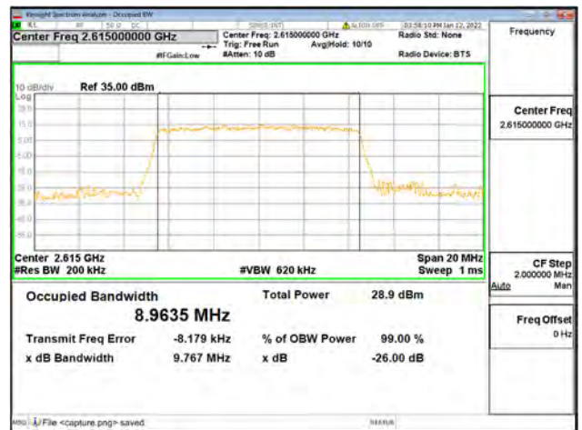
Band38 / 10MHz / High CH / 64QAM
