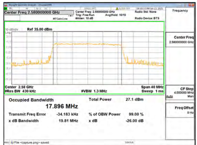
Band38 / 20MHz / Low CH / 64QAM
