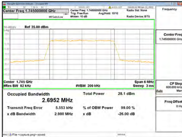
Band66 / 3MHz / High CH / 16QAM
