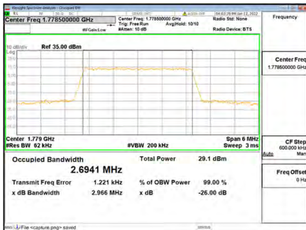
Band66 / 3MHz / High CH / 16QAM
