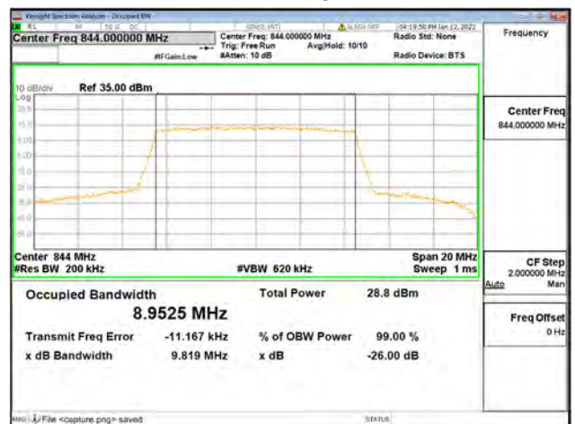
Band26 / 10MHz / High CH / 64QAM
