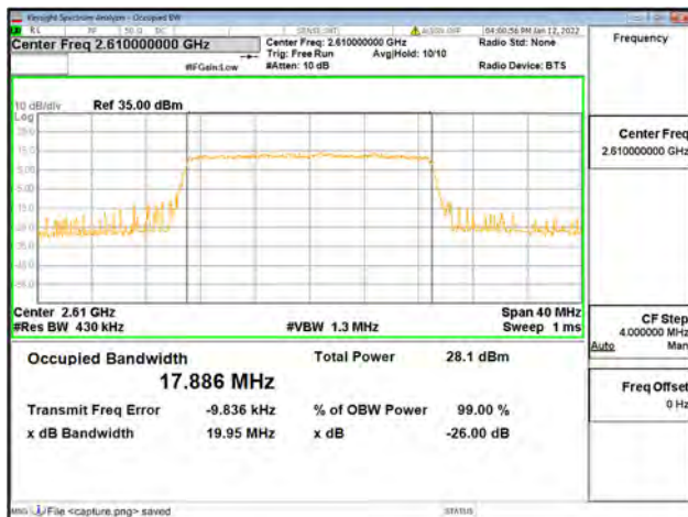
Band38 / 20MHz / High CH / 16QAM
