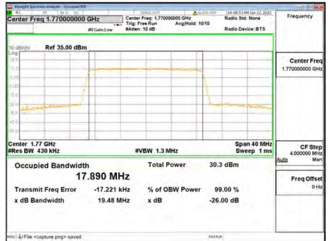
Band66 / 20MHz / High CH / 64QAM
