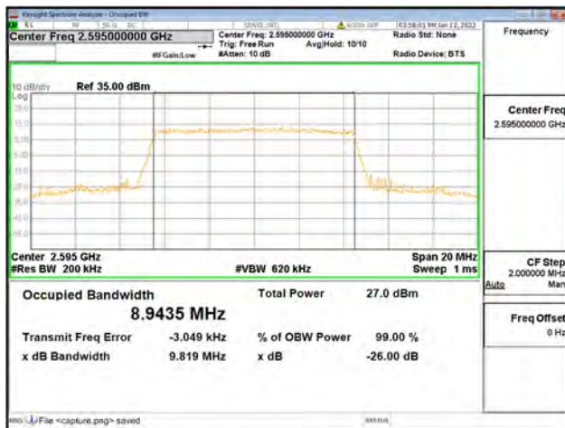
Band38 / 10MHz / High CH / 16QAM
