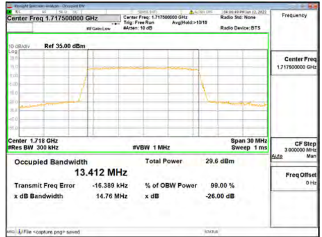
Band66 / 15MHz / Mid CH / QPSK
