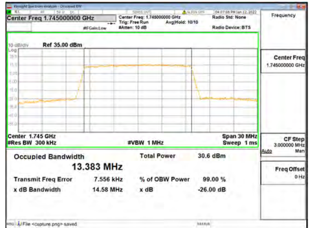
Band66 / 15MHz / Mid CH / 64QAM
