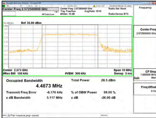
Band38 / 5MHz / Low CH / 64QAM
