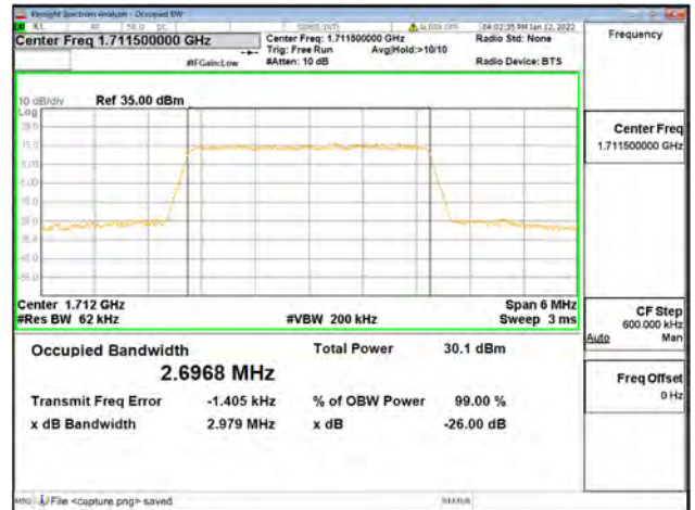
Band66 / 3MHz / Low CH / 64QAM
