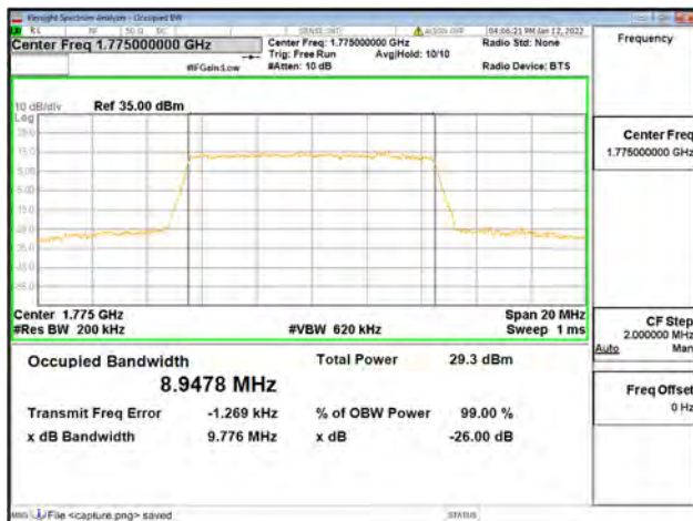
Band66 / 10MHz / High CH / 16QAM
