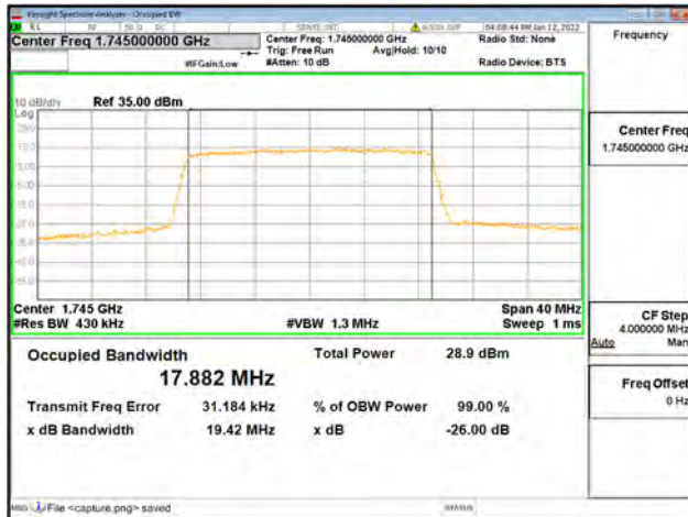
Band66 / 20MHz / High CH / 16QAM
