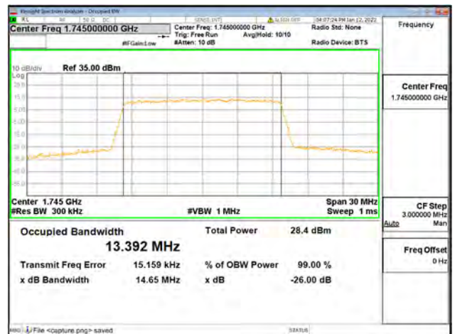
Band66 / 15MHz / Mid CH / 64QAM
