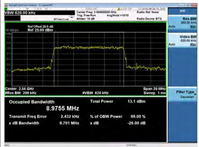
Band41 / 10MHz / Low CH / 64QAM
