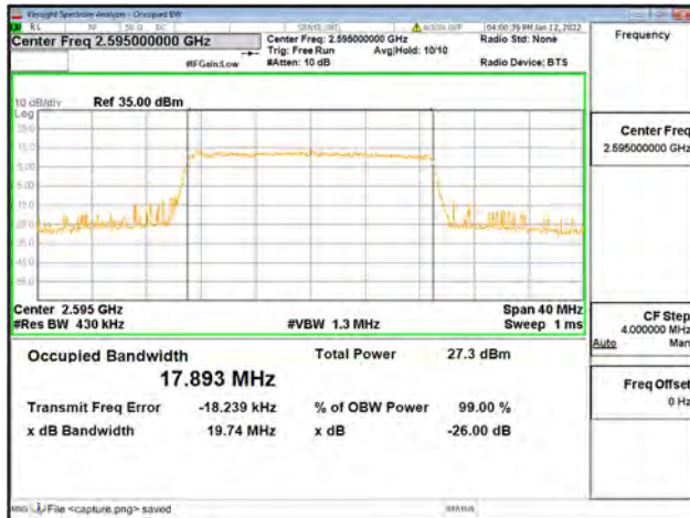
Band38 / 20MHz / High CH / 16QAM
