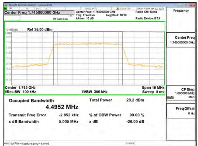
Band66 / 5MHz / Mid CH / 64QAM
