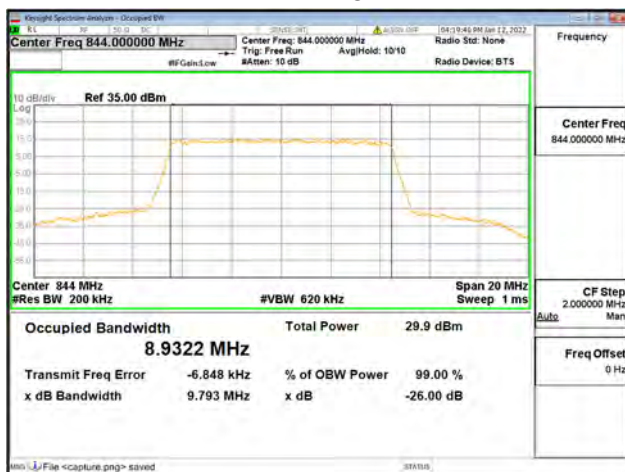
Band26 / 10MHz / High CH / 16QAM
