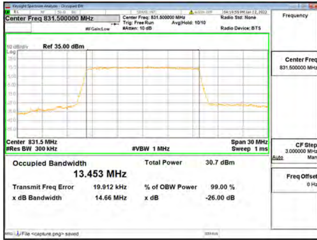
Band26 / 15MHz / Low CH / 64QAM
