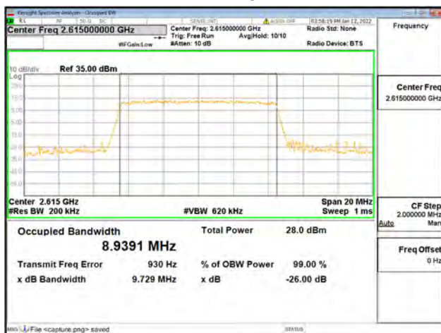
Band38 / 10MHz / High CH / 16QAM
