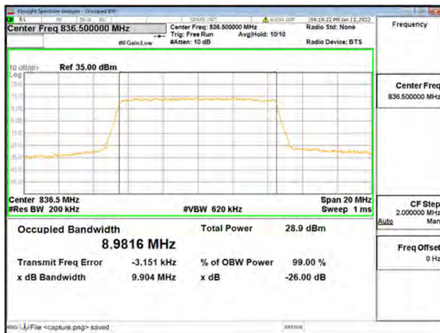
Band26 / 10MHz / High CH / 16QAM
