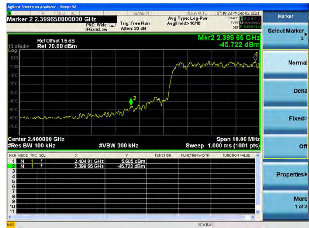
(Band edge with hopping on, Channel 0, 8-DPSK)
