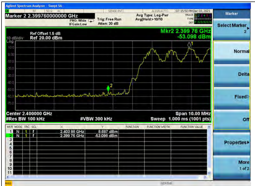
(Band edge with hopping on, Channel 0, GFSK)
