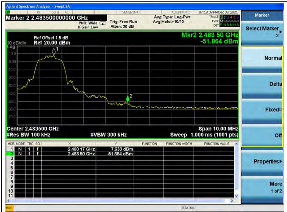
(Band edge, Channel 78, \pi/4 -DQPSK)
