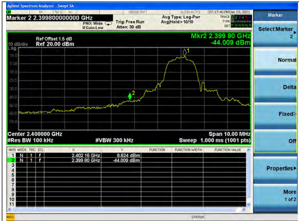
(Band edge, Channel 0, \pi/4 -DQPSK)
