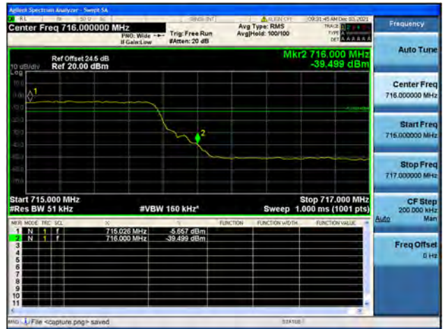
Band12 / 5MHz / High CH / QPSK / FULL RB
