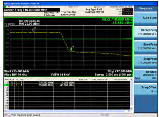
Band12 / 1.4MHz / High CH / QPSK / FULL RB
