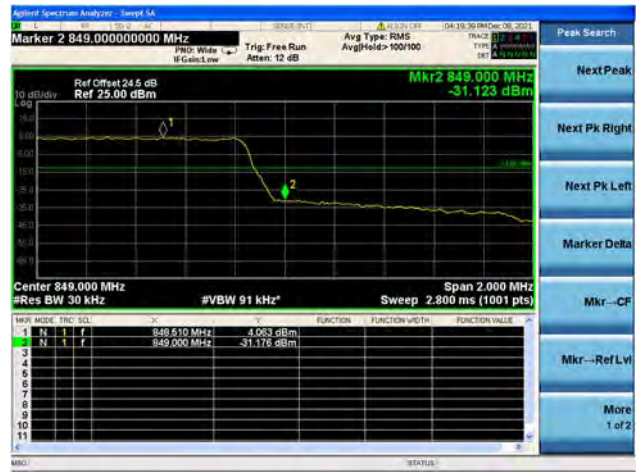
Band26 / 1.4MHz / High CH / QPSK / FULL RB
