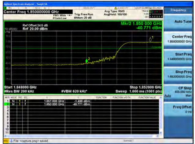
Band2 / 20MHz / High CH / QPSK / FULL RB
