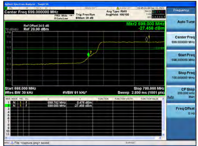
Band12 / 3MHz / High CH / QPSK / FULL RB
