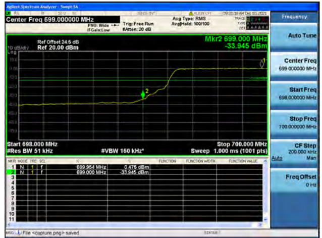
Band12 / 5MHz / High CH / QPSK / FULL RB
