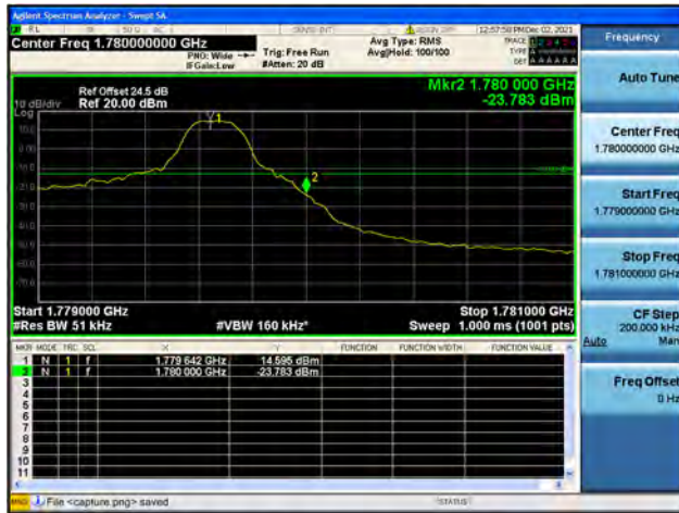
Band66 / 5MHz / High CH / QPSK / 1 RB
