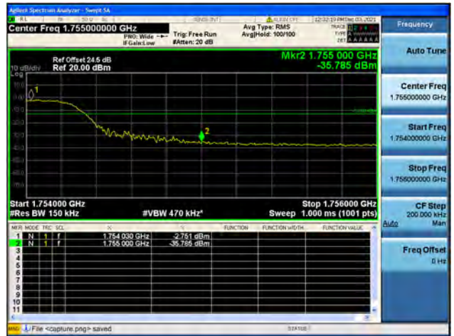
Band4 / 15MHz / High CH / QPSK / FULL RB
