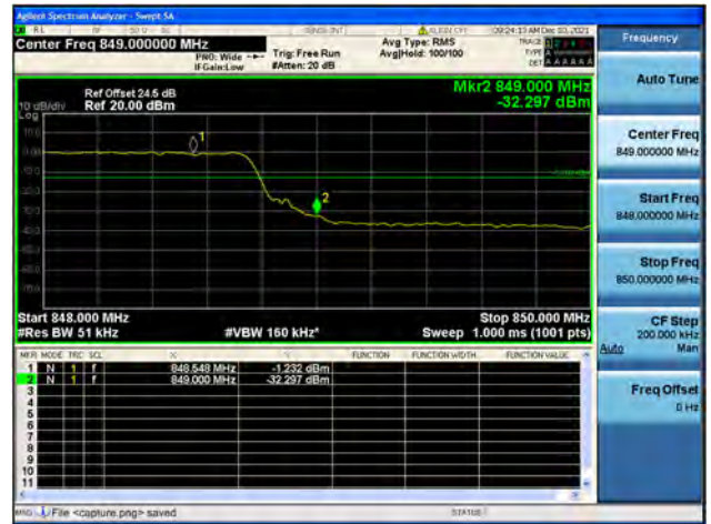
Band5 / 5MHz / High CH / QPSK / FULL RB
