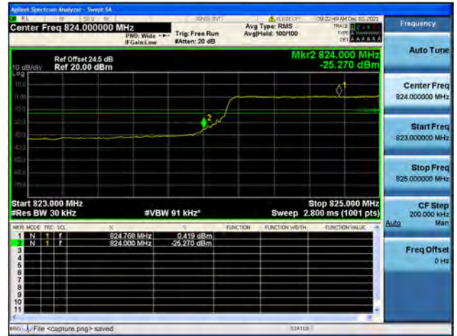
Band5 / 3MHz / High CH / QPSK / FULL RB
