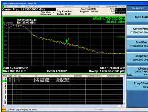
Band4 / 15MHz / High CH / QPSK / 1 RB
