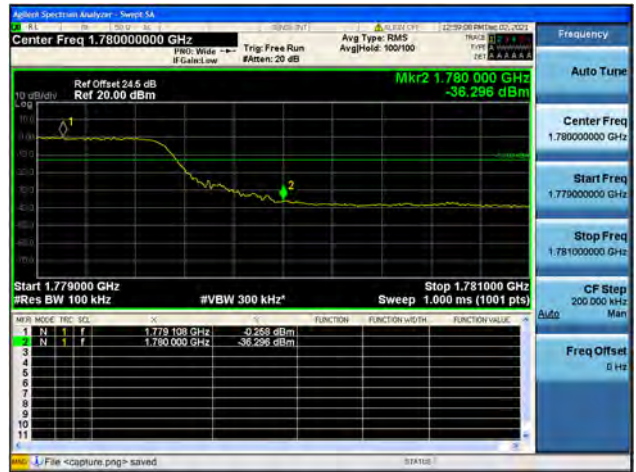
Band66 / 10MHz / High CH / QPSK / FULL RB
