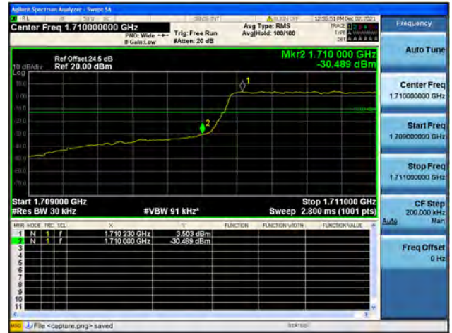
Band66 / 1.4MHz / High CH / QPSK / FULL RB
