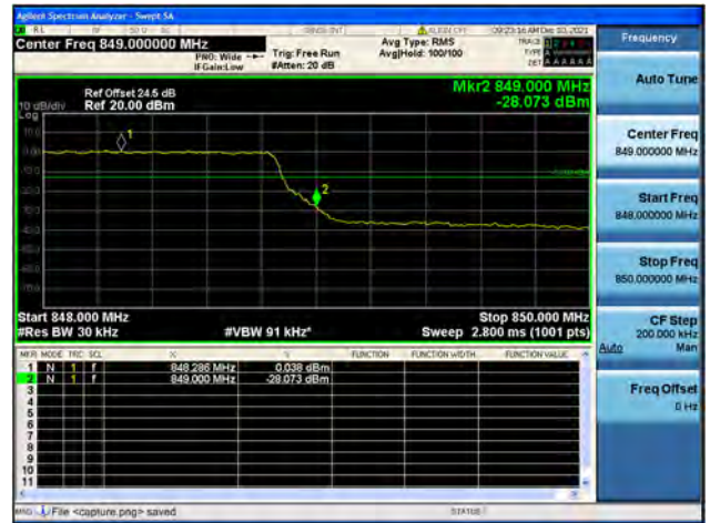
Band5 / 3MHz / High CH / QPSK / FULL RB
