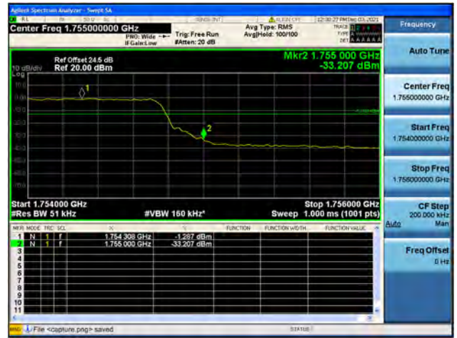
Band4 / 5MHz / High CH / QPSK / FULL RB
