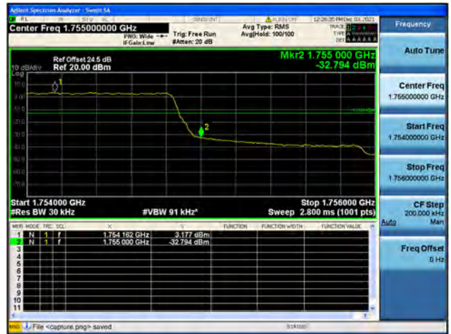
Band4 / 1.4MHz / High CH / QPSK / FULL RB
