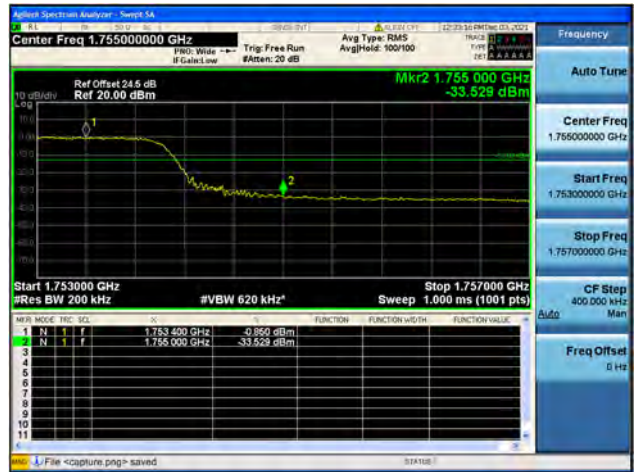
Band4 / 20MHz / High CH / QPSK / FULL RB
