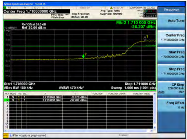
Band66 / 15MHz / High CH / QPSK / FULL RB
