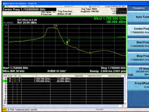
Band4 / 1.4MHz / High CH / QPSK / 1 RB
