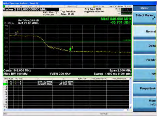
Band26 / 10MHz / High CH / QPSK / FULL RB
