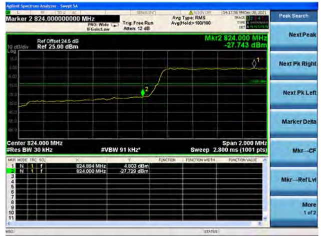
Band26 / 1.4MHz / High CH / QPSK / FULL RB
