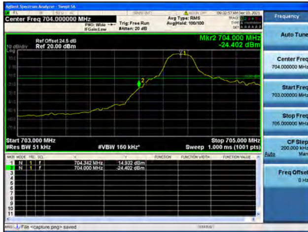
Band17 / 5MHz / High CH / QPSK / 1 RB
