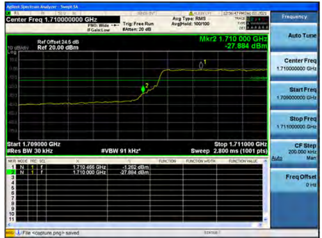
Band66 / 3MHz / High CH / QPSK / FULL RB
