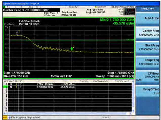
Band66 / 15MHz / High CH / QPSK / FULL RB
