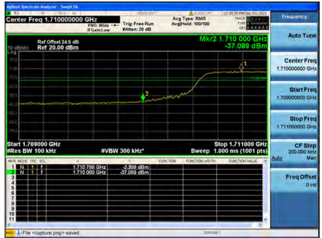
Band4 / 10MHz / High CH / QPSK / FULL RB
