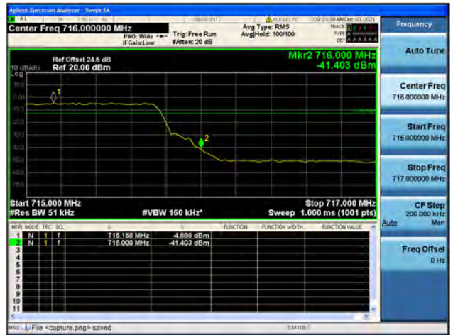
Band17 / 5MHz / High CH / QPSK / FULL RB
