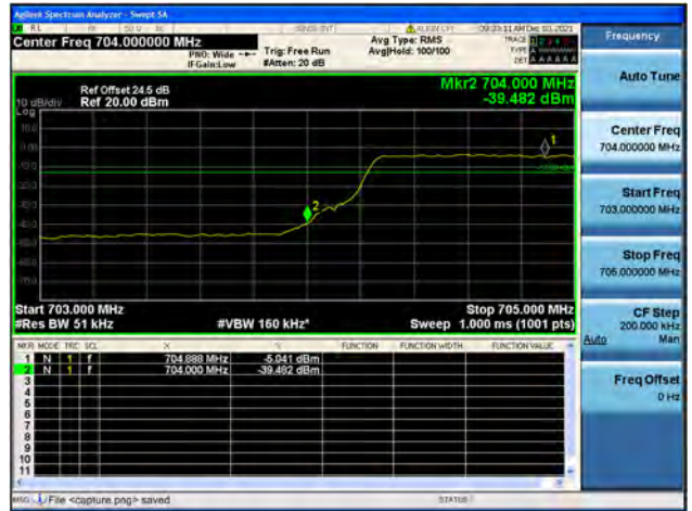
Band17 / 5MHz / High CH / QPSK / FULL RB
