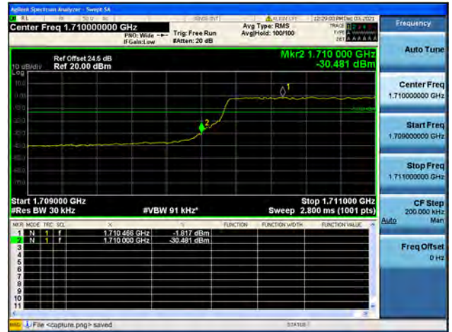
Band4 / 3MHz / High CH / QPSK / FULL RB
