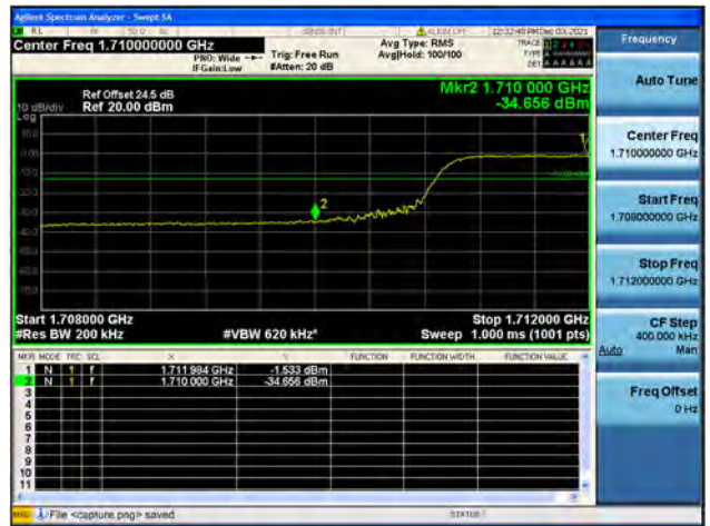
Band4 / 20MHz / High CH / QPSK / FULL RB
