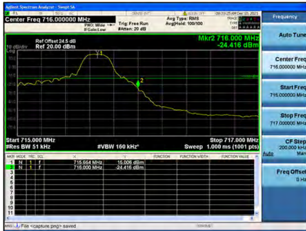
Band17 / 5MHz / High CH / QPSK / 1 RB
