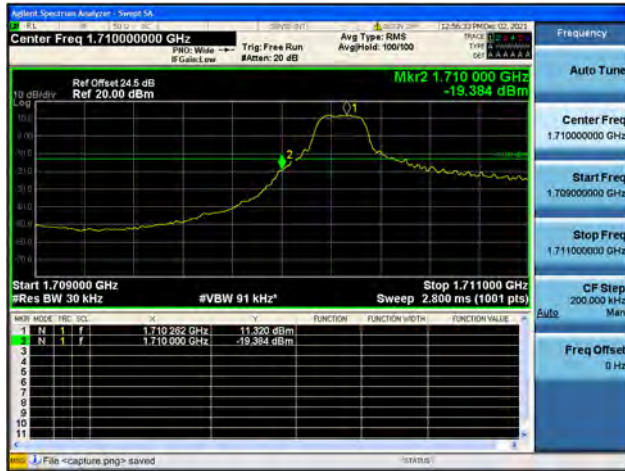
Band66 / 3MHz / High CH / QPSK / 1 RB
