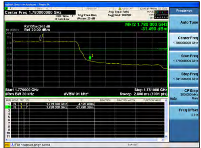
Band66 / 1.4MHz / High CH / QPSK / FULL RB
