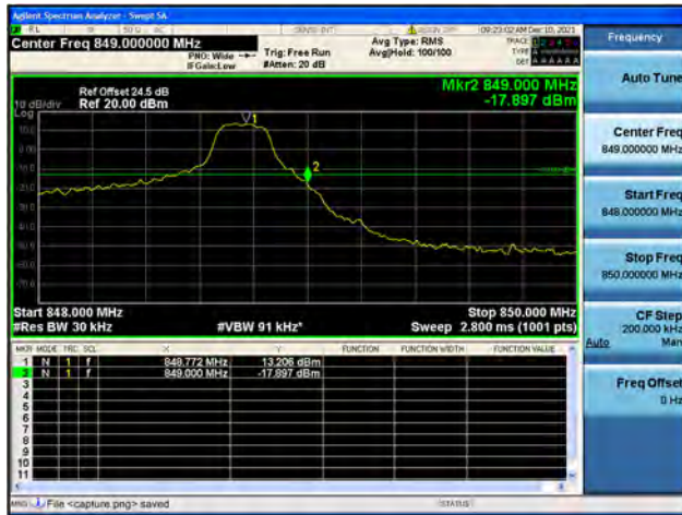
Band5 / 3MHz / High CH / QPSK / 1 RB
