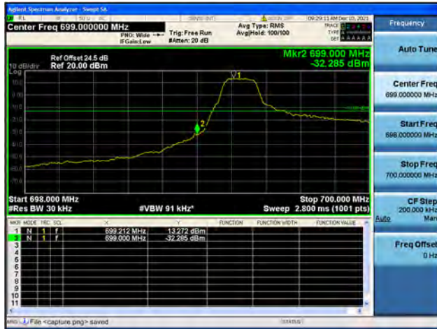
Band12 / 1.4MHz / High CH / QPSK / 1 RB
