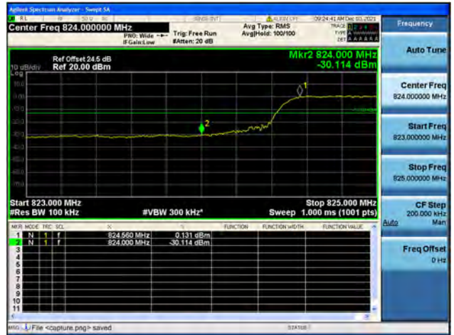
Band5 / 10MHz / High CH / QPSK / FULL RB
