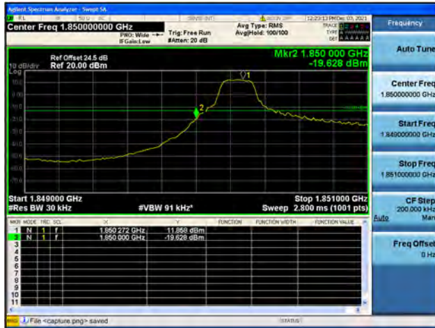
Band2 / 3MHz / High CH / QPSK / 1 RB
