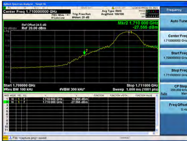
Band4 / 10MHz / High CH / QPSK / 1 RB
