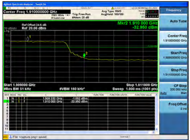
Band2 / 5MHz / High CH / QPSK / FULL RB
