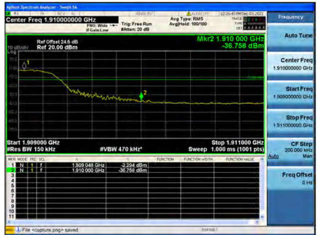
Band2 / 15MHz / High CH / QPSK / FULL RB
