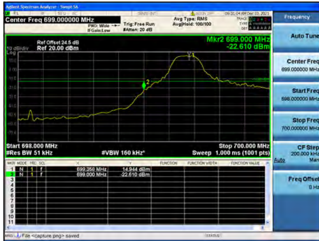
Band12 / 5MHz / High CH / QPSK / 1 RB
