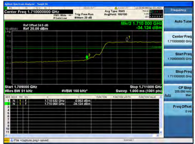
Band4 / 5MHz / High CH / QPSK / FULL RB
