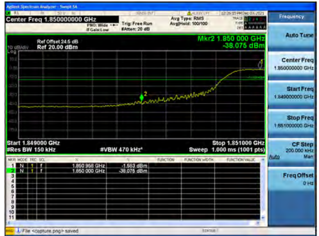
Band2 / 15MHz / High CH / QPSK / FULL RB
