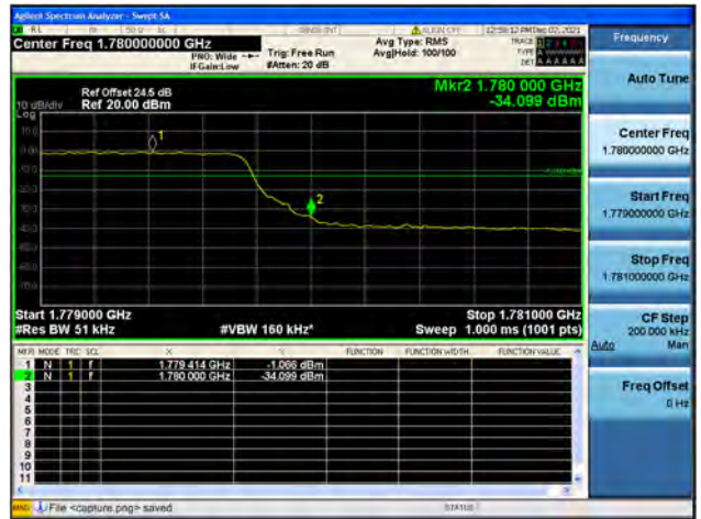
Band66 / 5MHz / High CH / QPSK / FULL RB
