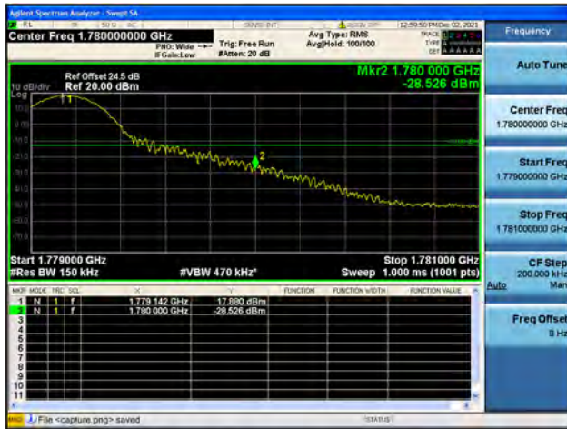
Band66 / 15MHz / High CH / QPSK / 1 RB
