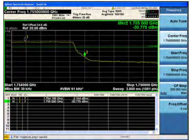
Band4 / 3MHz / High CH / QPSK / FULL RB
