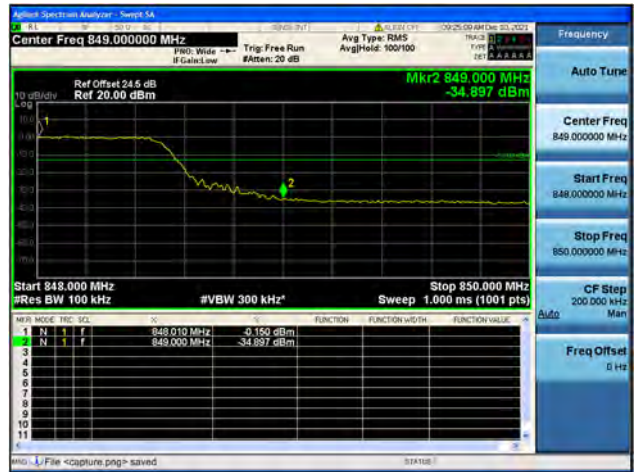
Band5 / 10MHz / High CH / QPSK / FULL RB
