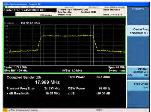
Band4 / 20MHz / High CH / 64QAM
