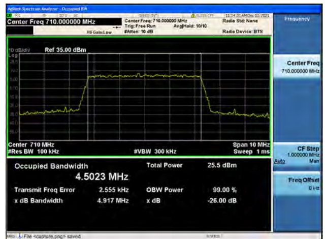
Band17 / 5MHz / Mid CH / 64QAM
