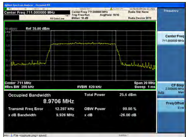
Band17 / 10MHz / High CH / 64QAM
