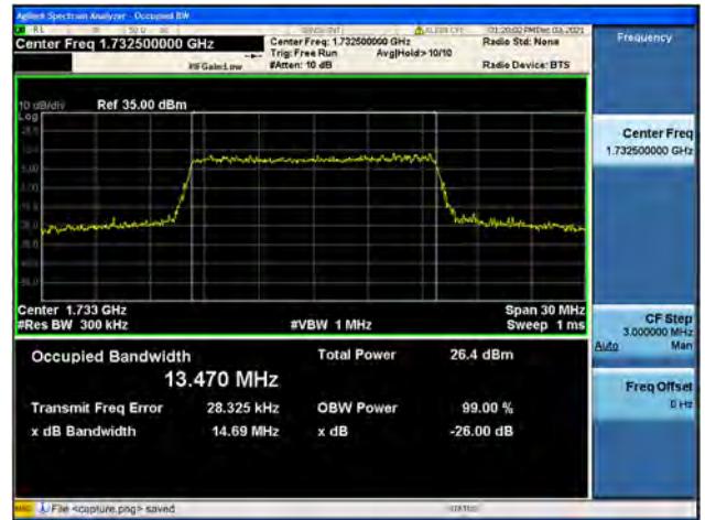
Band4 / 15MHz / Mid CH / 64QAM
