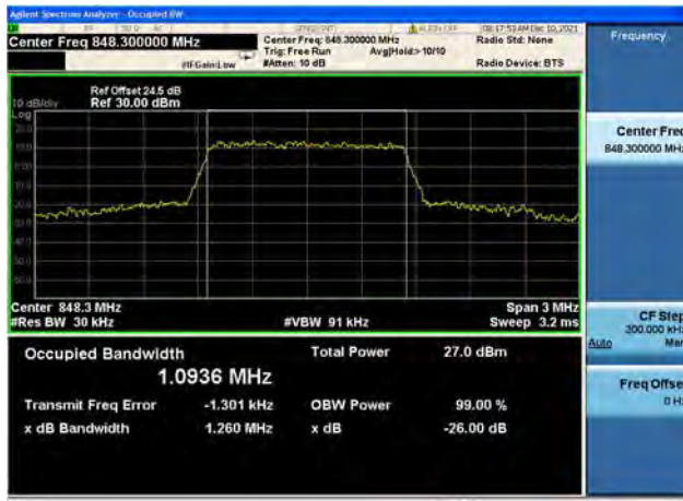
Band26 / 3MHz / Low CH / 16QAM
