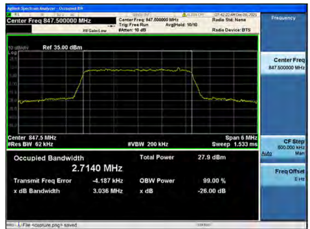
Band5 / 3MHz / High CH / 64QAM
