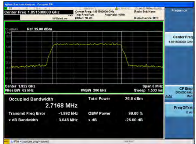
Band2 / 3MHz / Low CH / 64QAM
