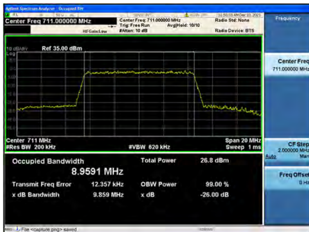
Band12 / 10MHz / High CH / 16QAM
