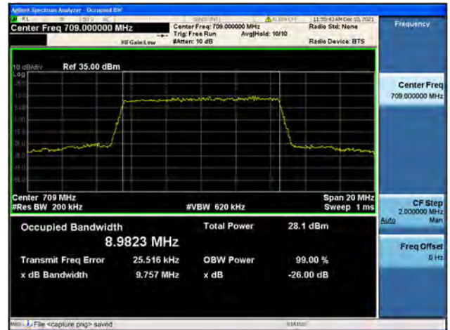
Band17 / 10MHz / Low CH / 64QAM
