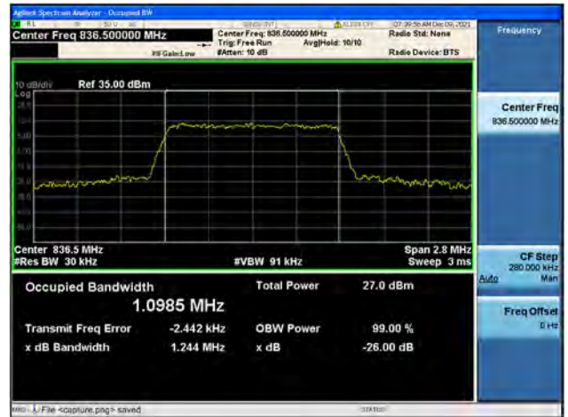
Band5 / 1.4MHz / Mid CH / 64QAM
