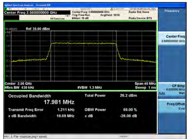
Band7 / 20MHz / High CH / 64QAM
