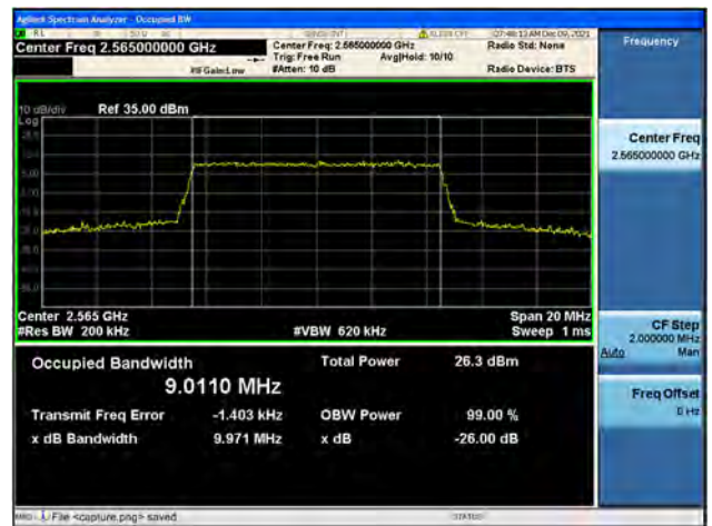
Band7 / 10MHz / High CH / 64QAM
