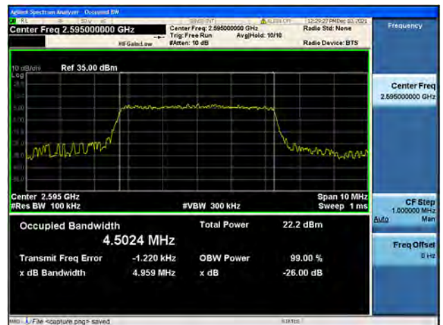
Band38 / 5MHz / Mid CH / 64QAM
