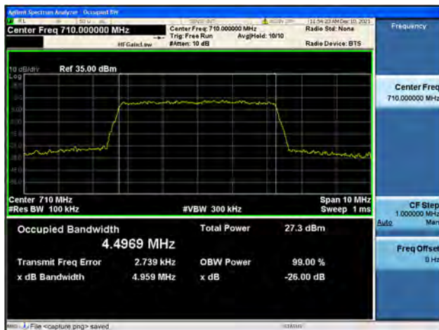
Band17 / 5MHz / Mid CH / 16QAM
