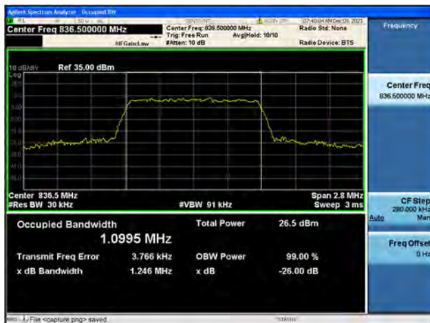
Band5 / 1.4MHz / Mid CH / 16QAM
