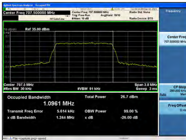
Band12 / 1.4MHz / Mid CH / 16QAM
