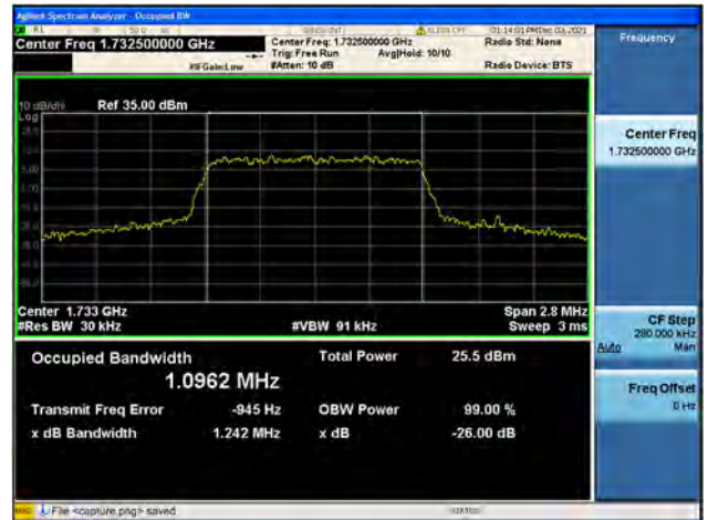
Band4 / 1.4MHz / Mid CH / 64QAM
