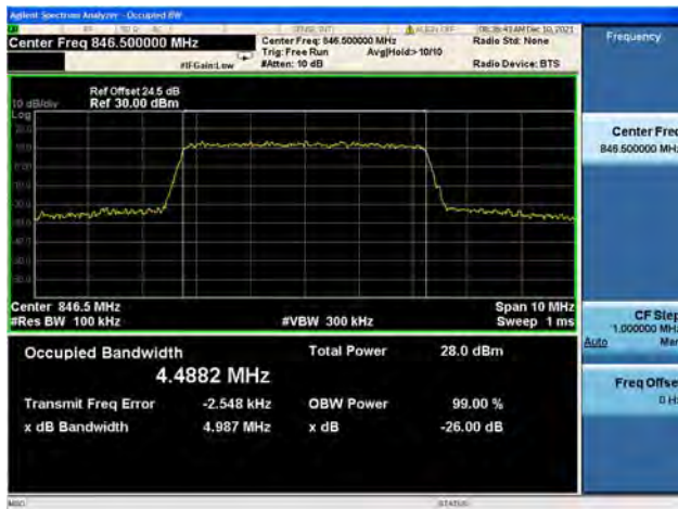
Band26 / 5MHz / High CH / 64QAM
