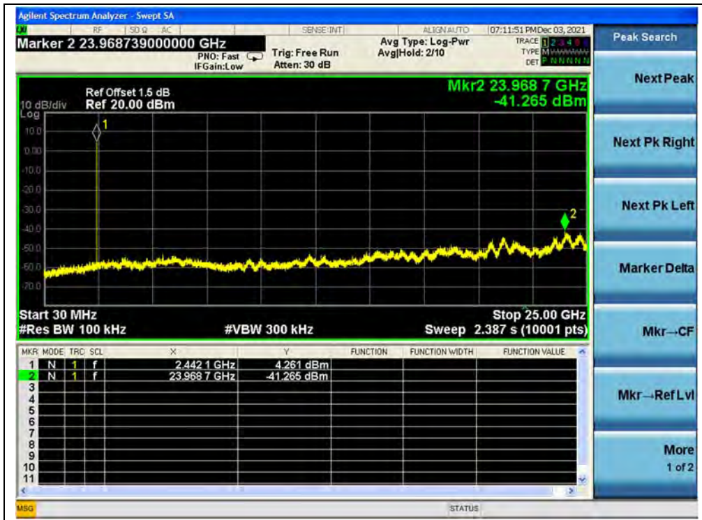
(30MHz to 25GHz, Channel 39, 8-DPSK)
