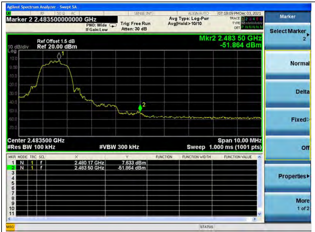
(Band edge, Channel 78, \pi/4 -DQPSK)
