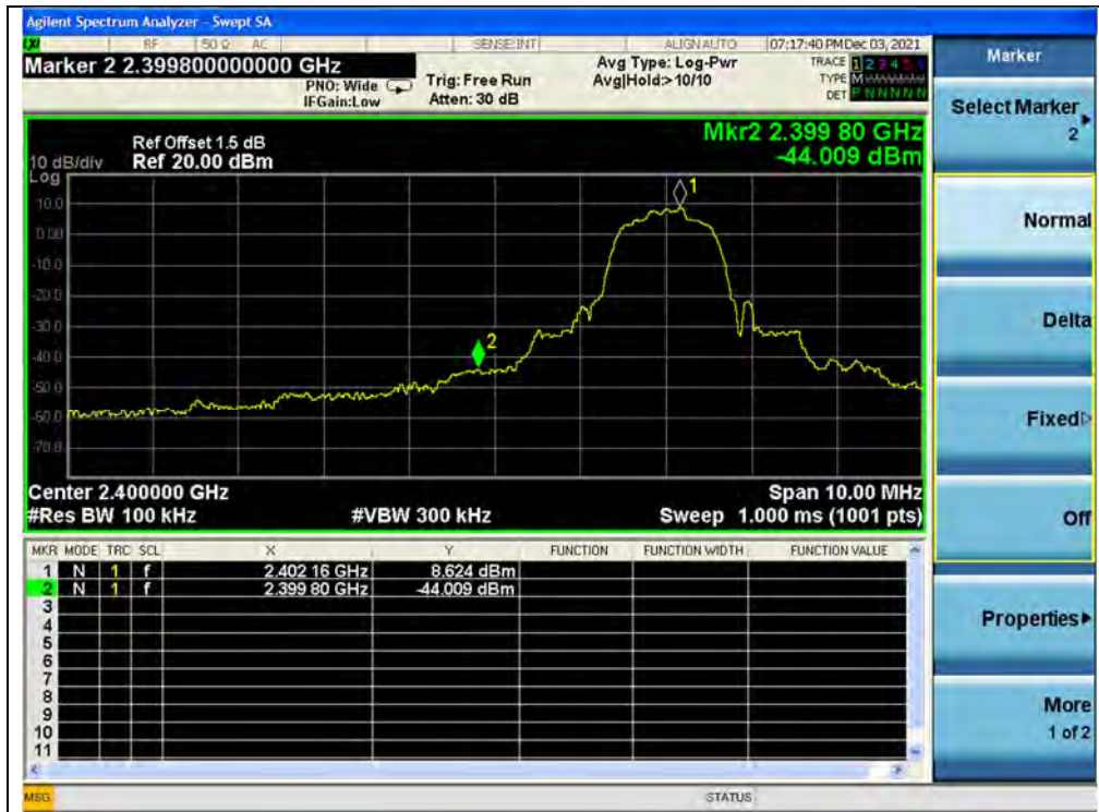
(Band edge, Channel 0, \pi/4 -DQPSK)
