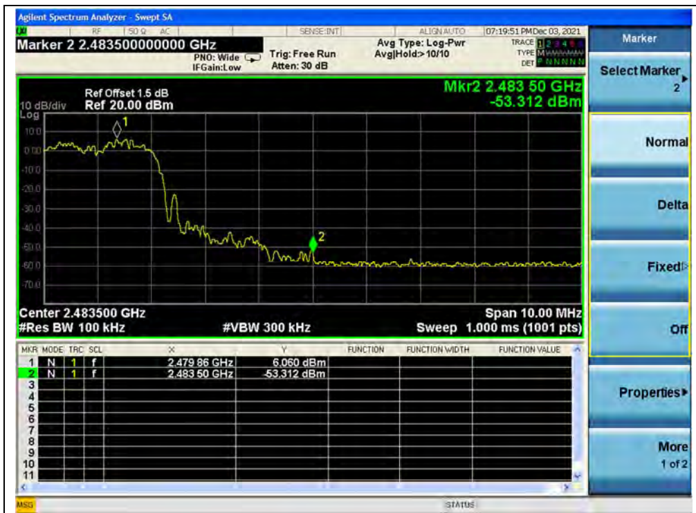
(Band edge with hopping on, Channel 78, 8-DPSK)
