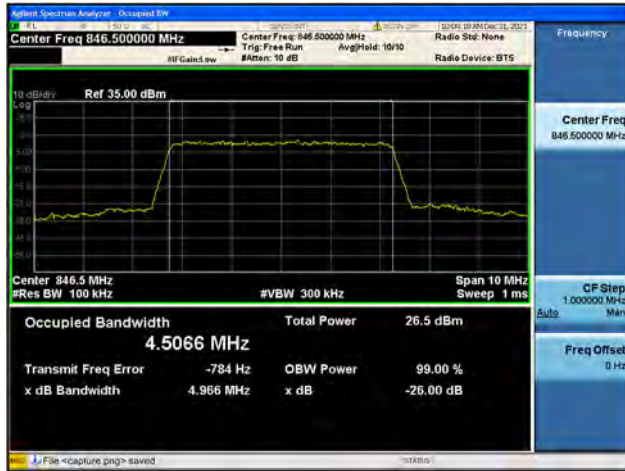
Band26 / 5MHz / High CH / 64QAM
