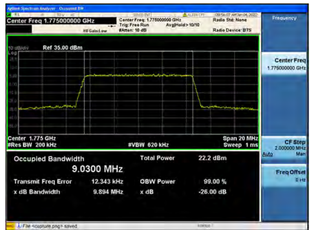
Band66 / 10MHz / High CH / 64QAM
