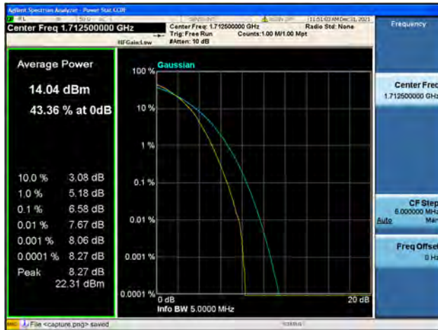
Band4 / 5MHz / Mid CH / 16QAM
