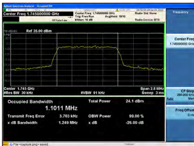
Band66 / 1.4MHz / Mid CH / 16QAM
