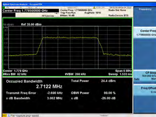
Band66 / 3MHz / High CH / 16QAM
