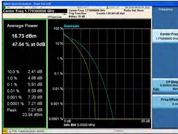
Band66 / 1.4MHz / High CH / 64QAM
