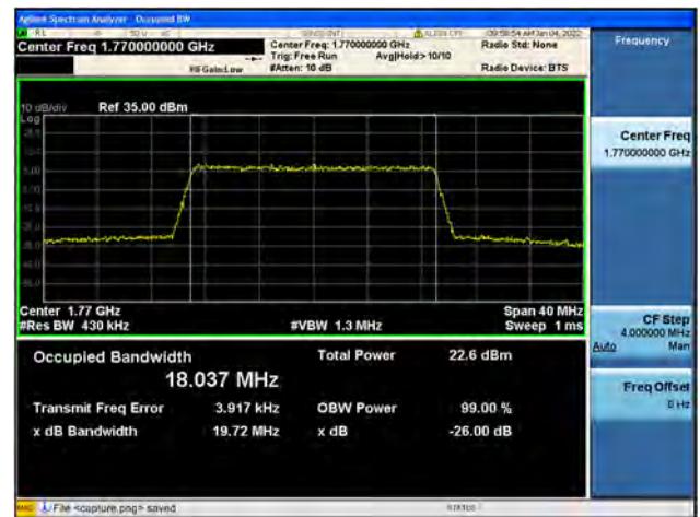
Band66 / 20MHz / High CH / 64QAM
