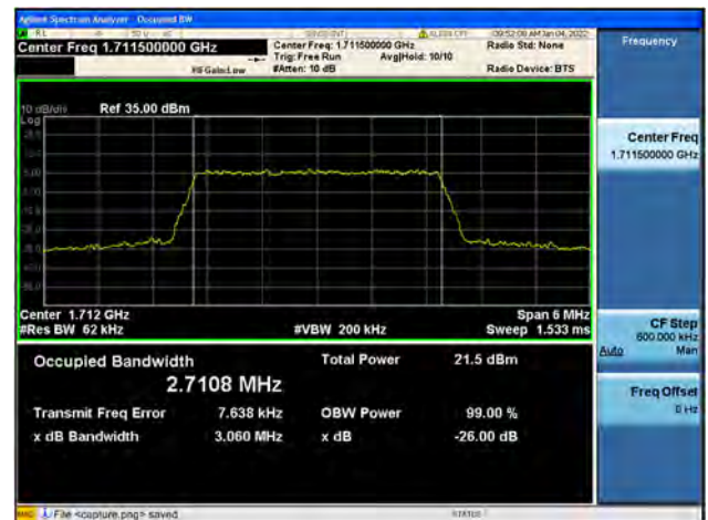
Band66 / 3MHz / Low CH / 64QAM
