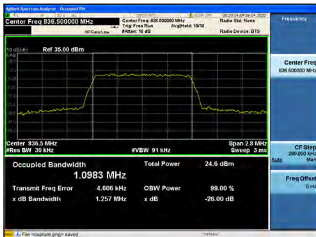
Band5 / 1.4MHz / Mid CH / 16QAM
