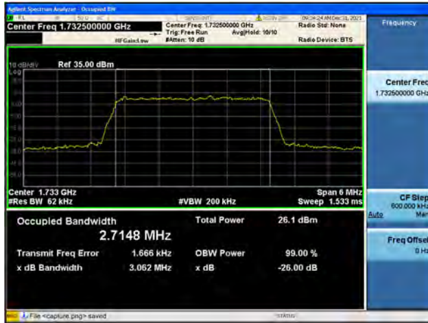
Band4 / 3MHz / Mid CH / 64QAM
