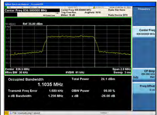
Band26 / 1.4MHz / Mid CH / 64QAM
