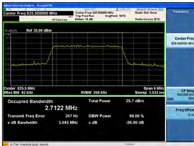
Band5 / 3MHz / Low CH / 16QAM
