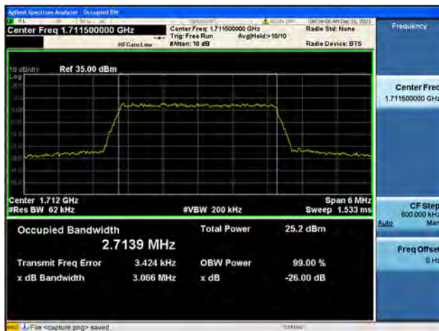
Band4 / 3MHz / Low CH / 16QAM
