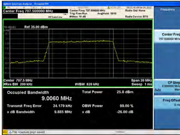
Band12 / 10MHz / Mid CH / 64QAM
