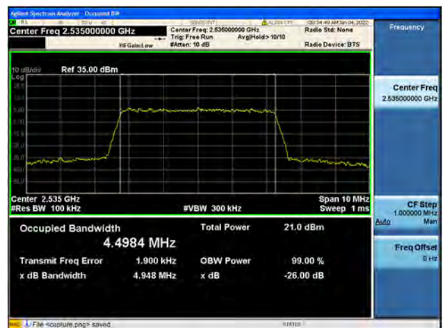
Band7 / 5MHz / Mid CH / 64QAM
