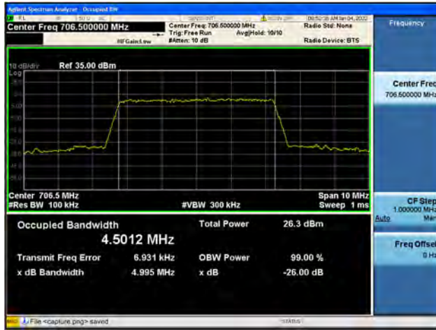
Band17 / 5MHz / Low CH / 64QAM
