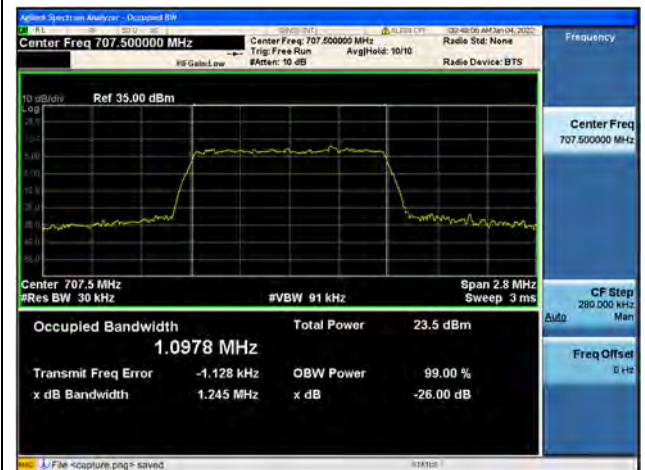
Band12 / 1.4MHz / Mid CH / 64QAM
