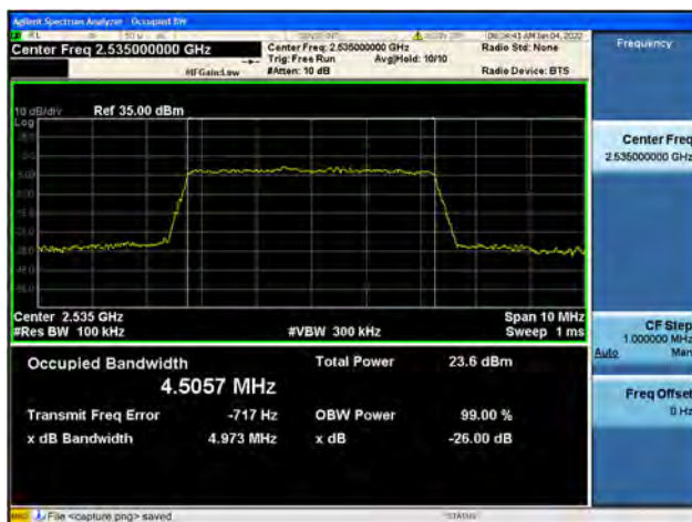
Band7 / 5MHz / Mid CH / 16QAM
