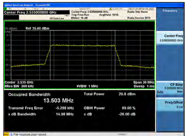
Band7 / 15MHz / Mid CH / 64QAM
