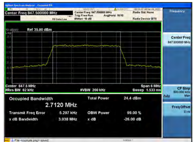
Band5 / 3MHz / High CH / 64QAM
