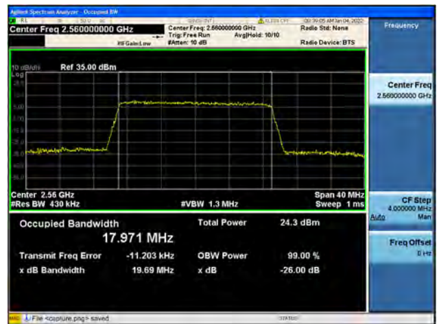
Band7 / 20MHz / High CH / 64QAM
