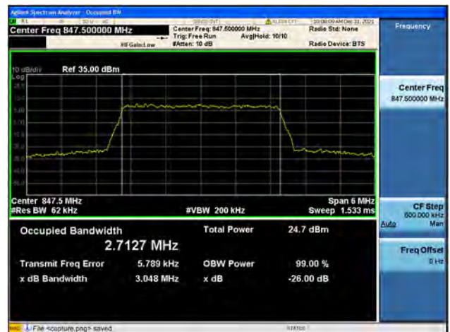
Band26 / 3MHz / High CH / 64QAM
