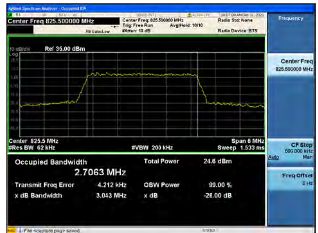
Band26 / 3MHz / Low CH / 64QAM
