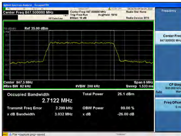
Band5 / 3MHz / High CH / 16QAM
