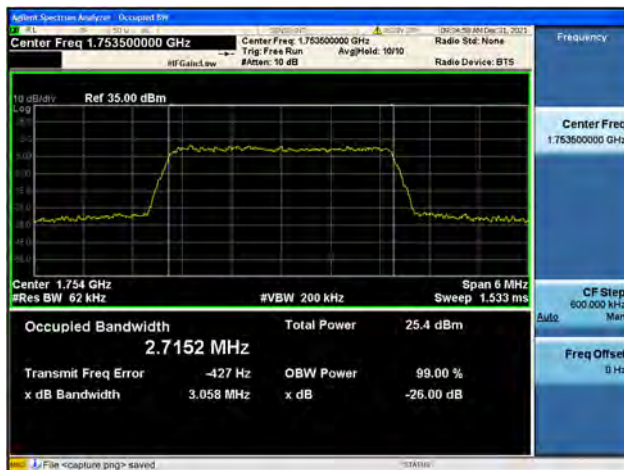
Band4 / 3MHz / High CH / 16QAM
