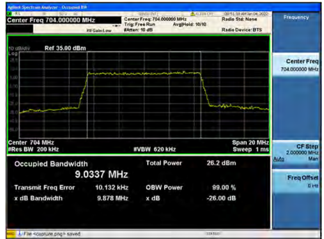
Band12 / 10MHz / Low CH / 64QAM
