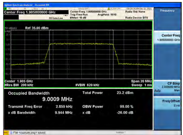
Band2 / 10MHz / High CH / 64QAM
