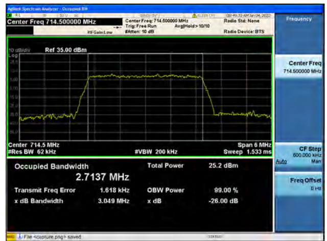
Band12 / 3MHz / High CH / 64QAM
