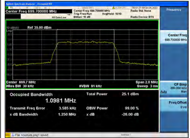
Band12 / 1.4MHz / Mid CH / QPSK
