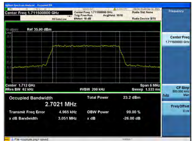
Band4 / 3MHz / Low CH / 64QAM
