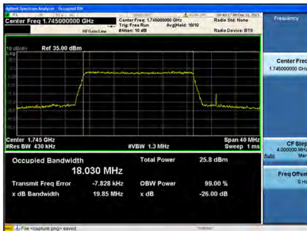
Band4 / 20MHz / High CH / 16QAM
