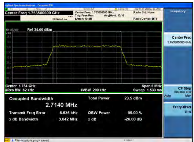
Band4 / 3MHz / High CH / 64QAM
