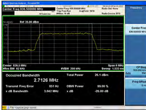
Band5 / 3MHz / Mid CH / 64QAM
