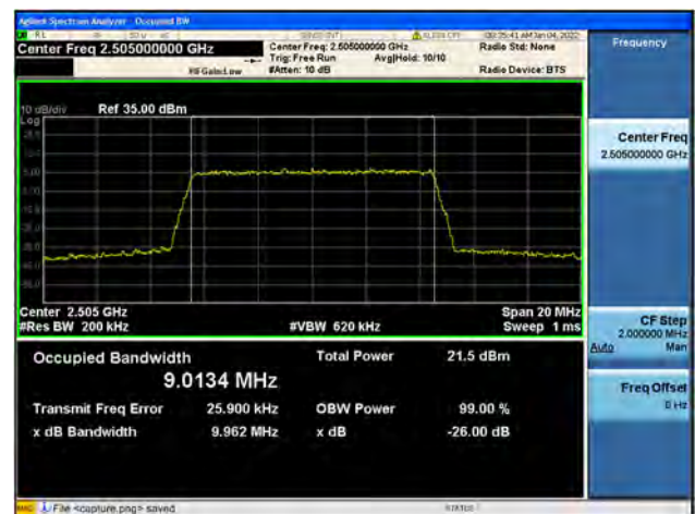
Band7 / 10MHz / Low CH / 64QAM
