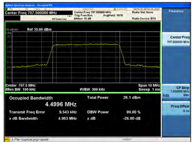
Band12 / 5MHz / Mid CH / 64QAM
