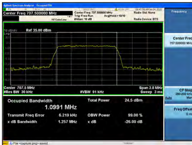
Band12 / 1.4MHz / Mid CH / 16QAM
