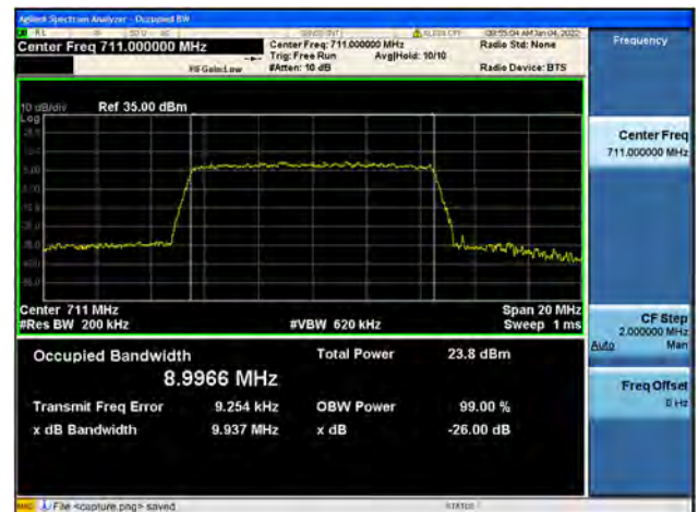
Band17 / 10MHz / High CH / 64QAM
