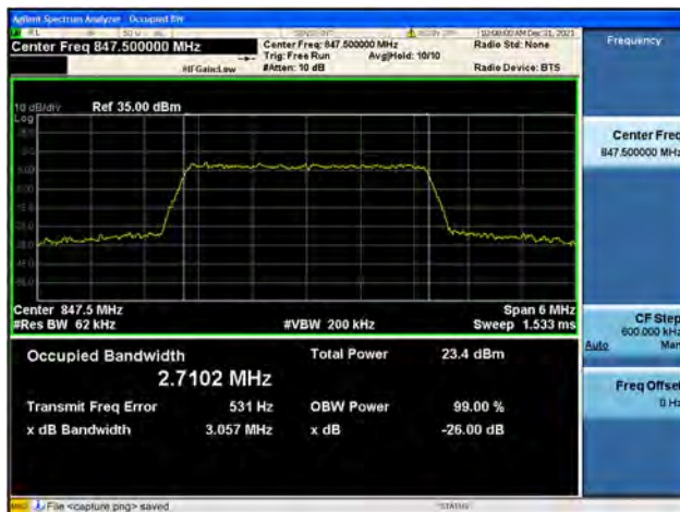
Band26 / 3MHz / High CH / 16QAM
