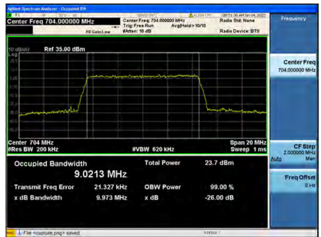
Band12 / 10MHz / Low CH / 64QAM
