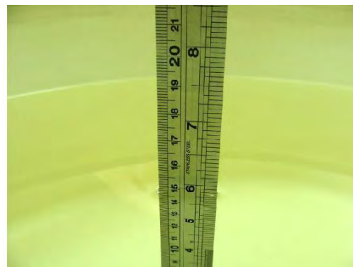
Fig 7.2 Photo of Liquid Height for Body SAR
