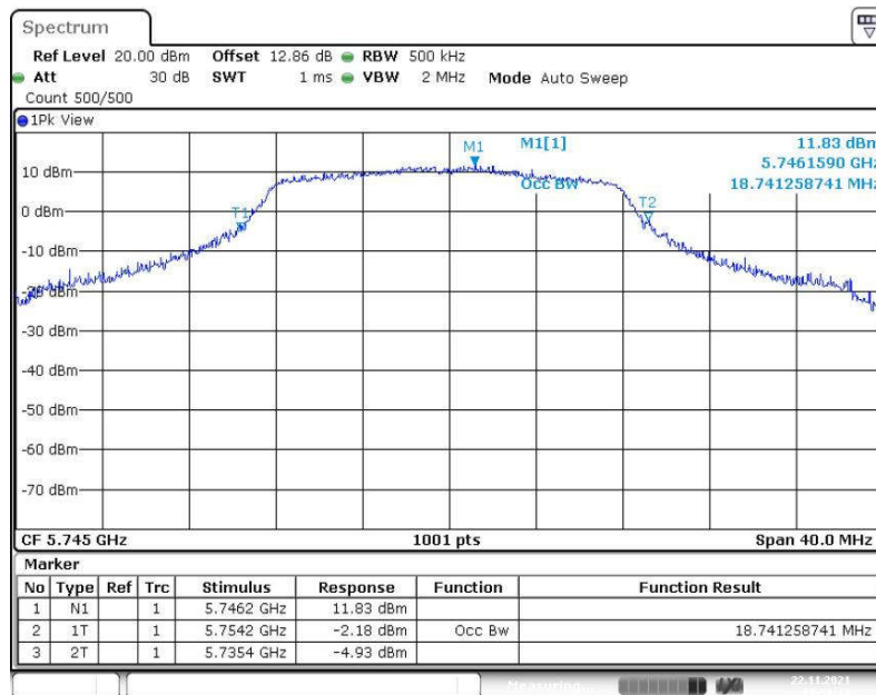
Fig. 42 99% Occupied Bandwidth (802.11a, 5745MHz)
