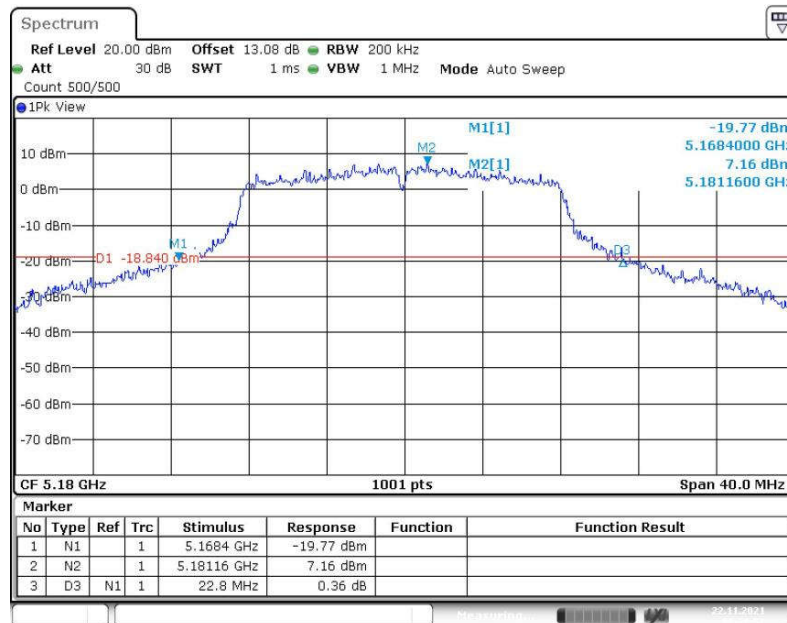
Fig. 1 Occupied 26dB Bandwidth (802.11a, 5180MHz)
