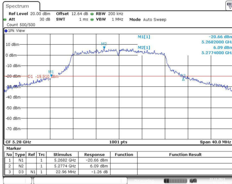
Fig. 5 Occupied 26dB Bandwidth (802.11a, 5280MHz)
