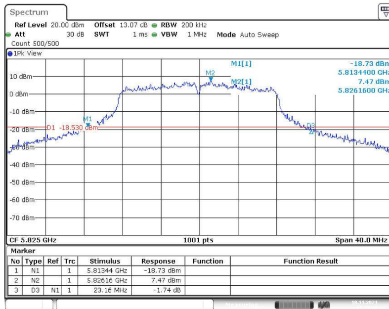
Fig. 12 Occupied 26dB Bandwidth (802.11a, 5825MHz)
