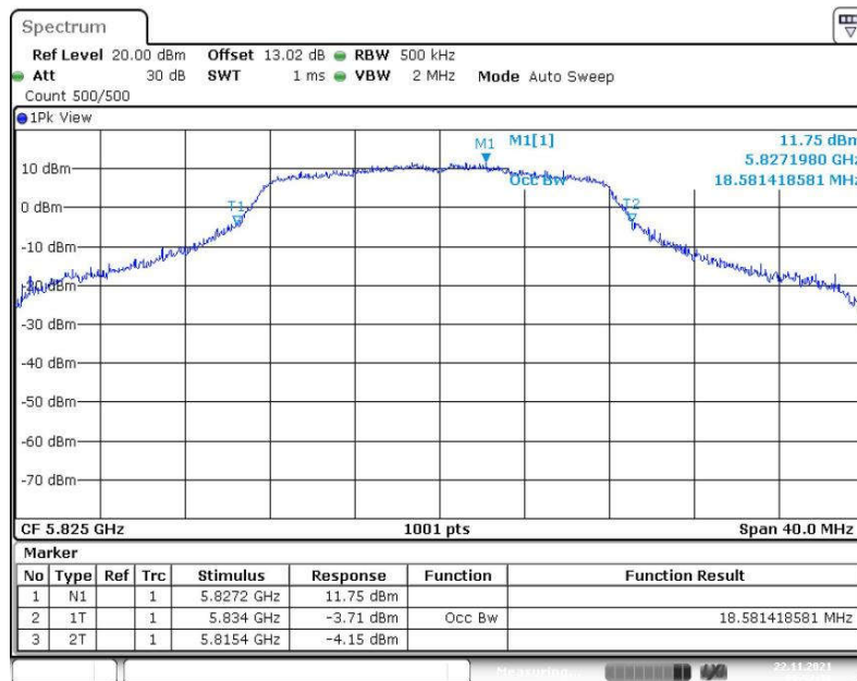
Fig. 44 99% Occupied Bandwidth (802.11a, 5825MHz)
