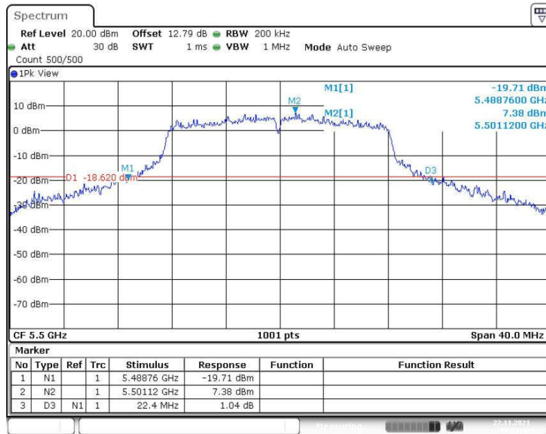
Fig. 7 Occupied 26dB Bandwidth (802.11a, 5500MHz)
