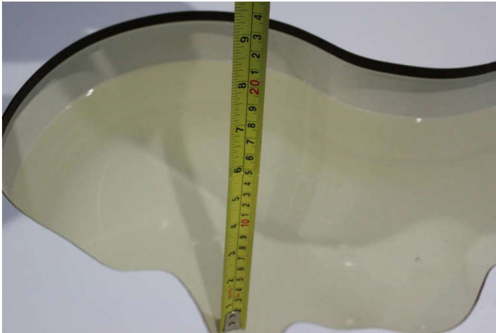
Picture 7-7: Liquid depth in the Head Phantom(5GHz)
