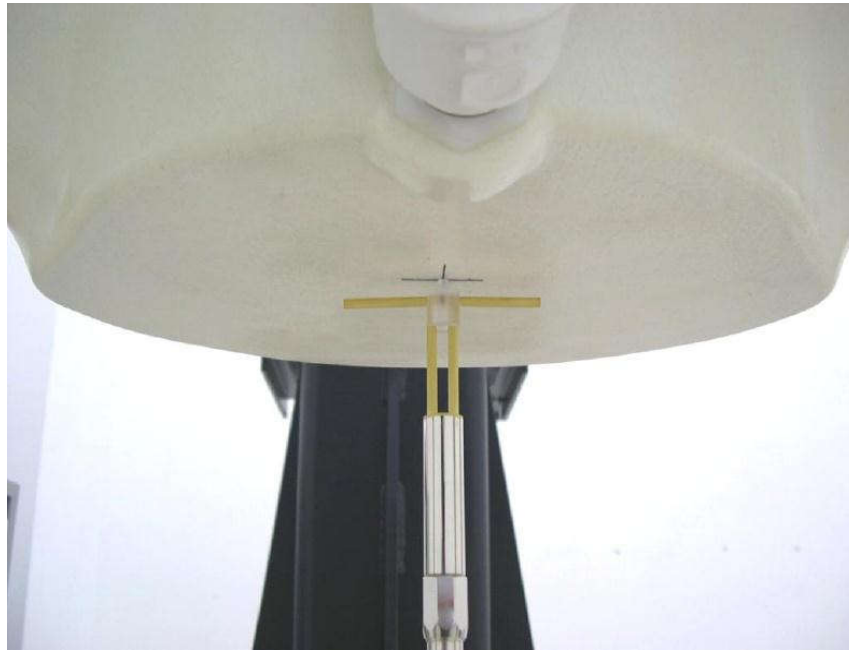
Picture 8.2 Photo of Dipole Setup
