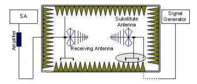
In the chamber, an substitution antenna for the frequency band of interest is placed at the ©Copyright. All rights reserved by SAICT. Page 16 of 108
