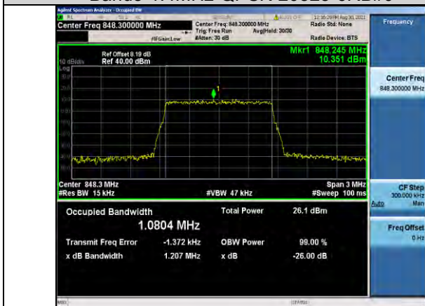
Band5-1.4MHz-QPSK-20643-6RB#0
