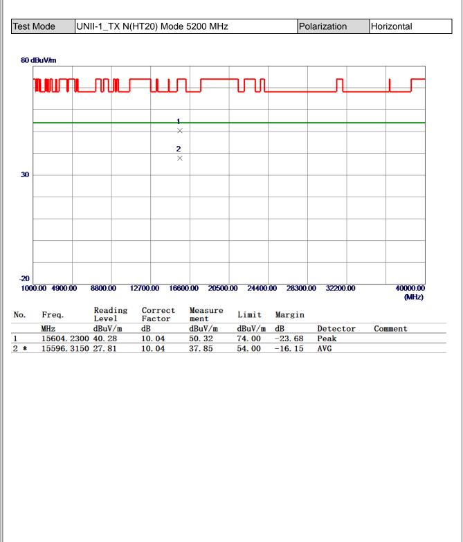
(1) Measurement Value = Reading Level + Correct Factor.
