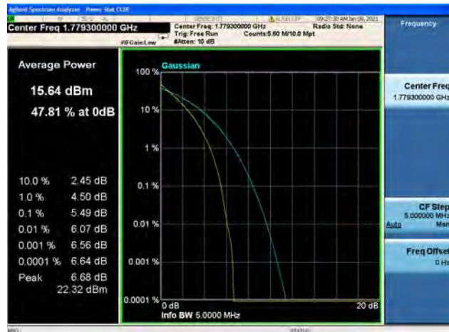
Band66 / 1.4MHz / High CH / 64QAM
