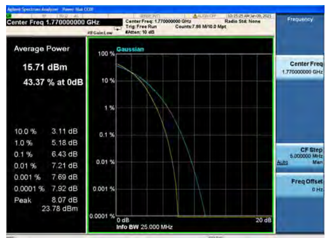
Band66 / 20MHz / High CH / 64QAM
