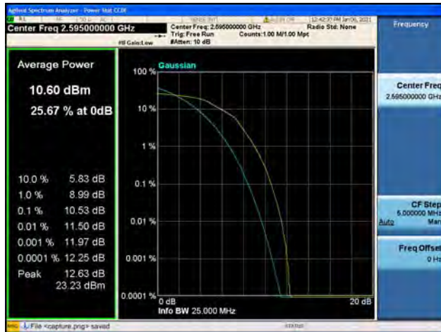
Band38 / 20MHz / High CH / 16QAM
