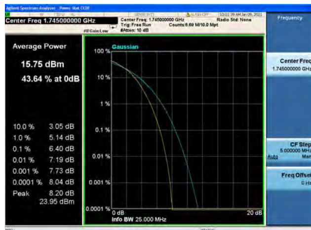
Band66 / 20MHz / High CH / 16QAM
