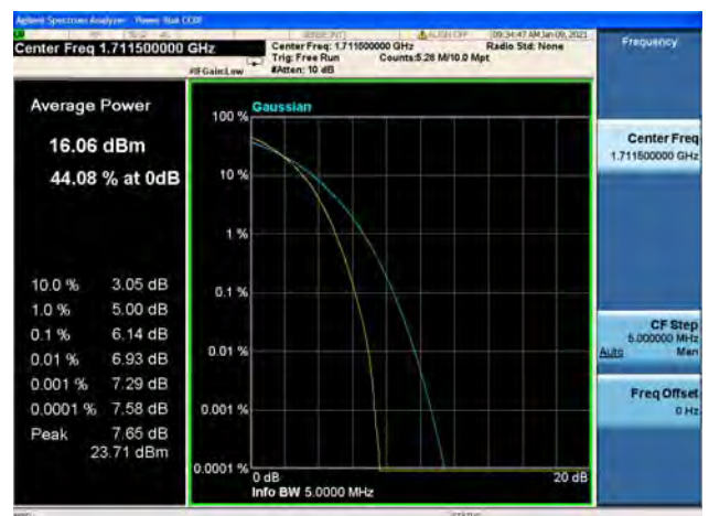
Band66 / 3MHz / Low CH / 64QAM
