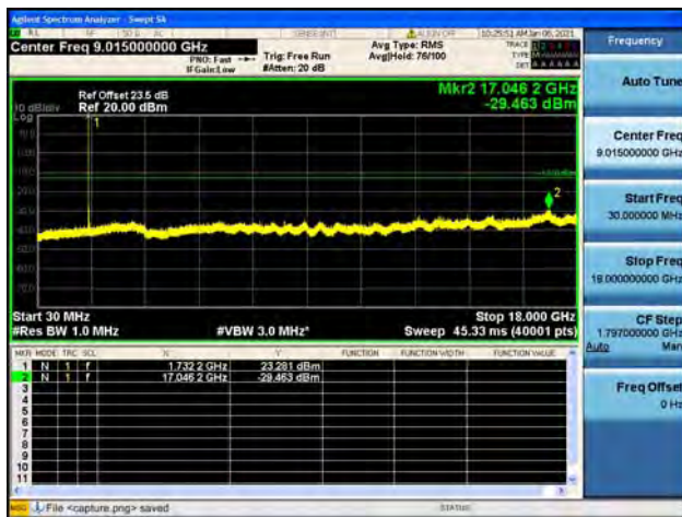
Band4 / 1.4MHz / Mid CH / 16QAM
