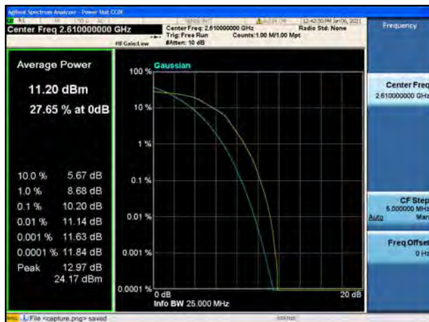
Band38 / 20MHz / High CH / 16QAM
