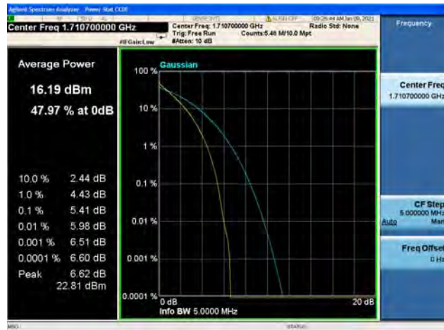
Band66 / 1.4MHz / Low CH / 64QAM
