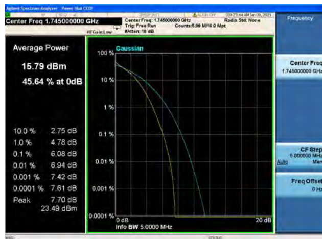
Band66 / 1.4MHz / Mid CH / 16QAM
