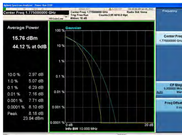
Band66 / 10MHz / High CH / 16QAM
