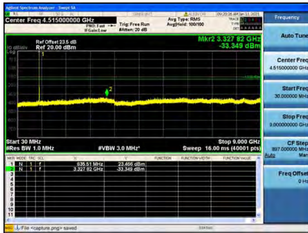
Band5 / 3MHz / Mid CH / 64QAM
