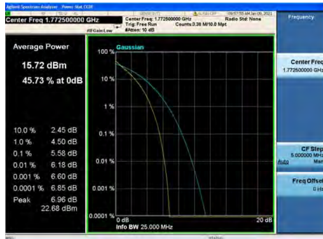
Band66 / 15MHz / High CH / 64QAM
