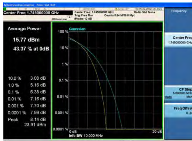
Band66 / 10MHz / High CH / 16QAM
