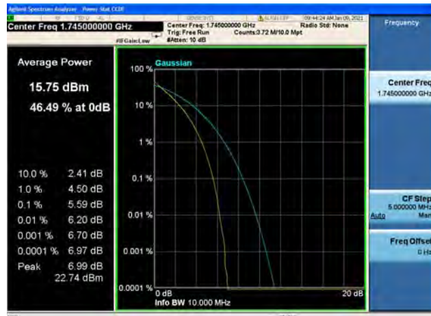
Band66 / 10MHz / Mid CH / 64QAM
