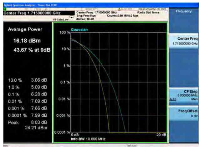
Band66 / 10MHz / Low CH / 64QAM
