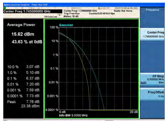
Band66 / 5MHz / Mid CH / 64QAM
