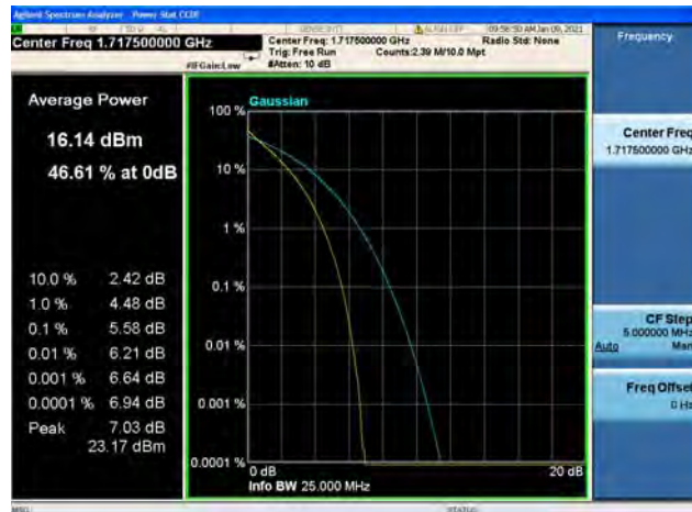
Band66 / 15MHz / Low CH / 64QAM
