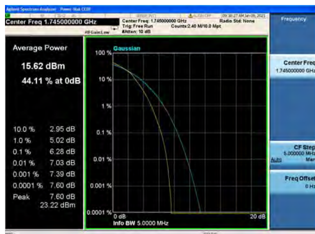
Band66 / 5MHz / Mid CH / 16QAM
