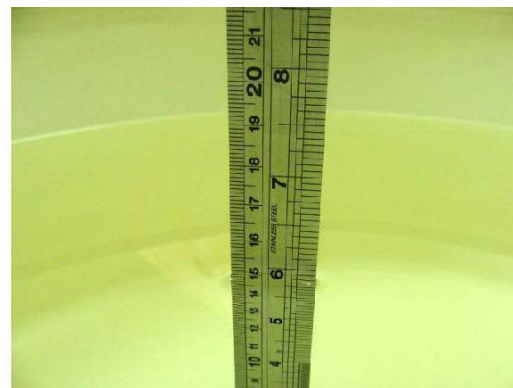
Fig 7.2 Photo of Liquid Height for Body SAR
