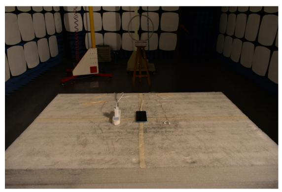
3. Radiated emission (9KHz-30MHz)
