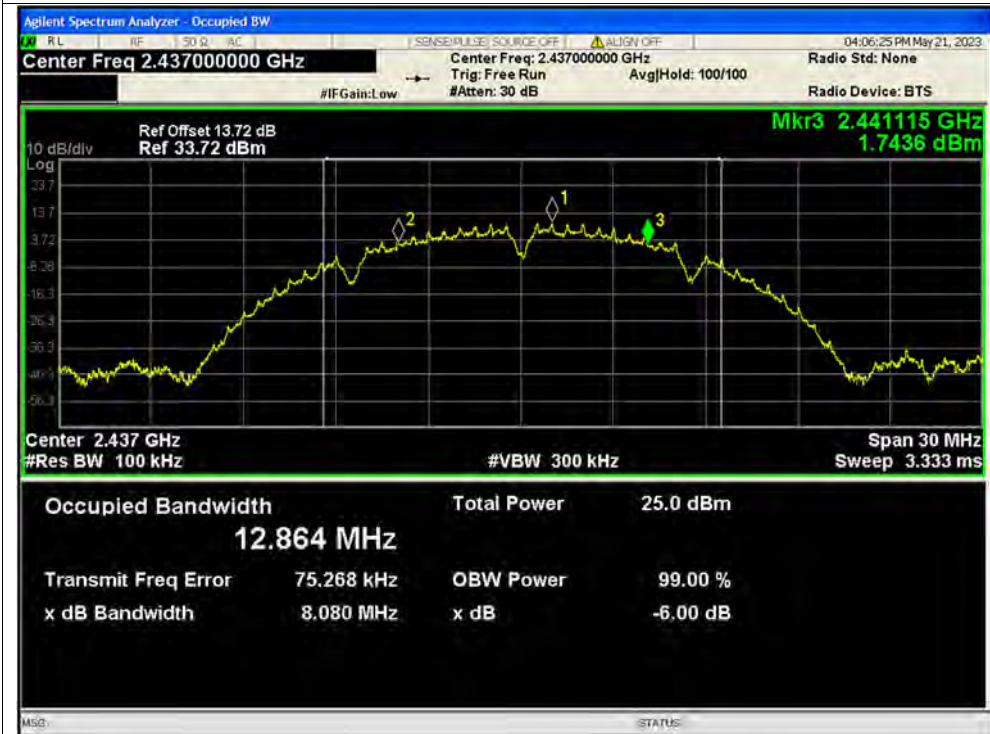
-6dB Bandwidth NVNT b 2437MHz Ant1
