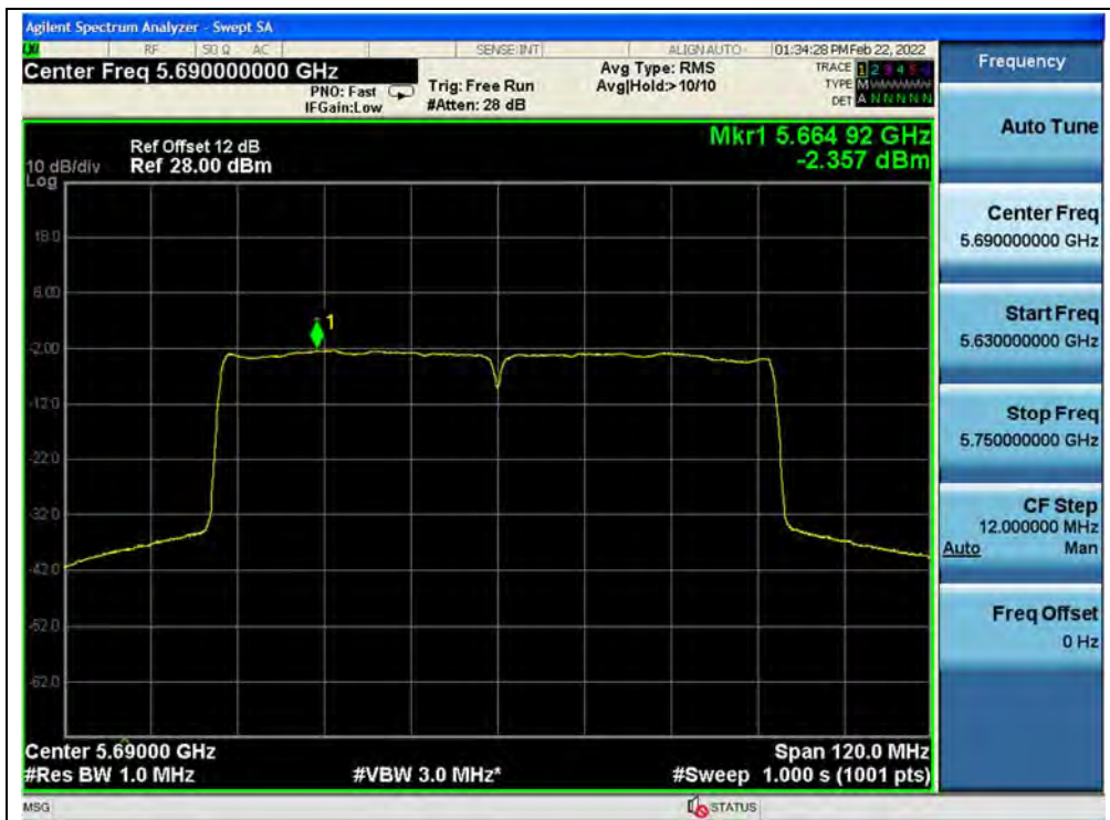
(Channel 138, 5690MHz, 802.11ac (VHT80))
