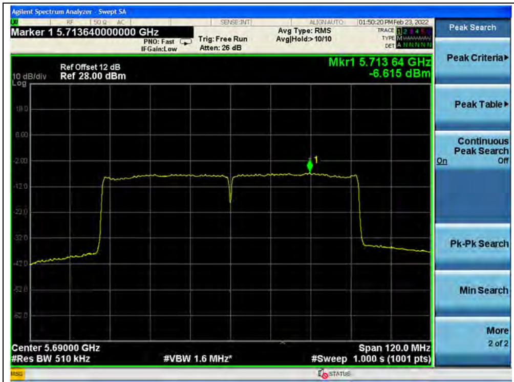
(Channel 138, 5690MHz, 802.11ac (VHT80))
