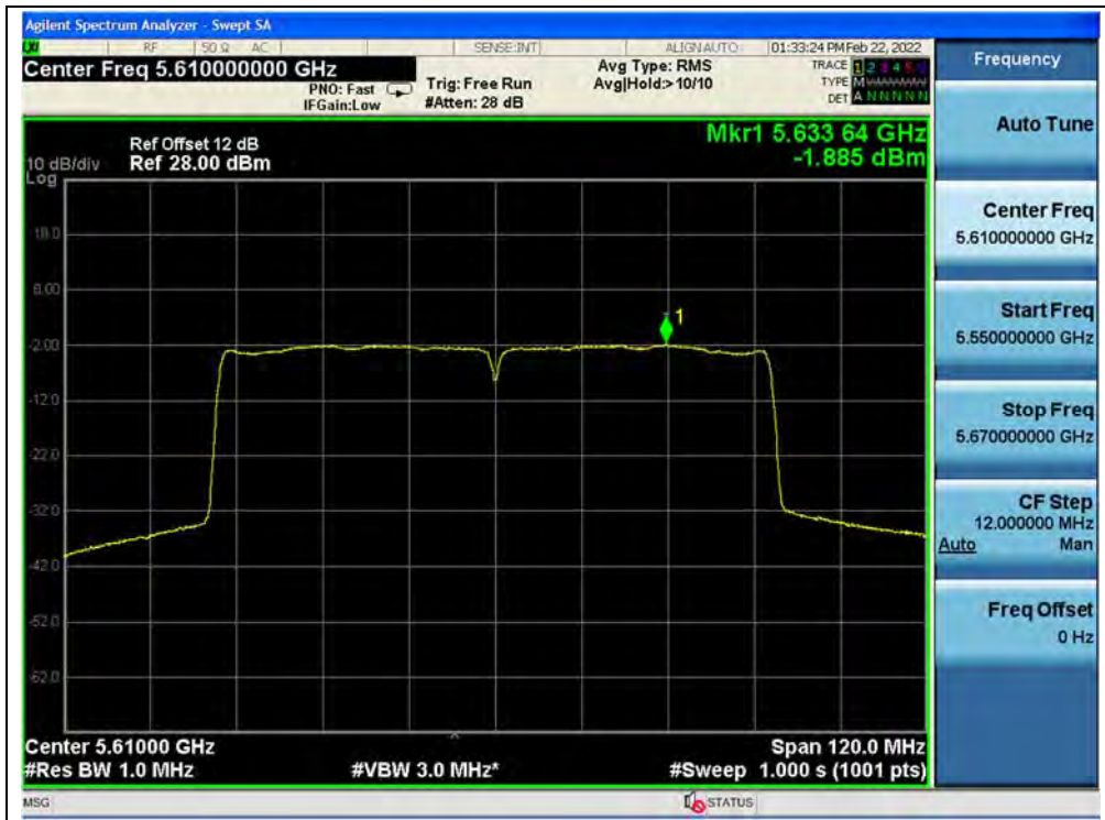
(Channel 122, 5610MHz, 802.11ac (VHT80))
