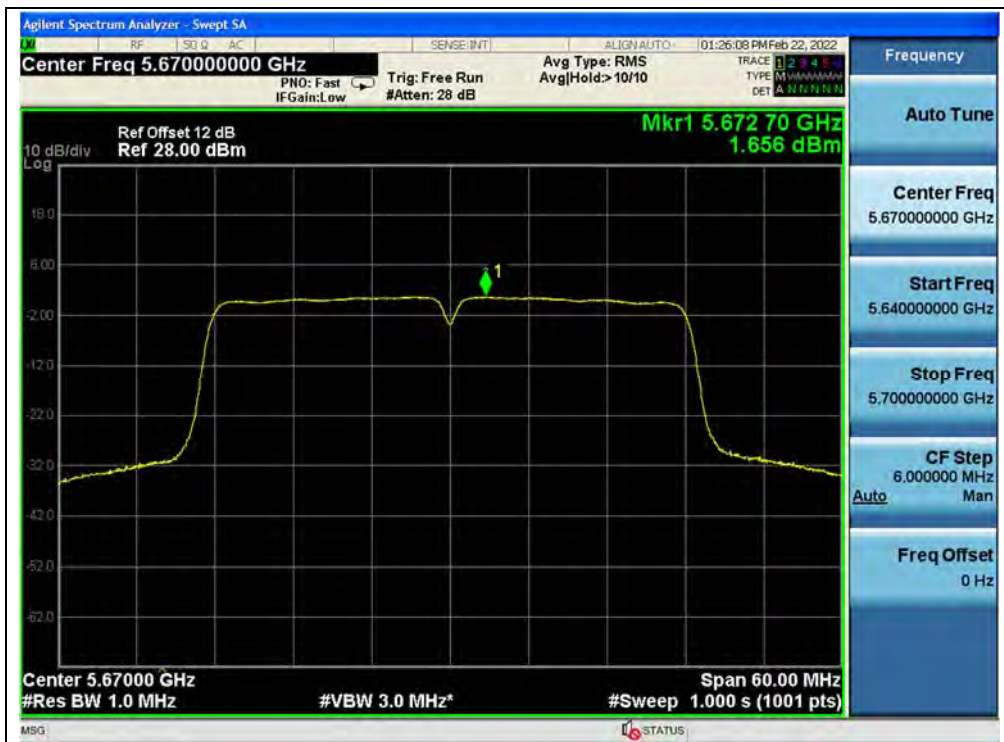
(Channel 134, 5670MHz, 802.11ac (VHT40))
