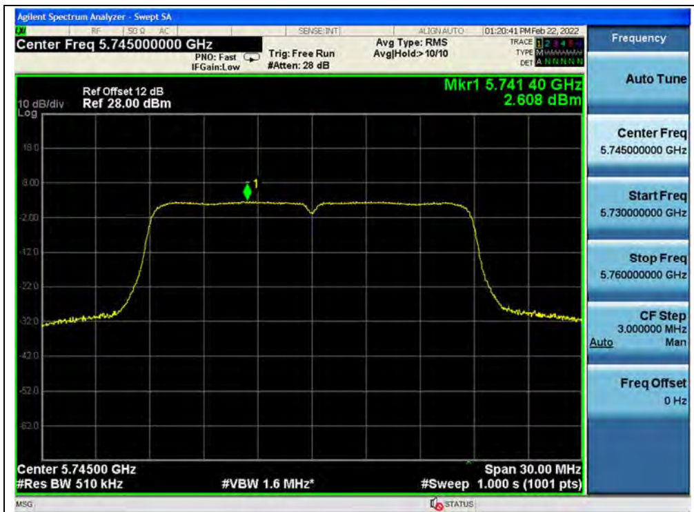
(Channel 149, 5745MHz, 802.11ac (VHT20))
