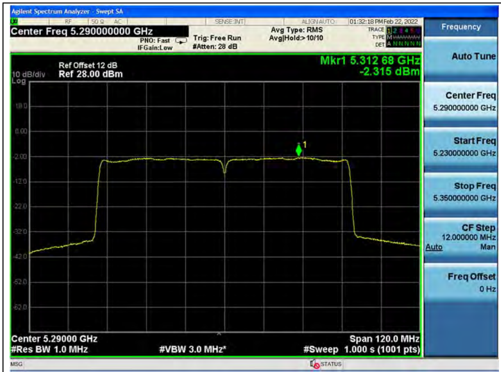
(Channel 58, 5290MHz, 802.11ac (VHT80))
