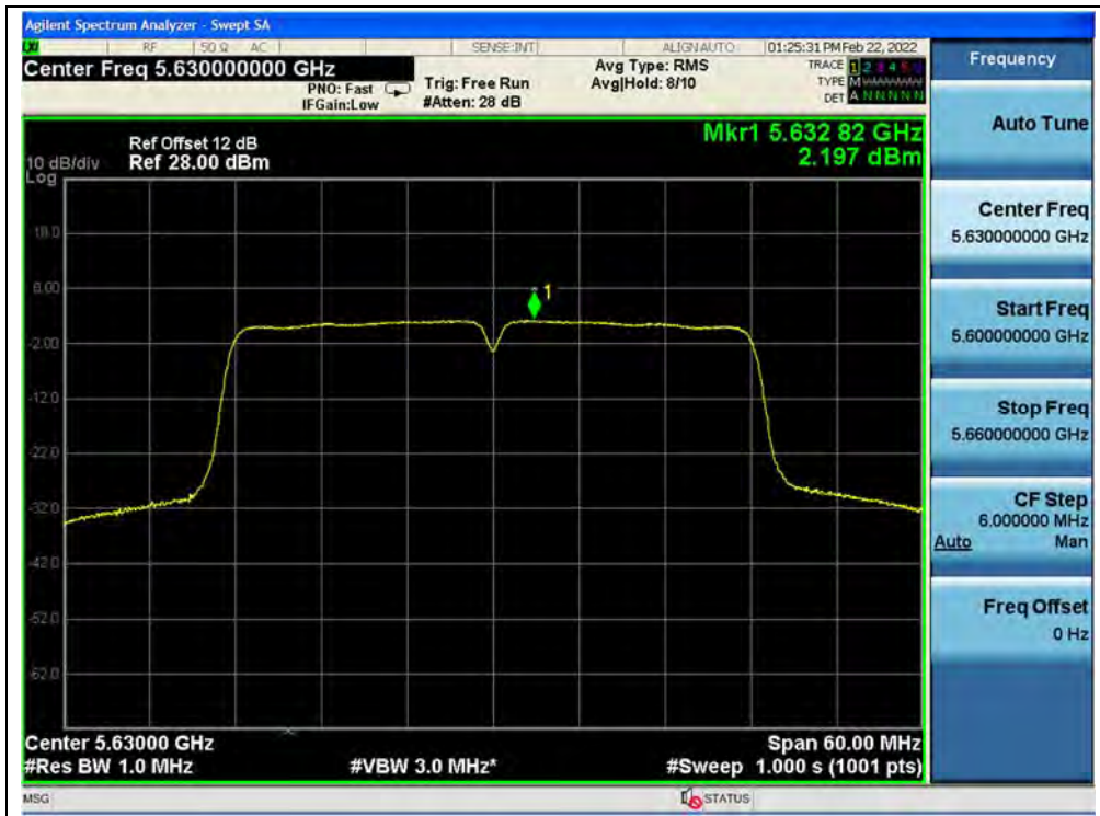
(Channel 126, 5630MHz, 802.11ac (VHT40))
