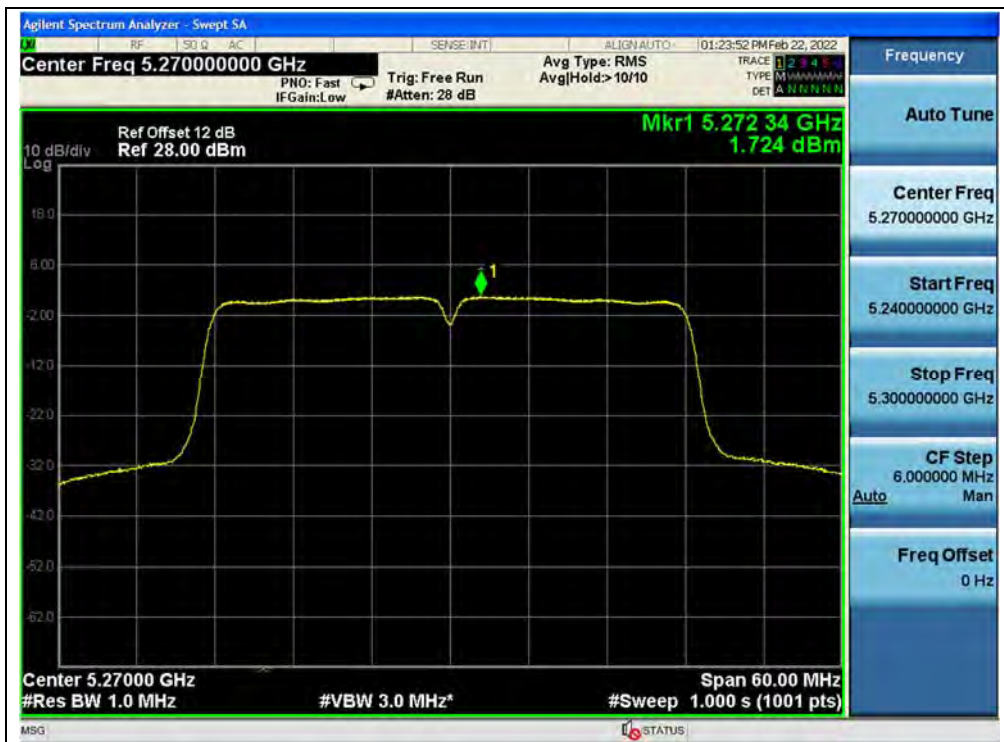
(Channel 54, 5270MHz, 802.11ac (VHT40))
