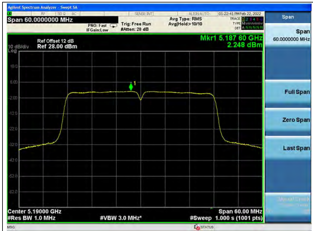
(Channel 38, 5190MHz, 802.11ac (VHT40))
