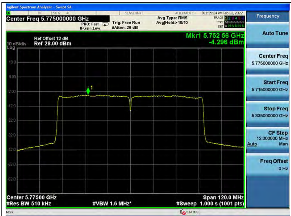
(Channel 155, 5775MHz, 802.11ac (VHT80))
