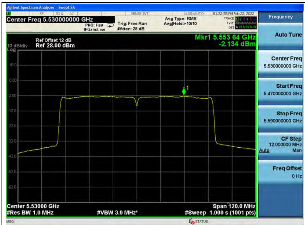
(Channel 106, 5530MHz, 802.11ac (VHT80))
