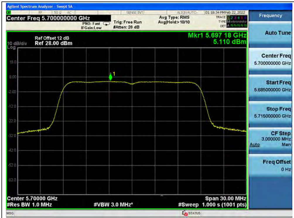
(Channel 140, 5700MHz, 802.11ac (VHT20))
