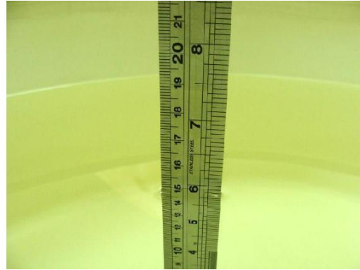
Fig 7.2 Photo of Liquid Height for Body SAR
