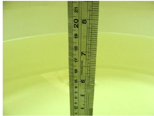
Fig 7.2 Photo of Liquid Height for Body SAR
