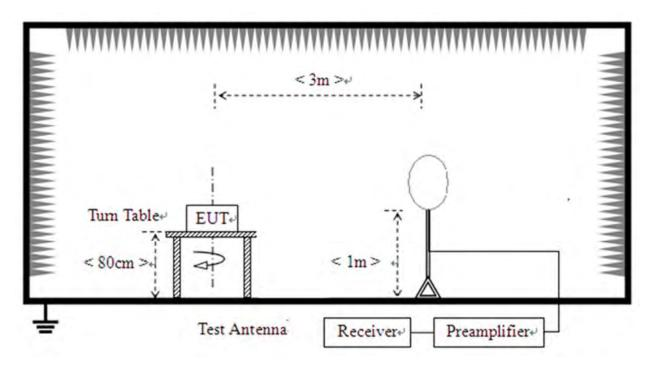
2) For radiated emissions from 30MHz to1GHz
