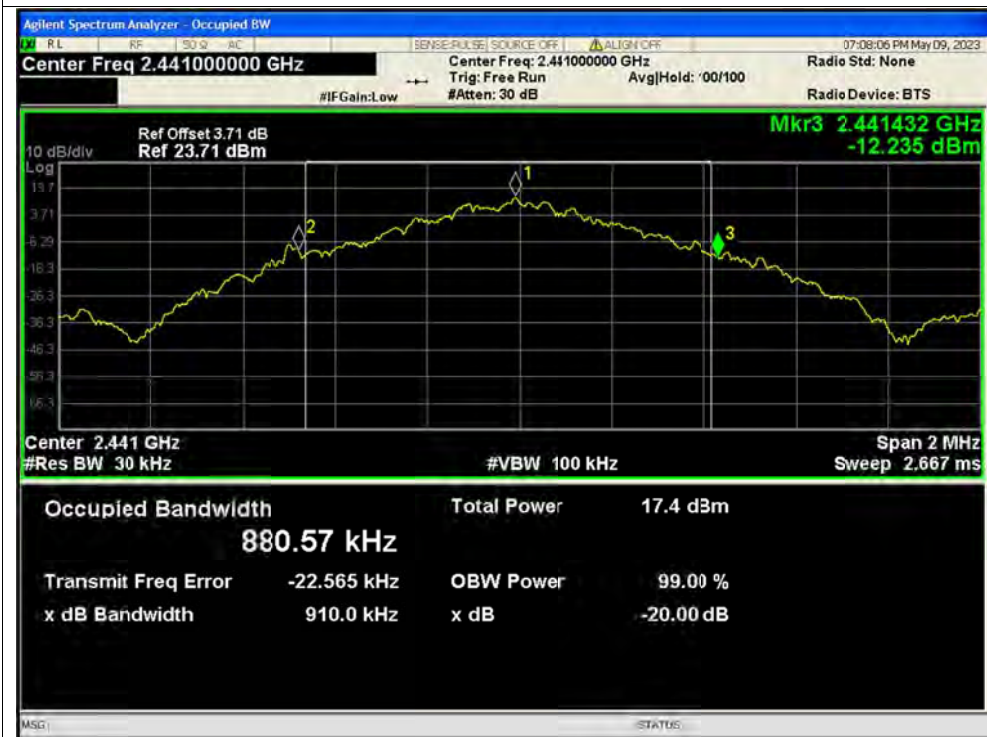
-20dB Bandwidth NVNT 1-DH5 2441MHz Ant1
