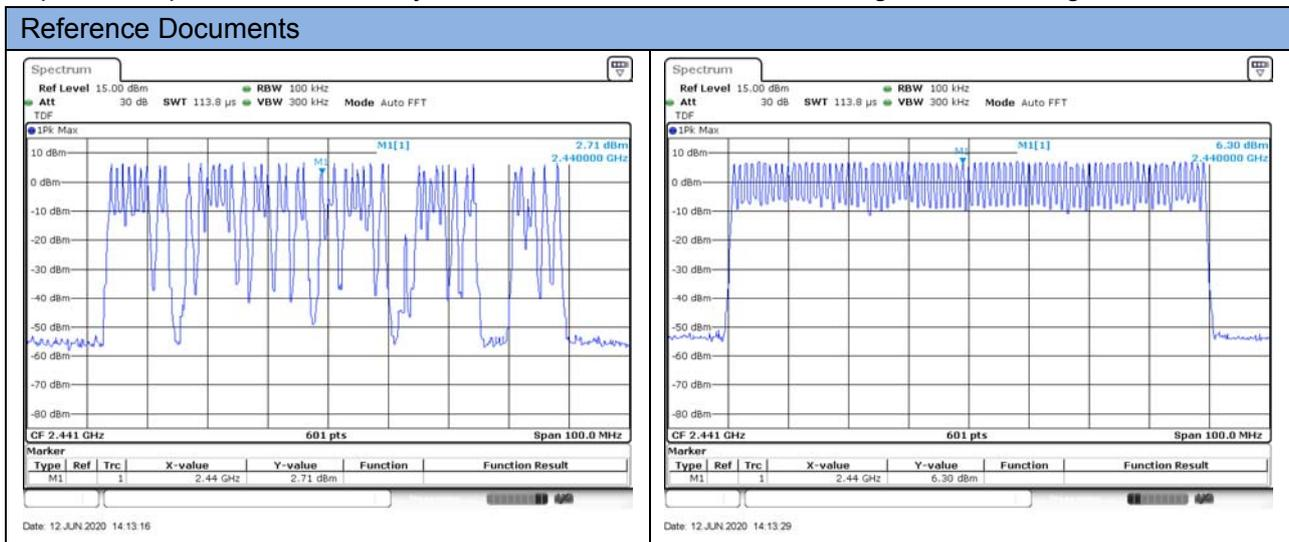
3. Channels are classified into two categories, used and unused, where used channels are part of the hopping sequence and unused channels are replaced in the hopping sequence by used channels in a pseudo-random way. Make each individual EUT meets the requirement that each of its hopping channels is used equally on average.
