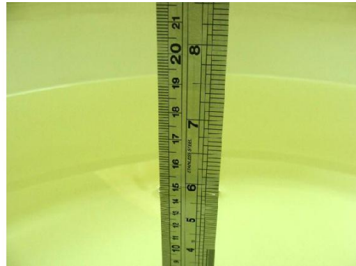
Fig 7.2 Photo of Liquid Height for Body SAR
