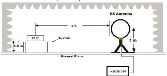
(2) Radiated Emission Test-Up Frequency 30MHz~1GHz
