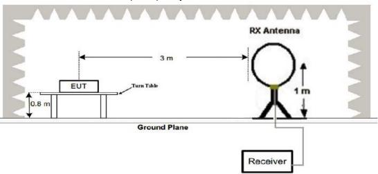
(2) Radiated Emission Test-Up Frequency 30MHz~1GHz
