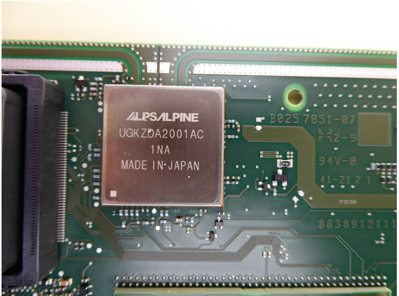
WLAN module – close-up
