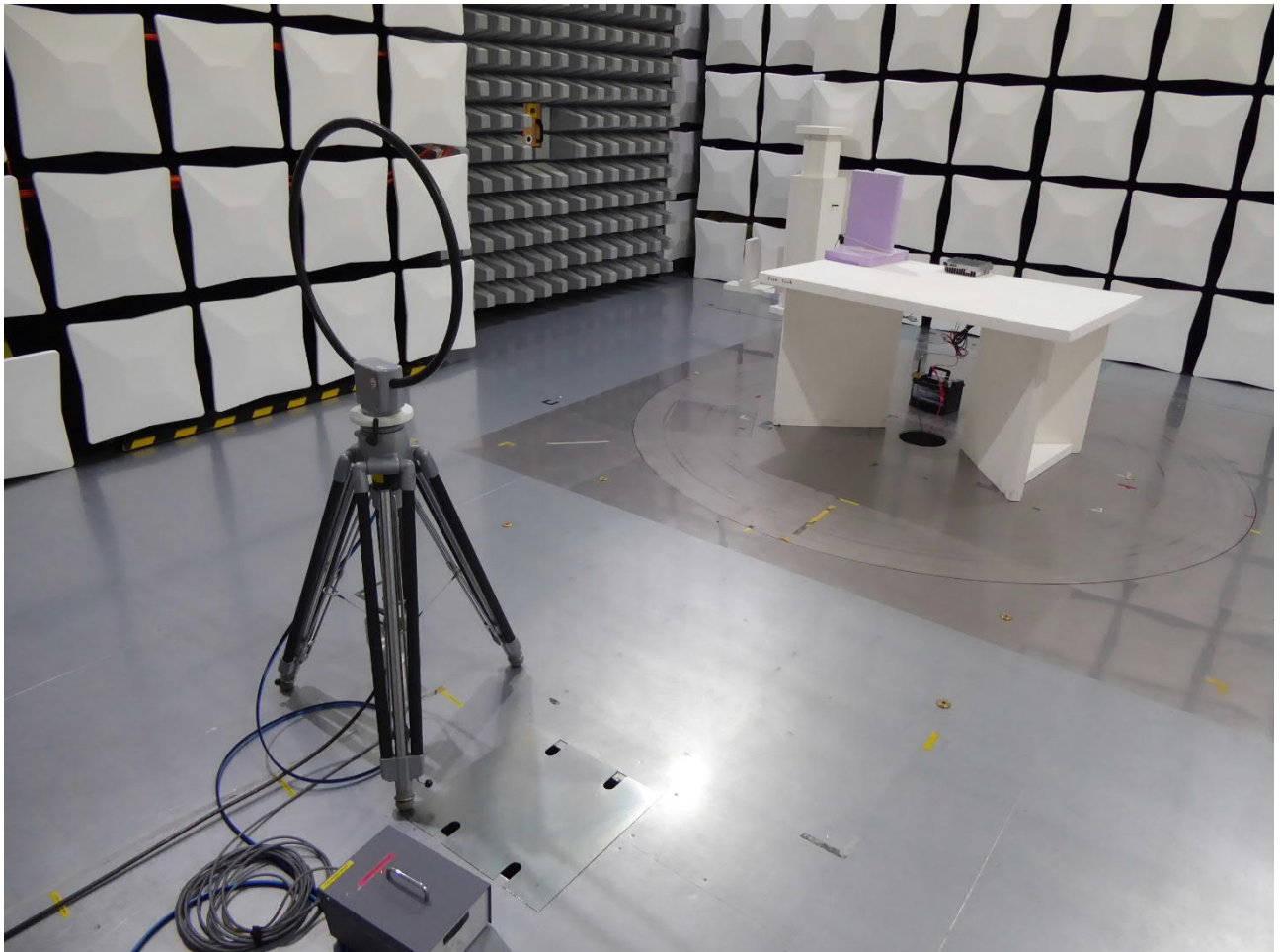
Test setup semi anechoic chamber (9 kHz – 30 MHz)
