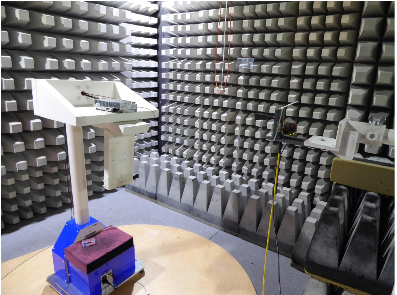
Test setup fully anechoic chamber (26.5 - 40 GHz)
