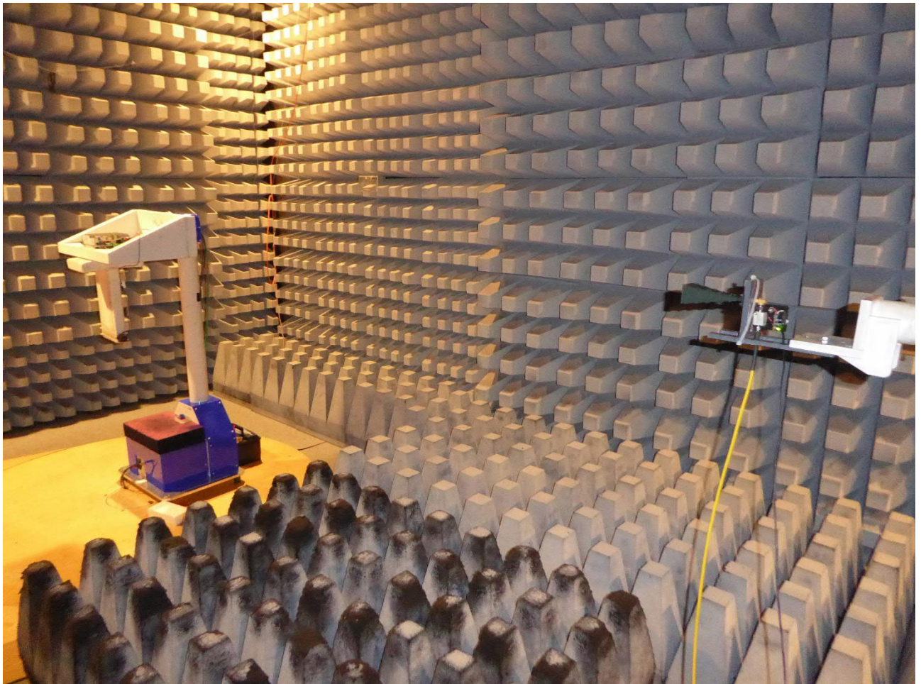
Test setup fully anechoic chamber (18 – 26.5 GHz)
