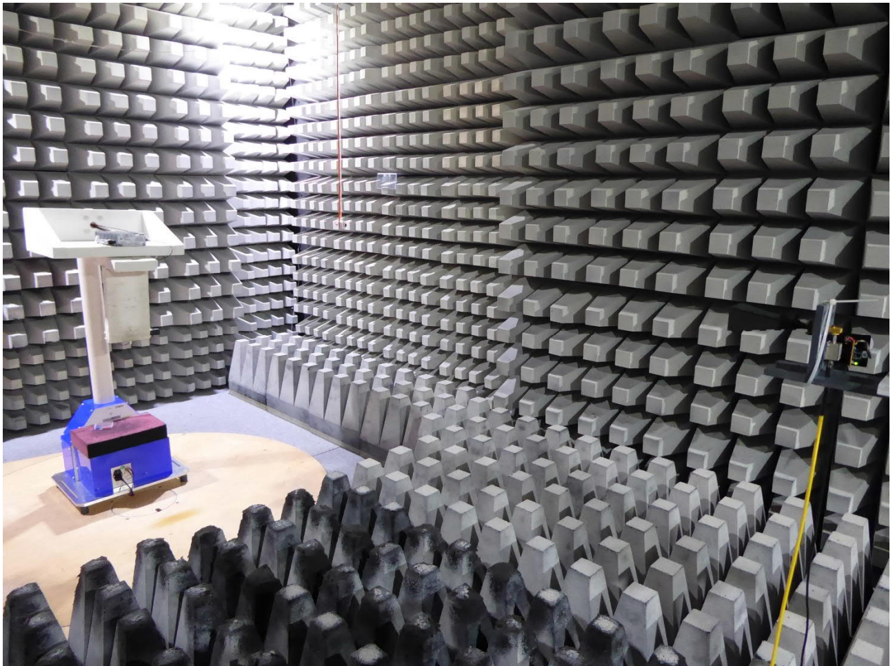
Test setup fully anechoic chamber (18 – 26.5 GHz)
