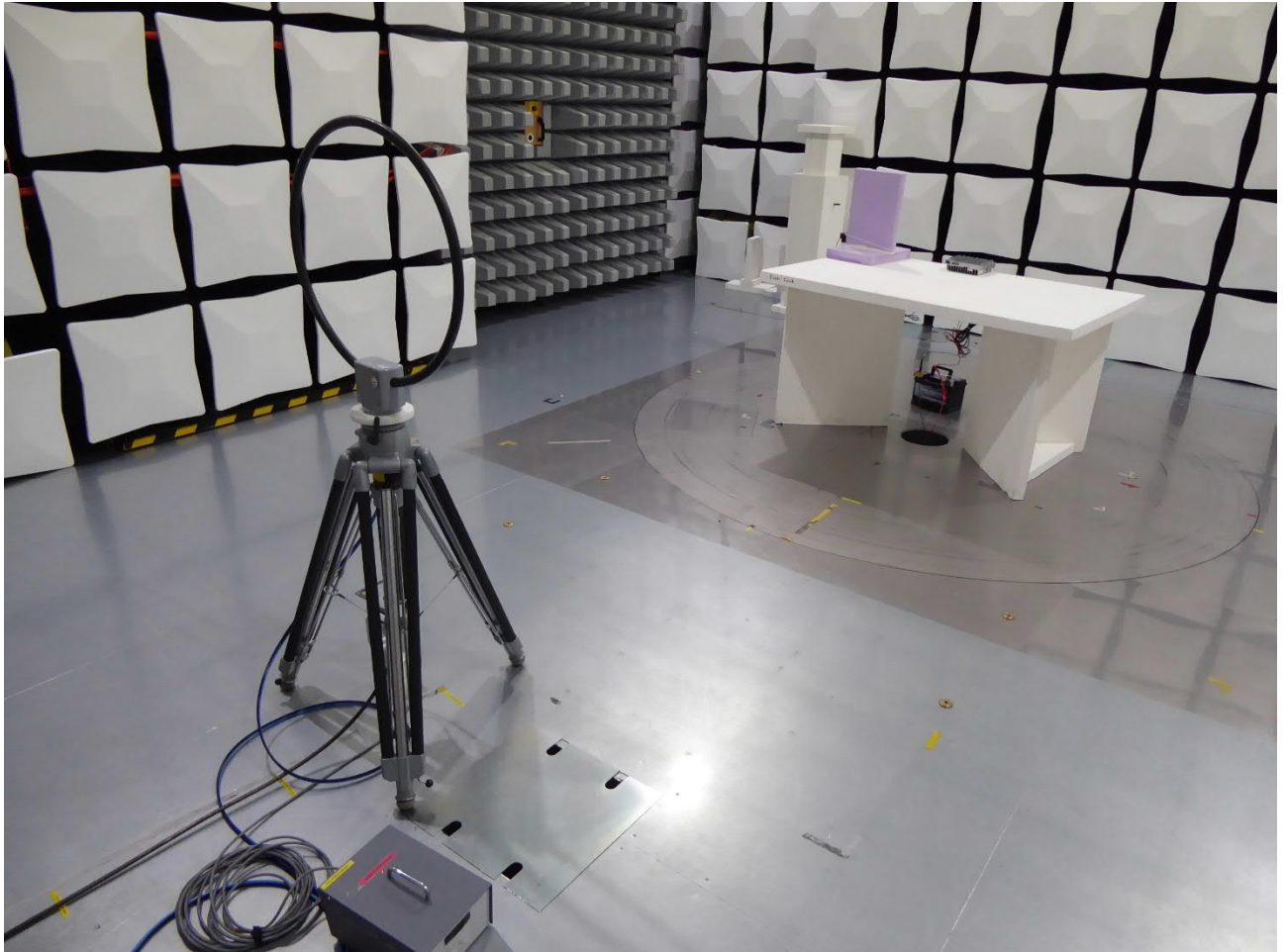
Test setup semi anechoic chamber (9 kHz – 30 MHz)
