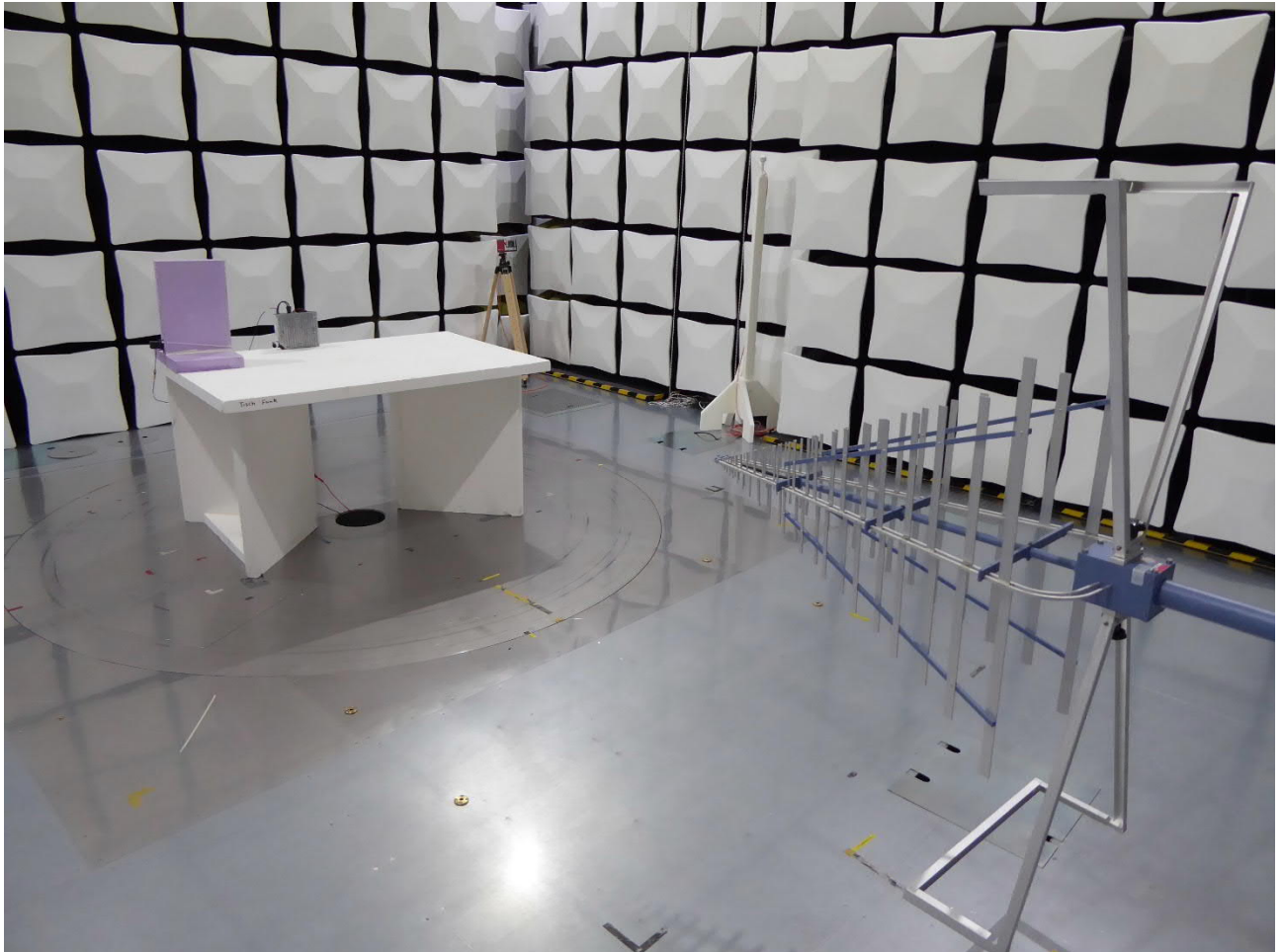
Test setup semi anechoic chamber (30 MHz – 1 GHz)
