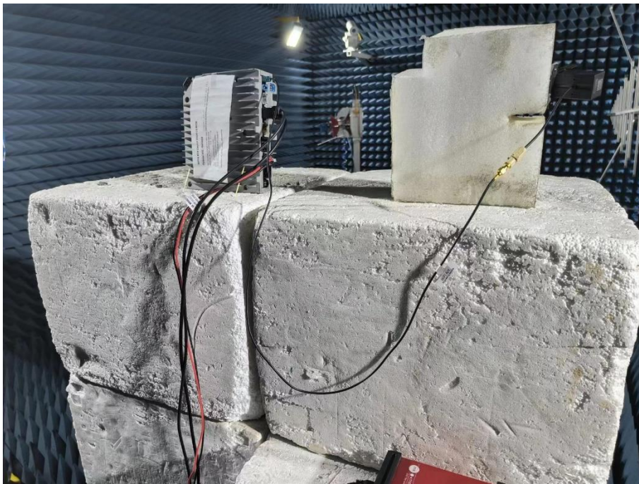
8. Radiated Emissions (Part 15C&Part 15E, 1GHz -18GHz, Pos 2)
