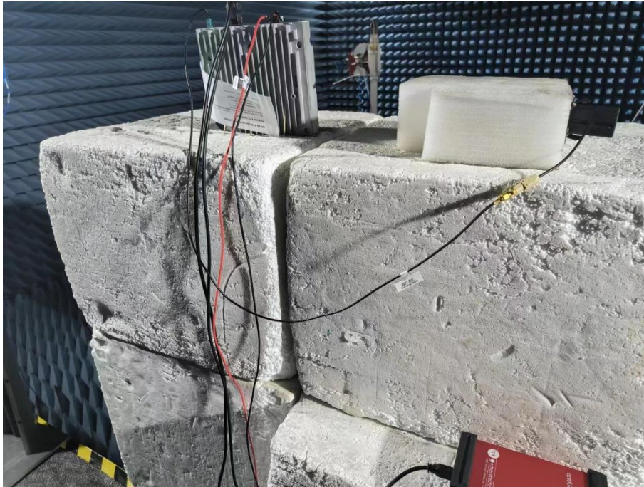
9. Radiated Emissions (Part 15C&Part 15E, 1GHz -18GHz, Pos 3)
