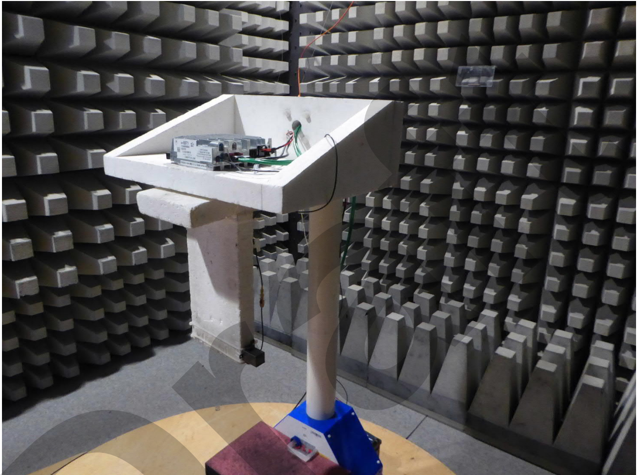
Test setup fully anechoic chamber
