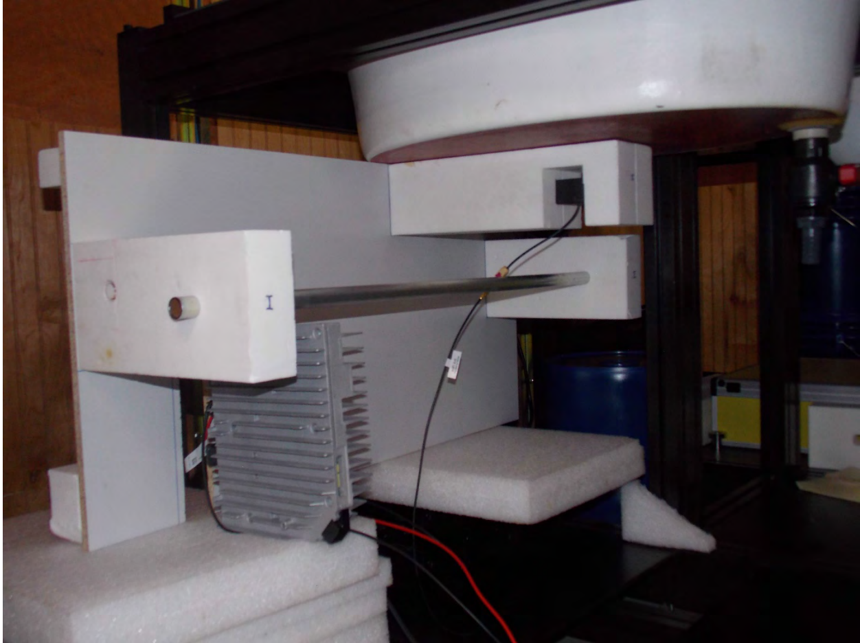
Back Test Position using Test Jig Supplied by Robert Bosch Front View
