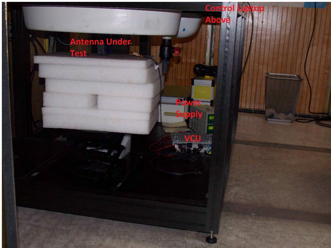
Photo of the Setup showing the VCU location during each test
