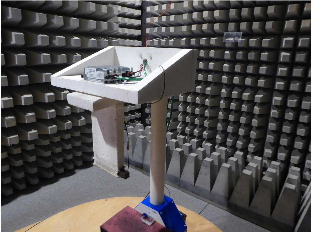
Test setup fully anechoic chamber
