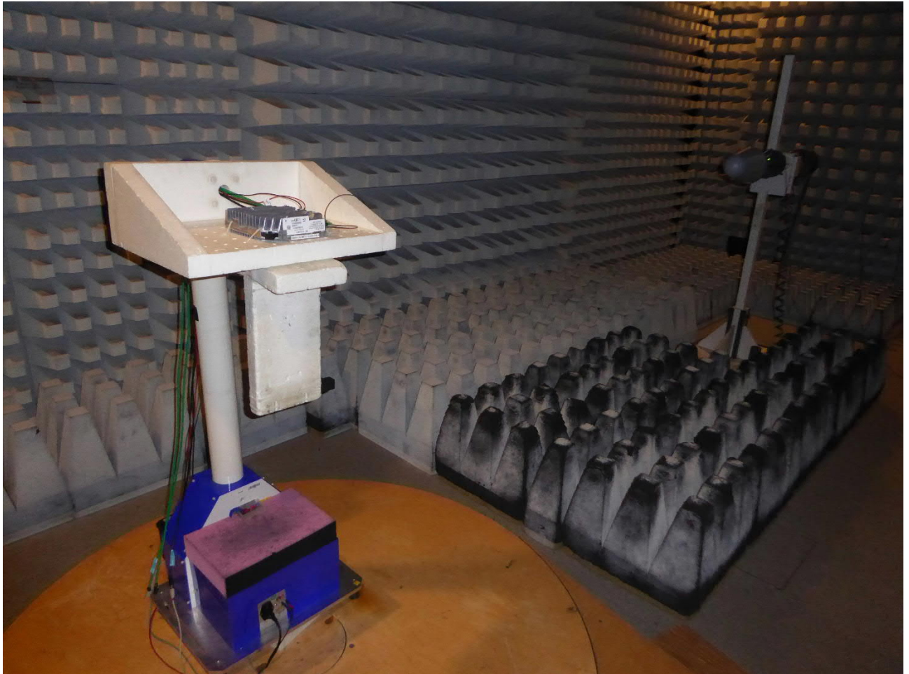
Test setup fully anechoic chamber (1 – 12 GHz)
