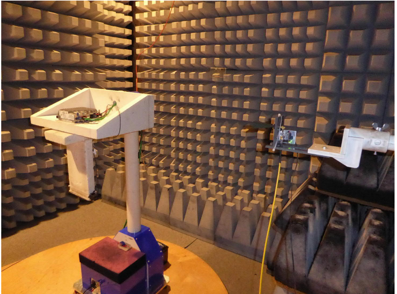
Test setup fully anechoic chamber (26.5 – 40 GHz)
