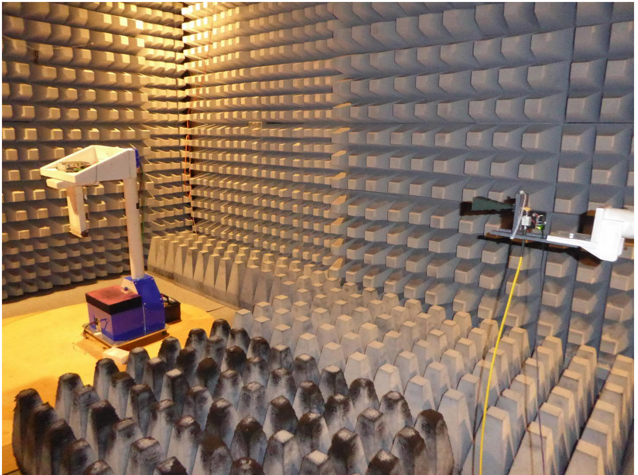
Test setup fully anechoic chamber (18 – 26.5 GHz)
