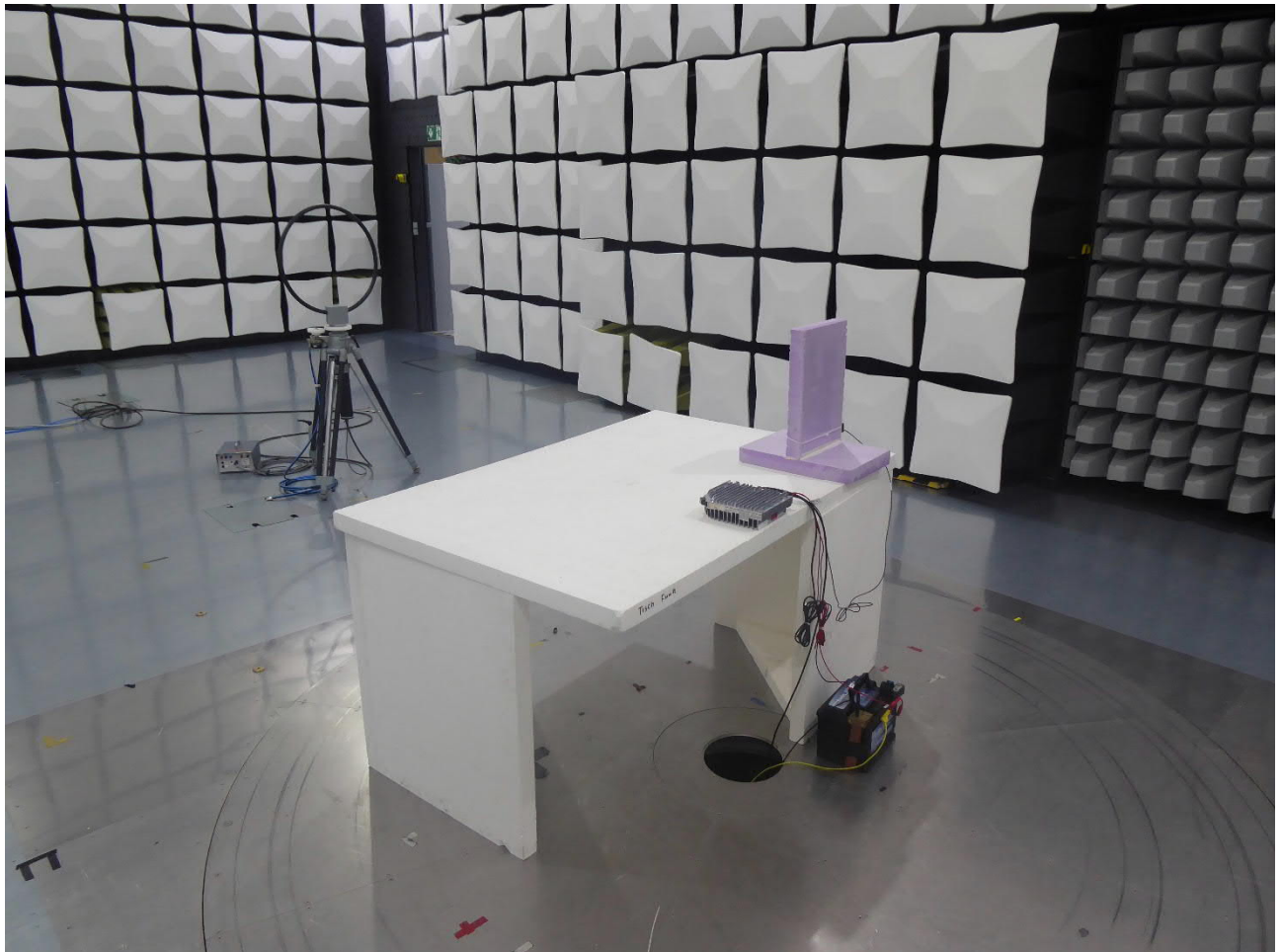
Test setup semi anechoic chamber (9 kHz – 30 MHz) – EUT Pos 1
