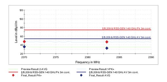
Only the worst-case emissions from the antenna port conducted pre-tests were repeated as radiated tests.
