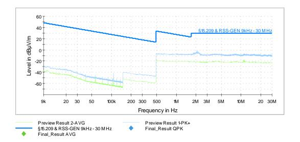
Remark: No emissions close than 20 dB to the limit, so no final measurement will be carried out.
