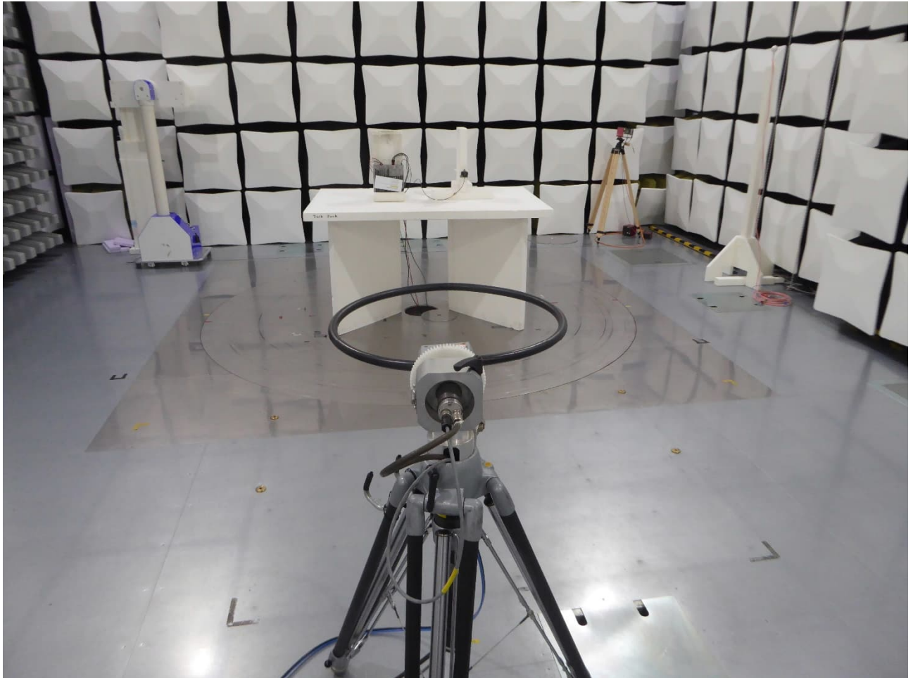
Test setup semi anechoic chamber (9 kHz – 30 MHz) Antenna Position 3 – ground parallel
