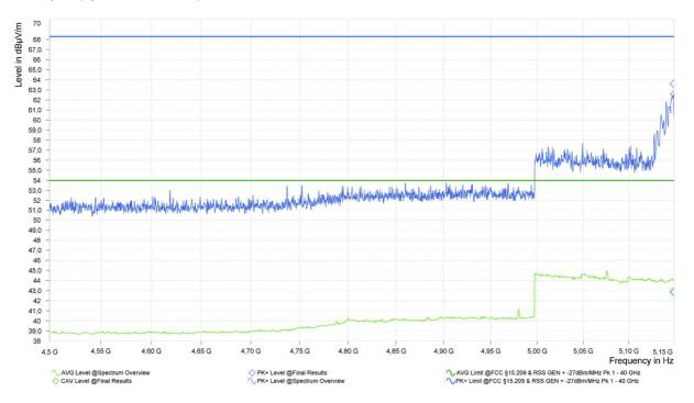
Only the worst-case emissions from the antenna port conducted pre-tests were repeated as radiated tests.
