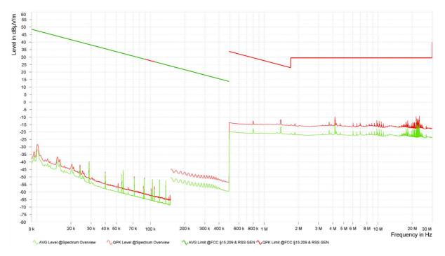
Spurious emissions from 9 kHz to 30 MHz (operation mode 9 - Pos 3):
