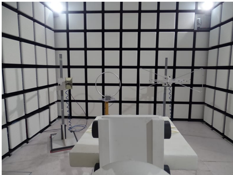
Photo 19: Gain tests with Puck antenna
