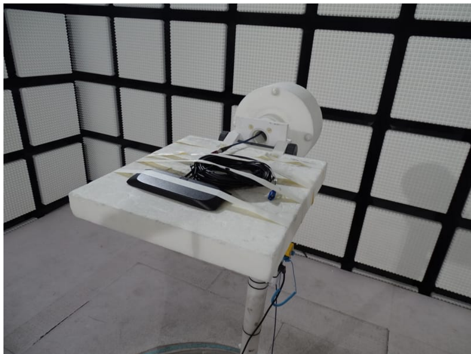
Photo 43: Gain tests with candybar antenna
