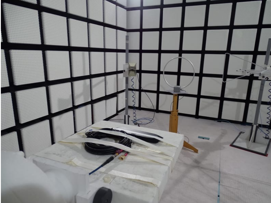
Photo 39: Gain tests with candybar antenna
