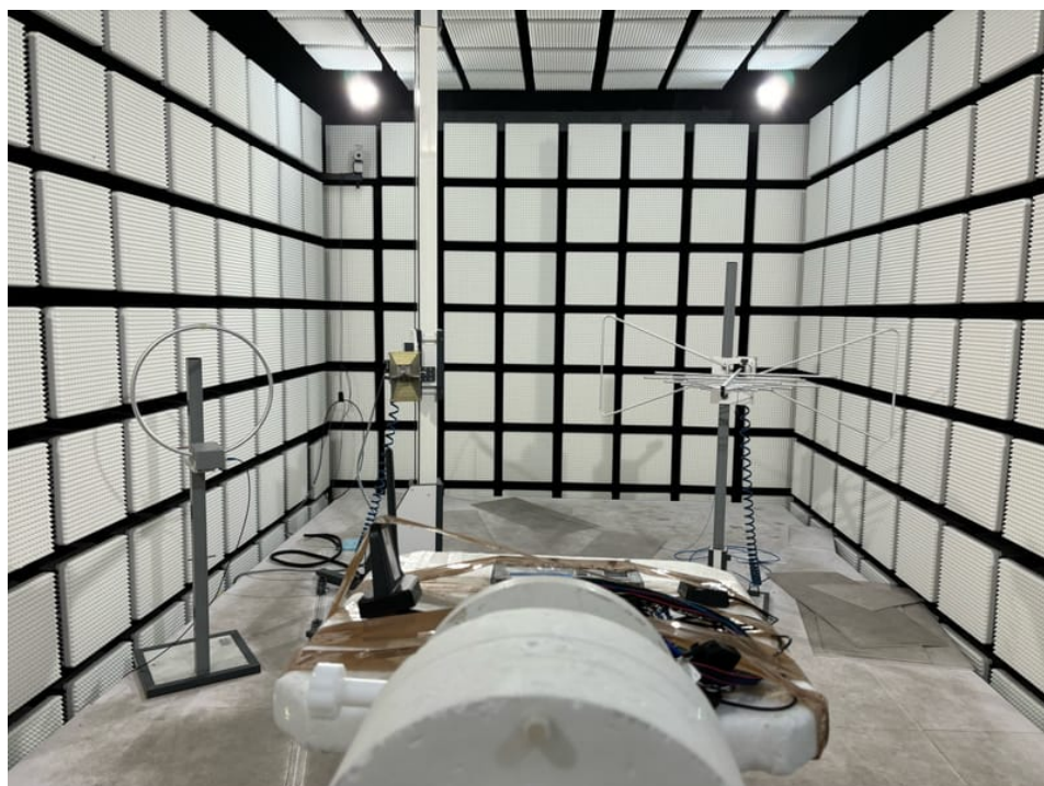
Photo 28: RSE tests with Supercombo antenna
