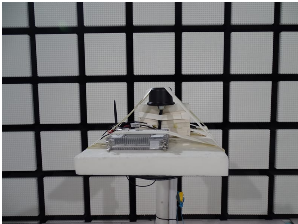
Photo 7: RSE tests with Puck antenna
