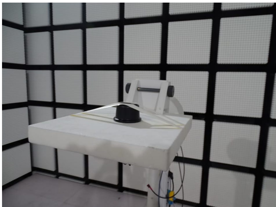
Photo 24: Gain tests with Puck antenna
