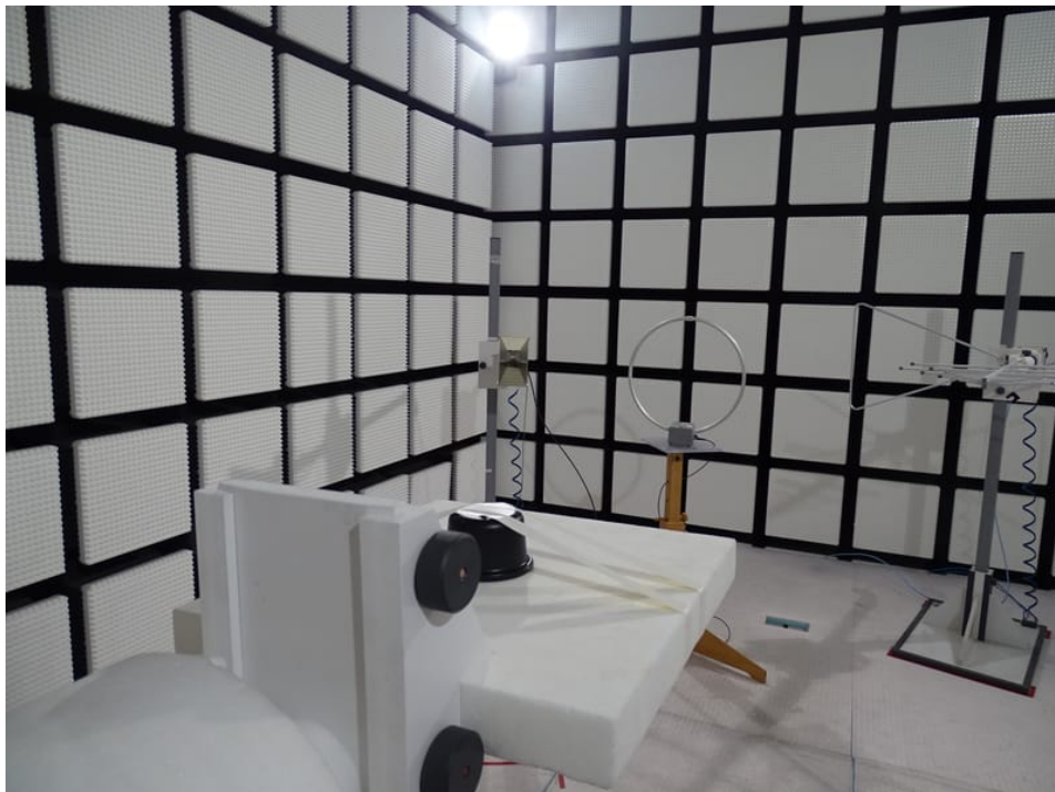
Photo 20: Gain tests with Puck antenna
