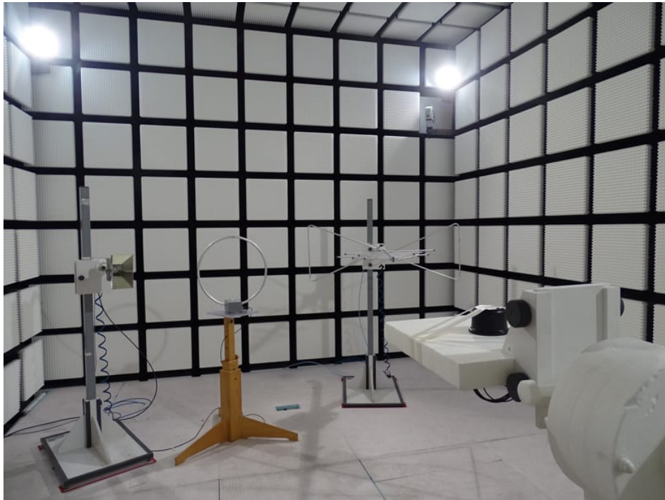
Photo 19: Gain tests with Puck antenna
