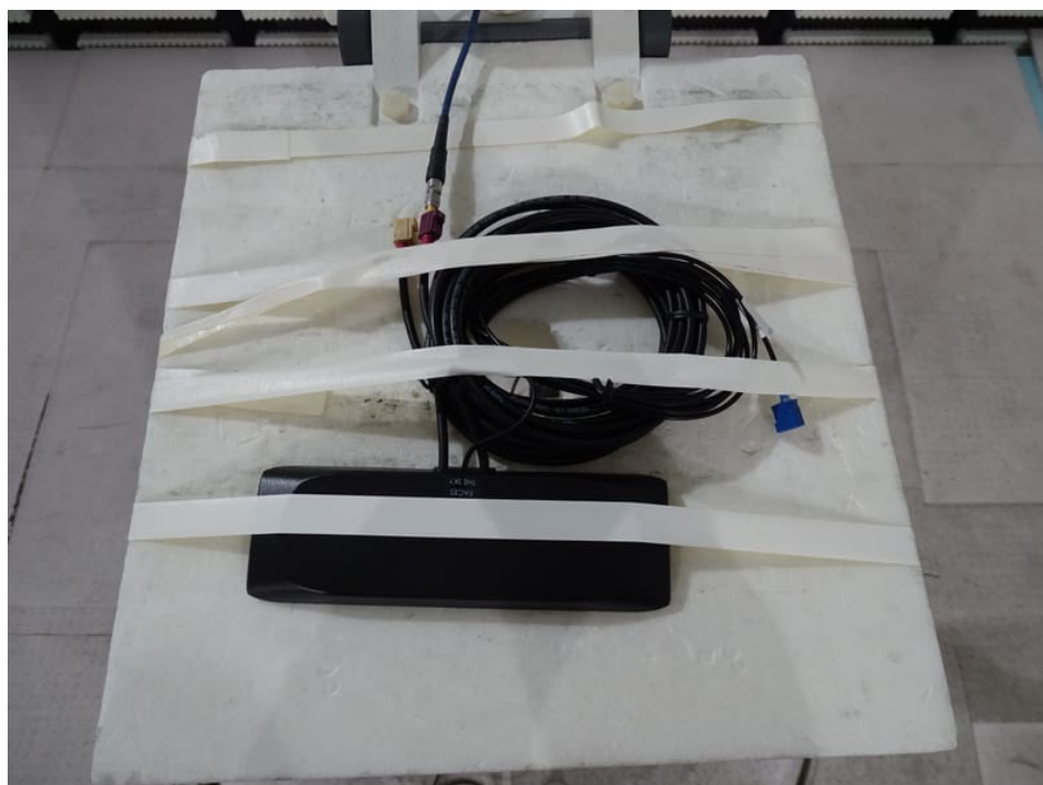
Photo 44: Gain tests with candybar antenna
