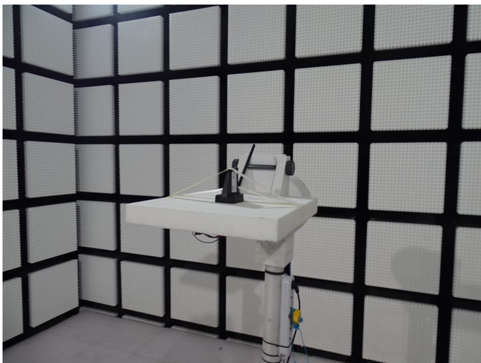
Photo 16: Gain tests with Supercombo antenna
