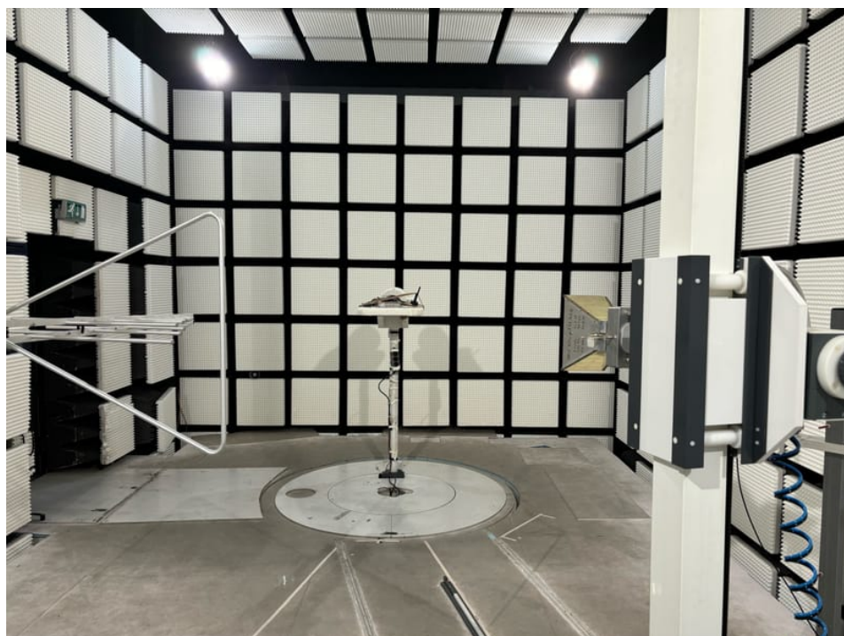
Photo 26: RSE tests with Supercombo antenna
