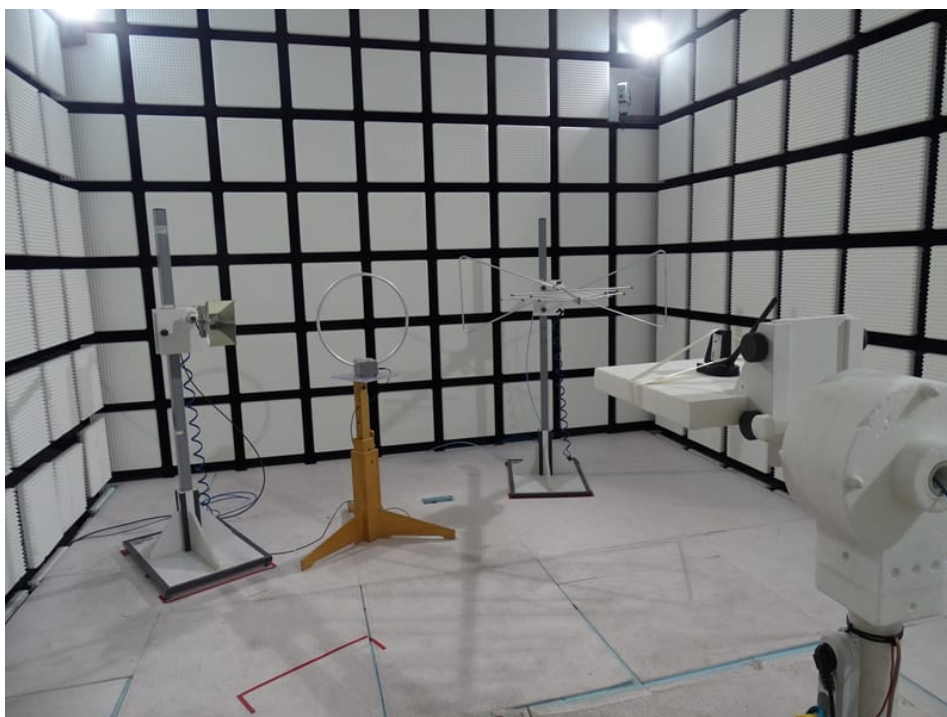
Photo 10: Gain tests with Supercombo antenna
