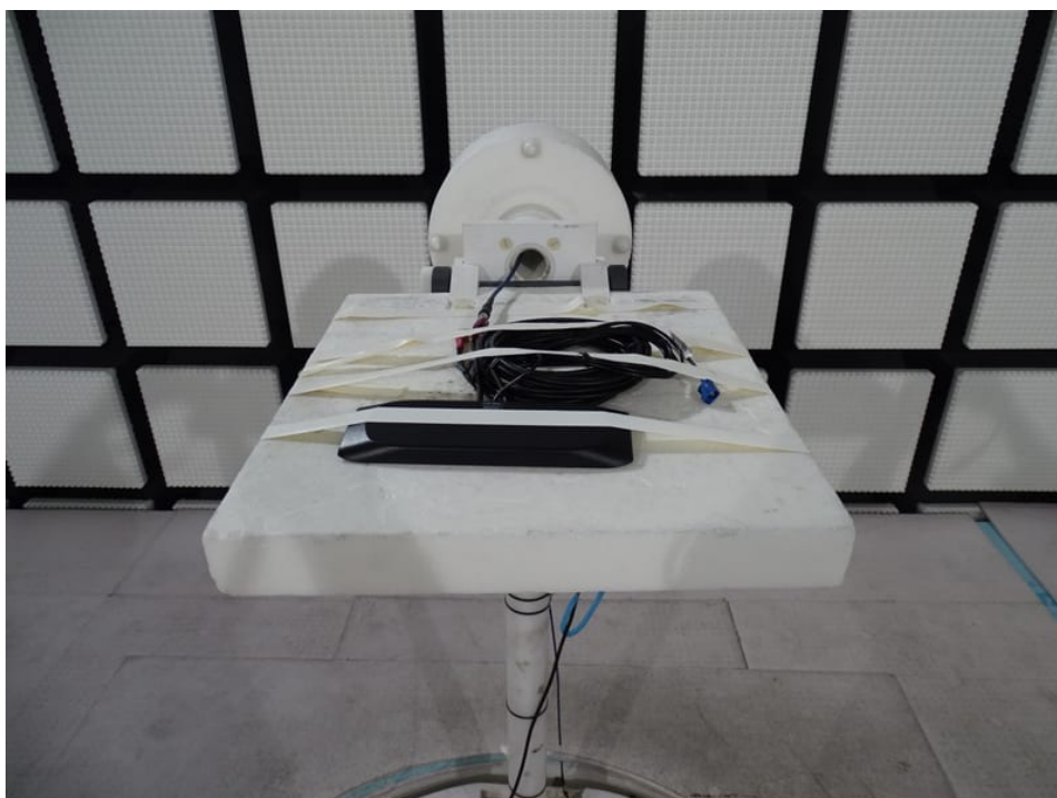
Photo 42: Gain tests with candybar antenna
