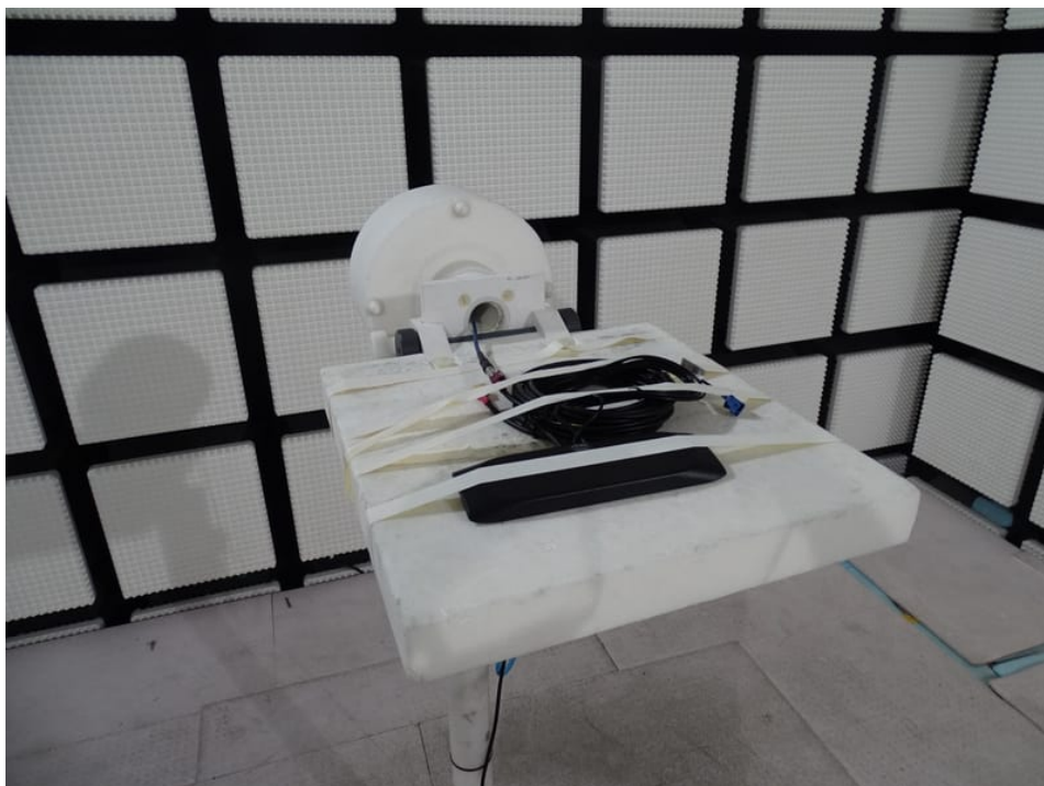
Photo 41: Gain tests with candybar antenna
