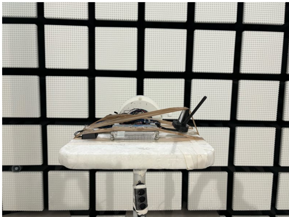
Photo 27: RSE tests with Supercombo antenna
