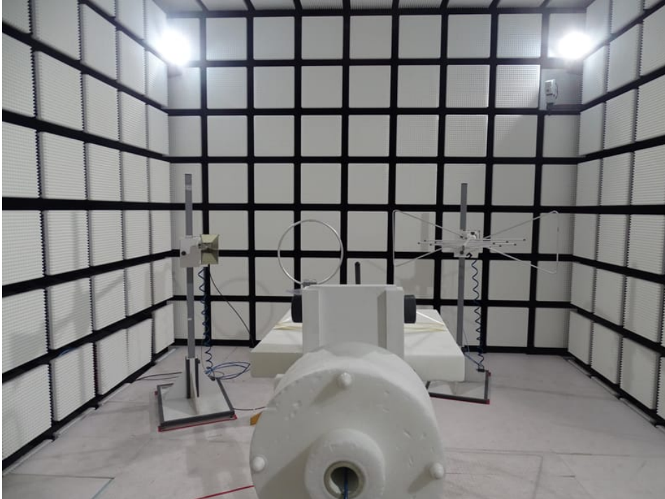
Photo 11: Gain tests with Supercombo antenna
