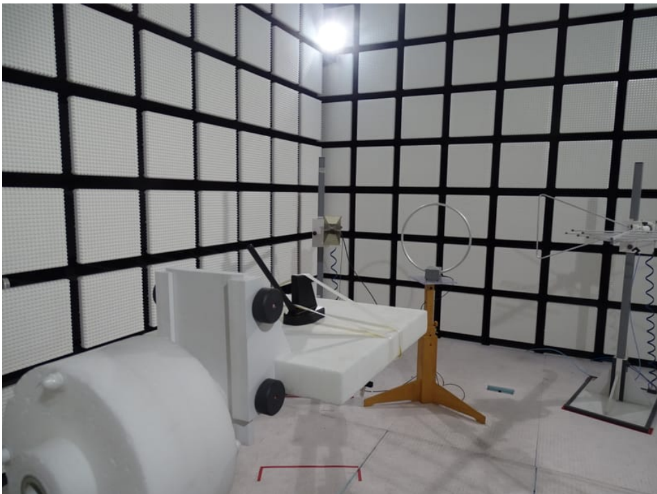
Photo 12: Gain tests with Supercombo antenna
