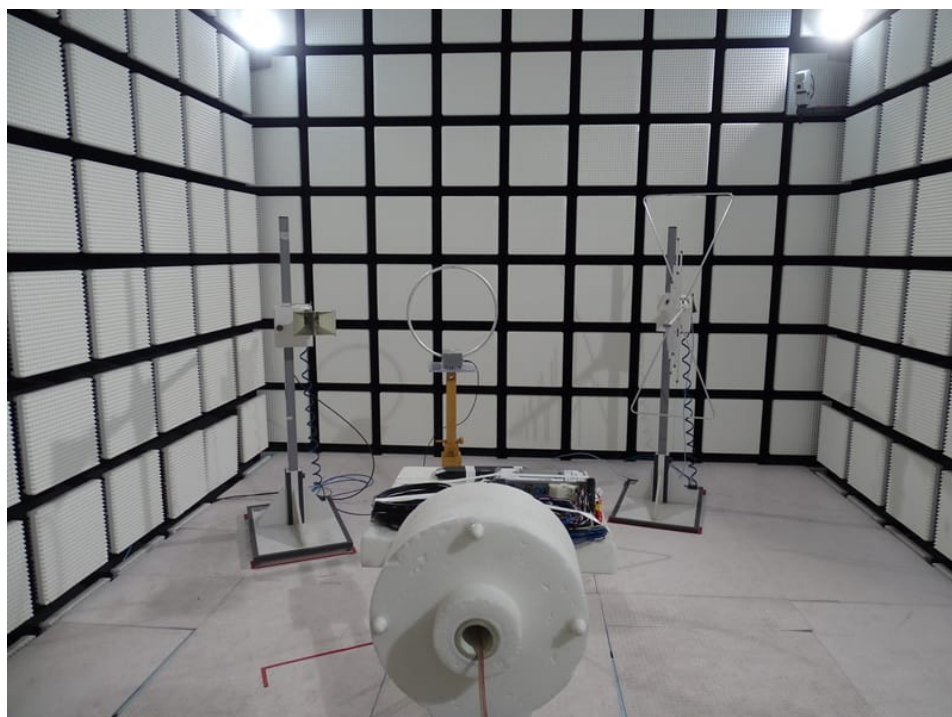
Photo 33: RSE tests with candybar antenna
