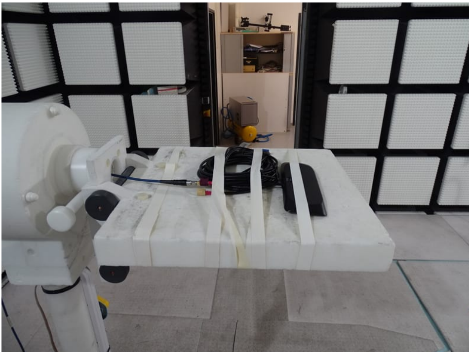
Photo 40: Gain tests with candybar antenna
